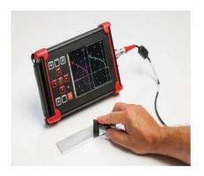
The most widely used technique is the eddy current. Eddy currents are composed of free electrons under the influence of an induced electromagnetic field which are made to "drift" through metal.
