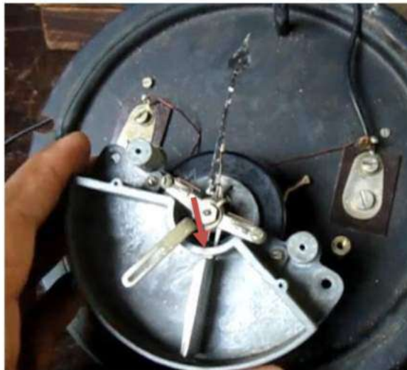
Aluminium vane enclosed in air chamber, attaches with the pointer
