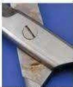
Example of Fretting Corrosion
