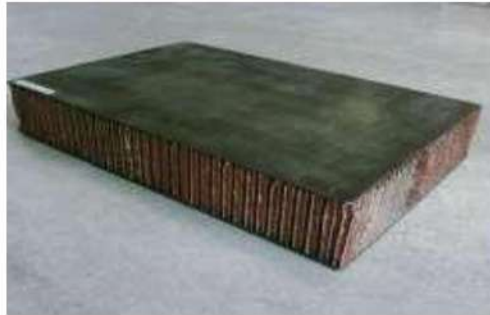
Fig. 3.55 Delamination at Honeycomb Core Edge band
