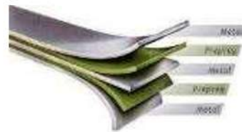
Fig. 3.62 Fiber/Metal Laminate (FML) Other Non-metallic Materials
