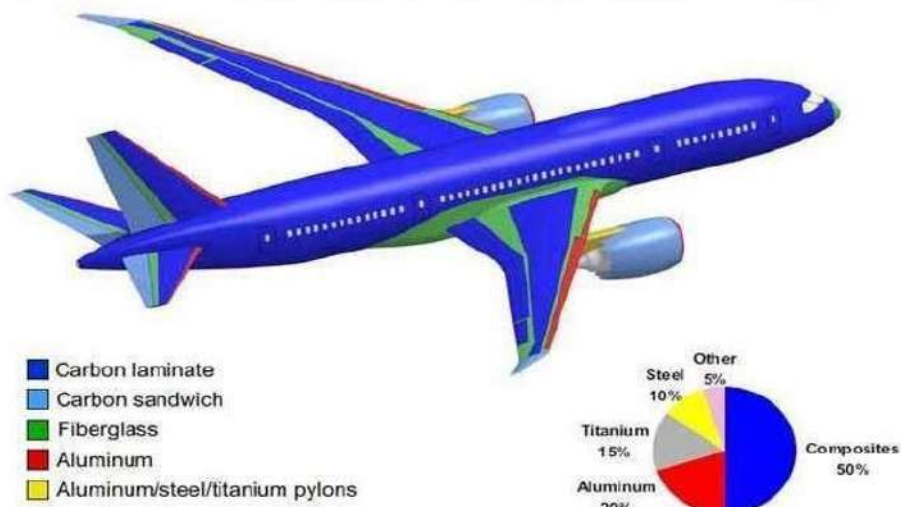
Fig. 6.3 Use of composite in Boeing -787
