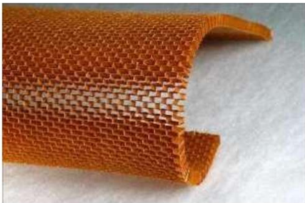
Fig. 3.32 Over expanded core
