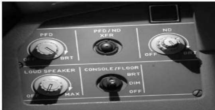
Figure 15.3: A320 PFD and ND Brightness and Transfer Controls
