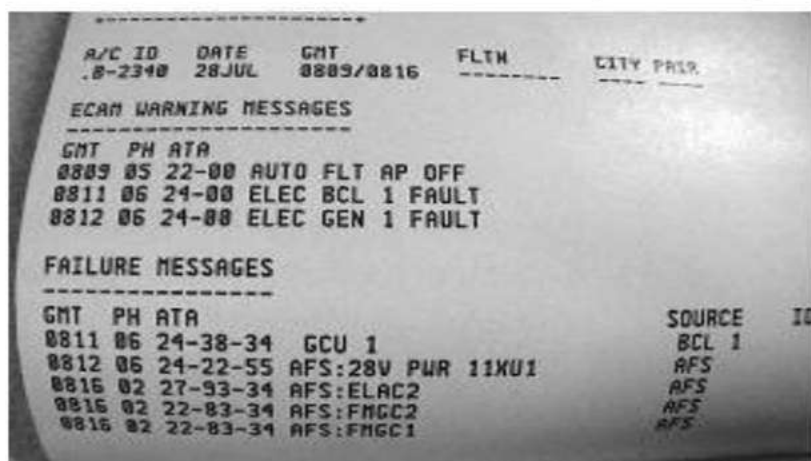
Figure 15.19: ECAM cockpit print out showing warning and failure messages
