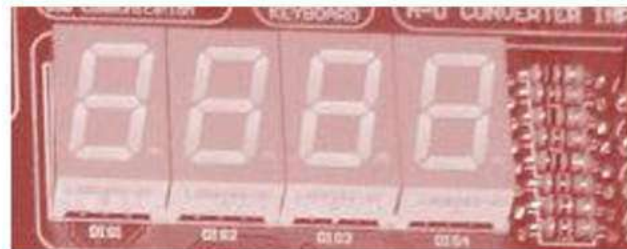
Figure 11.9: Typical example of a four-digit seven segment display
