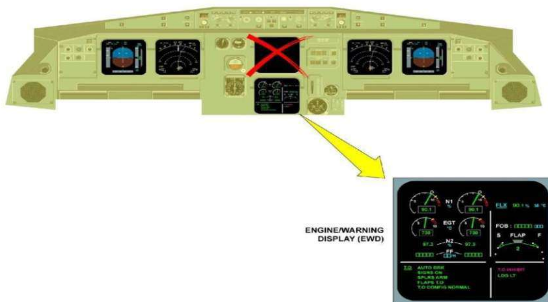
Figure 15.17: Failure of the Engine / Warning Display Unit
