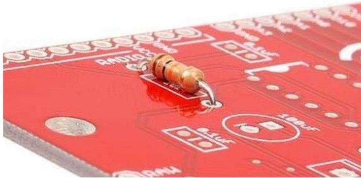
Fig 10.13: A PTH resistor inserted into the FabFM PCB, ready to be soldered. The legs of the resistor go through the holes. The plated holes can have traces connected to them on the front of the PCB and the rear of the PCB.
