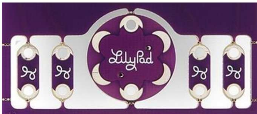
Fig 10.10 : Mouse bites on the LilyPad ProtoSnap allow the PCB to be snapped apart easily
