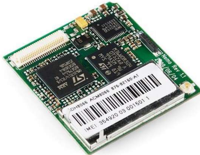
Fig 8.1 :Integrated circuits are the little black “chips”, found all over embedded electronics.
