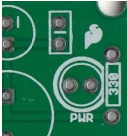
Fig 10.15 : Silkscreen identifying this LED as the power LED
