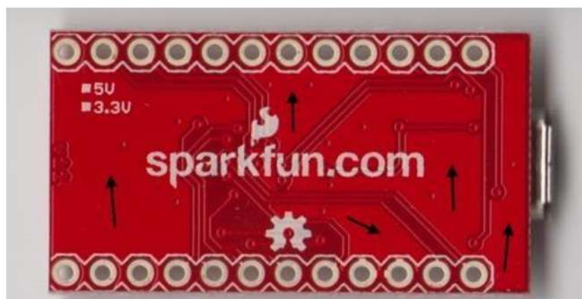
Fig 10.12: Various portions of the PCB that have no traces but has a ground pour instead.
