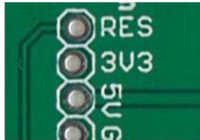
Fig 10.20: A small trace connecting the Reset pad to elsewhere on the board. A larger, thicker trace connects to the 5V power pin.
