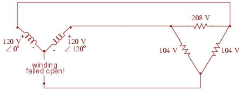
Fig. 13.59 Open “Y” source winding halves the voltage on two loads of a \Delta connected load.
