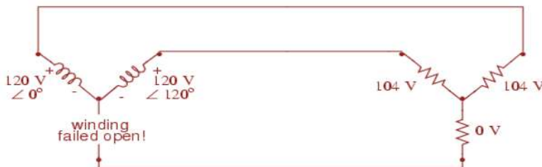
Fig. 13.60 Open source winding of a “Y-Y” system halves the voltage on two loads, and loses one load entirely.
