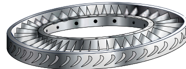
B. Turbine nozzle vane assembly with welded vanes.
