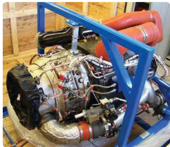
Figure 18-3. Honeywell GTCP 331-350 note the pneumatic output duct on the bottom of the engine the top duct is for the oil cooler unit.
