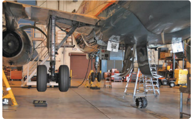
Figure 1-5. Airbus A-320 being jacked.
