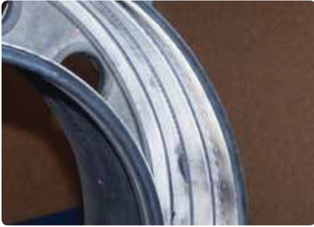
Figure 5-4. Annular combustion chamber liner.
