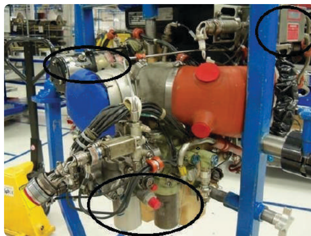
Figure 18-7. Honeywell GTCP 331-350 note the starter motor at upper left, the ignition exciter box at upper right and the fuel and oil filter units attached to the bottom of the gear box.
