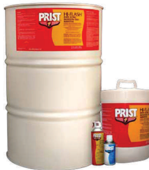
Figure 9-3. Fuel anti-icing products, such as Prist®, act as antifreeze for any free water in aircraft fuel. They dissolve in water and lower its freezing point to prevent ice crystals from disrupting fuel flow.
