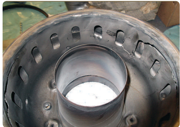
Figure 18-10. A typical APU hot section partially disassembled.
