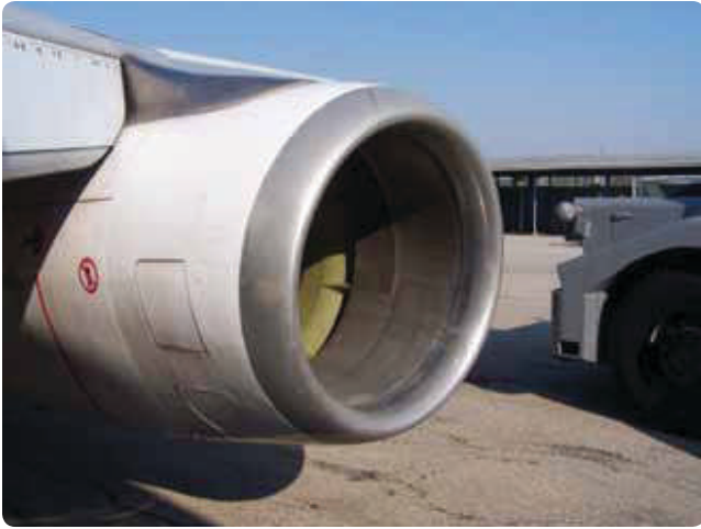
Figure 3-12. A typical turbofan intake section.
