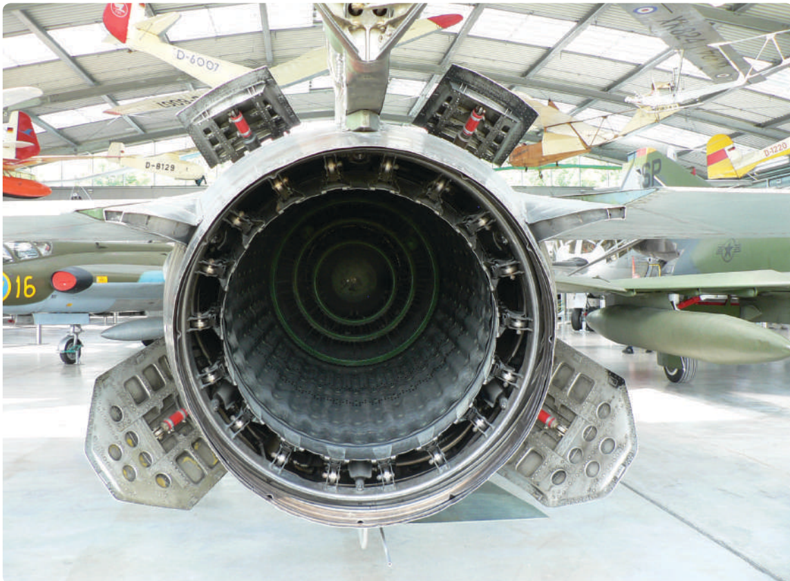
Figure 15-1. A variable exhaust nozzle used to increase or decrease exhaust flow during after burn.
