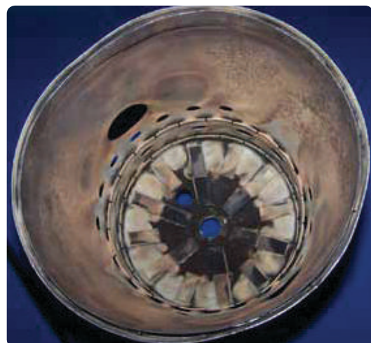
Figure 5-2. Inside view of a combustion chamber liner.
