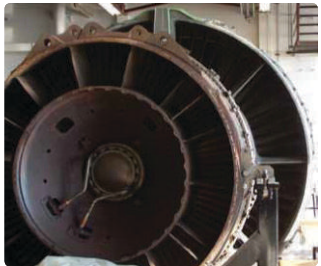
Figure 3-15. Air from the fan exhaust can be discharged overboard through short ducts directly behind the fan.
