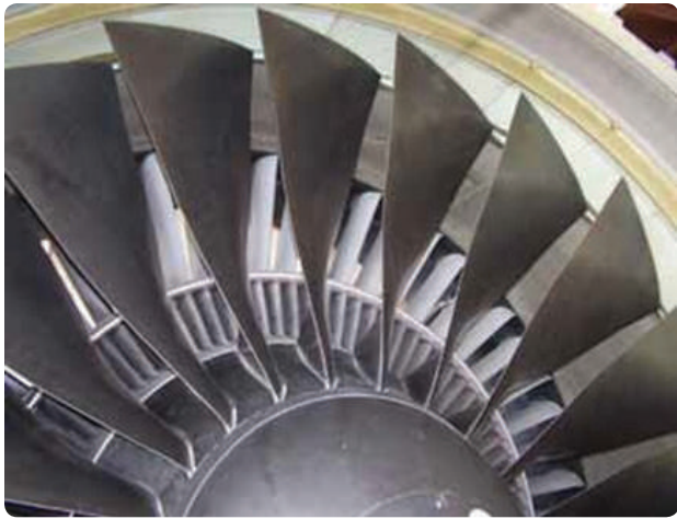
Figure 7-5. Air from these fan blades must be straightened.
