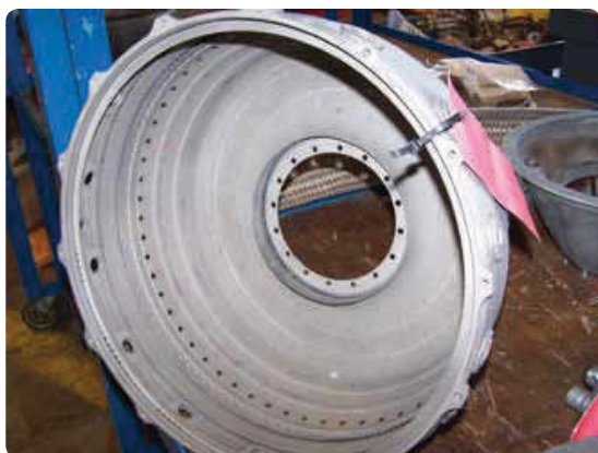
Figure 21-12. Combustion case inspection.
