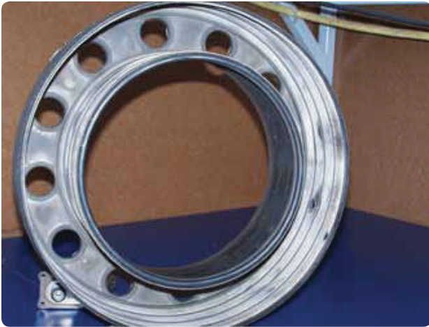
Figure 5-7. Annular combustion with chamber ceramic coating.
