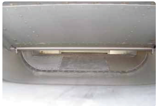
Figure 3-11. Deflector doors used to deflect ice or dirt away from the intake.
