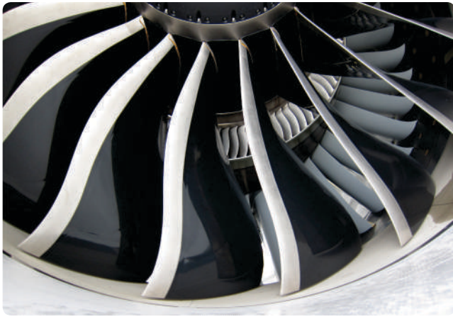
Figure 3-2. Inlet fan blades and guide vanes (inner circle) on a GEEnx engine.
