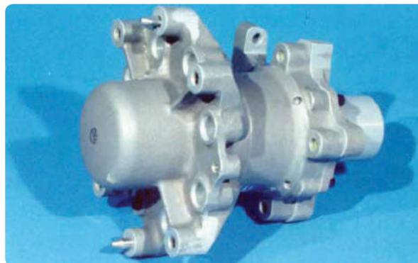
Figure 11-10. Fuel distribution valve.
