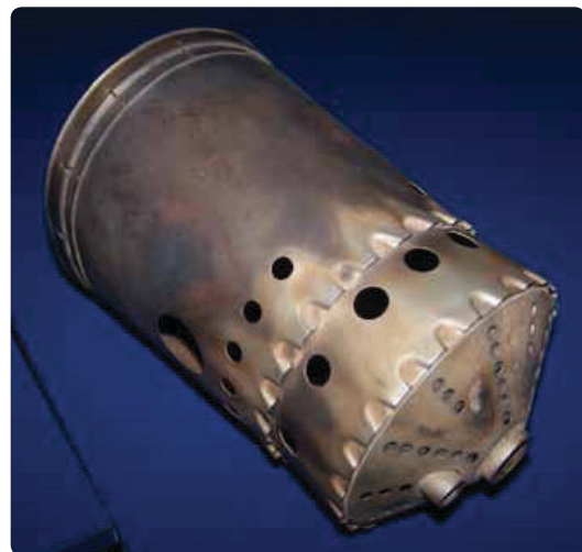
Figure 5-1. Can-type combustion chamber.
