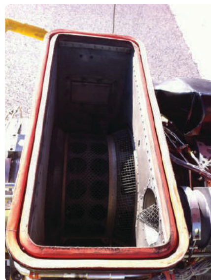
Figure 18-1. APU intake note FOD/ice screen around impeller.
