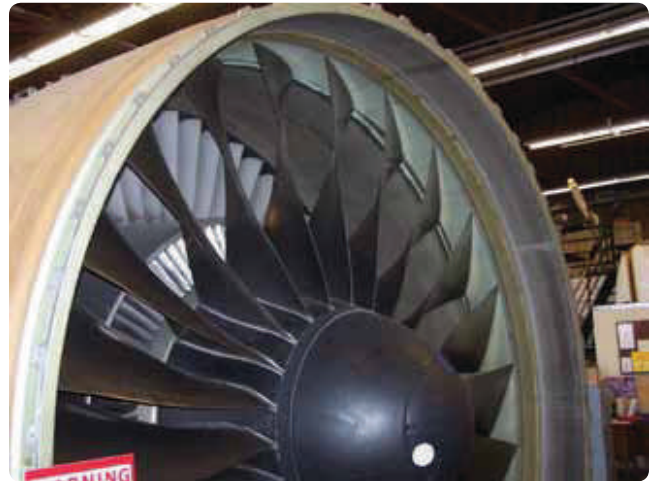
Figure 3-14. The air that passes through the inner part of the fan blades becomes the primary airstream.
