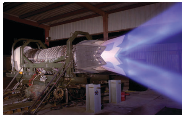
Figure 7-10. A pilot can direct thrust via the vectoring nozzle 20° up or down to increase flight maneuverability.
