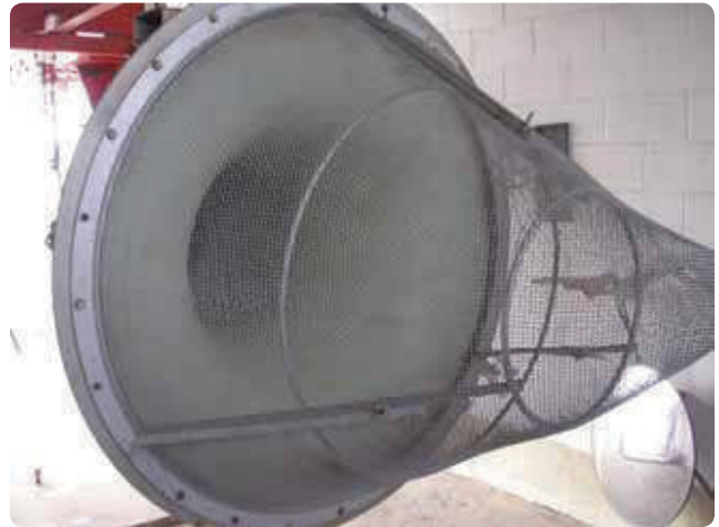
Figure 3-8. A bellmouth inlet used during system tests.
