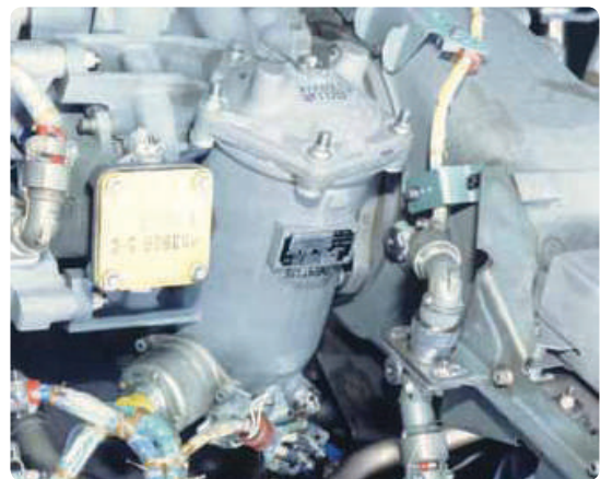
Figure 11-12. High pressure fuel pump of a M-601 turboprop engine manufactured by Jihostroj Technology.
