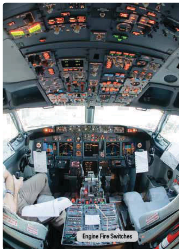
Figure 20-12. Engine fire switches.
