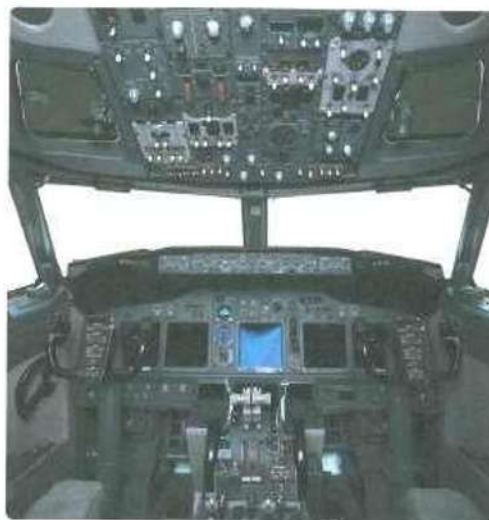
Figure 20-2. An instrument panel with fewer, integrated instruments.
