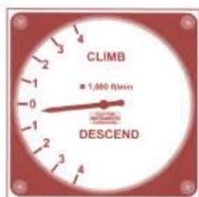
Figure 6.3. A V.S.I. With a Linear Scale Showing a Descent of 250 ft/min.
