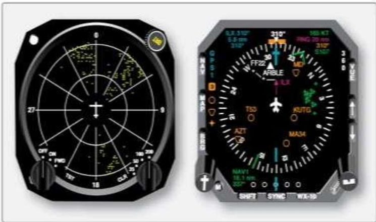
Figure 11-145. A dedicated stormscope lightning detector display (left), and an electronic navigational display with lightning strikes overlaid in the form of green "plus" signs (right).
