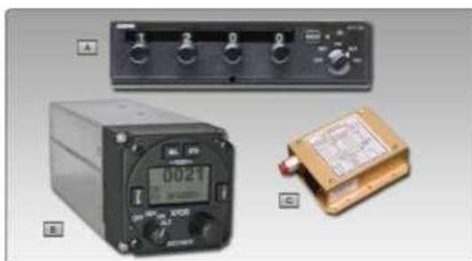
Figure 11-125. A traditional transponder control head (A), a lightweight digital transponder (B), and a remote altitude encoder (C) that connects to a transponder to provide ATC with an aircraft's altitude displayed on a PPI radar screen next to the target that represents the aircraft.
