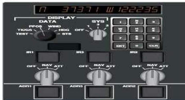
Figure 11-155. An interface panel for three air data and inertial reference systems on an Airbus. The keyboard is used to initialize the system. Latitude and longitude position is displayed at the top.
