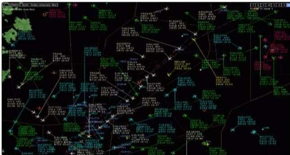
Figure 11-128. Air traffic control radar technology and an onboard radar beacon transponder work together to convey and display air traffic information on a PPI radar screen. A modern approach ATC PPI is shown. Targets representing aircraft are shown as little aircraft on the screen. The nose of the aircraft indicates the direction of travel. Most targets shown above are airliners. The data block for each target includes the following information either transmitted by the transponder or matched and loaded from flight plans by a flight data processor computer: call sign, altitude/speed, origin/destination, and aircraft type/ETA (ZULU time). A "C" after the altitude indicates the information came from a Mode C equipped transponder. The absence of a C indicates Mode S is in use. An arrow up indicates the aircraft is climbing. An arrow down indicates a descent. White targets are arrivals, light blue targets are departures, all other colors are for arrivals and departures to different airports in the area.
