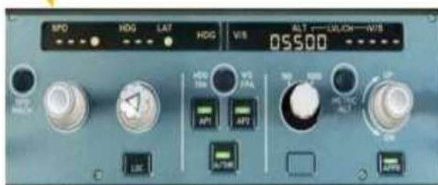
The FMS is well suited for long term planning and inputs. In case of sudden changes or technical malfunction it can always be overruled by taking over command through the Flight Control Unit (FCU) or by disengaging the autopilot. Using the FCU, inputs to speed, heading, altitude and vertical speed can be done with immediate effect.
