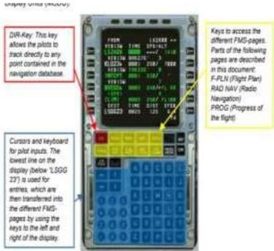
Fig. 1: Overview of the Multipurpose Control and Display Unit (MCDU) used in the Airbus A320.
