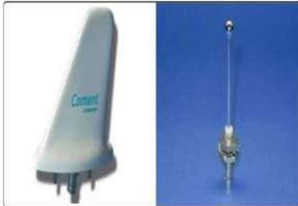
Figure 11-127. Aircraft radar beacon transponder antennas transmit and receive 1090 and 1095 MHz radio waves.
