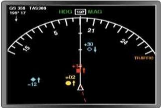
Figure 11-133. TCAS information displayed on a multifunction display. An open diamond indicates a target; a solid diamond represents a target that is within 6 nautical miles of 1,200 feet vertically. A yellow circle represents a target that generates a TA (25-48 seconds before contact). A red square indicates a target that generates an RA in TCAS II (contact within 55 seconds). A (+) indicates the target aircraft is above and a (-) indicates it is below. The arrows show if the target is climbing or descending.
