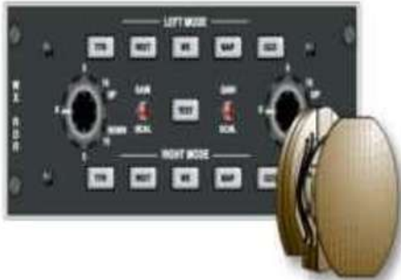
Figure 11-143. A typical weather radar control panel for a high performance aircraft with a new radome antenna the pilot is to install. The panel is to be installed in the cockpit. The radome is to be installed in the fuselage. The radome is to be painted with a special paint. The radome is to be grounded. The radome is to be protected from lightning strikes.
