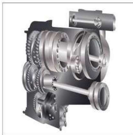
Figure 18-37A. Constant speed drive.
