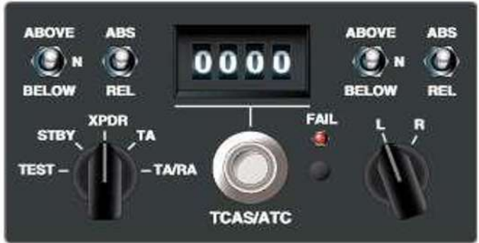
Figure 11-134. This control panel from a Boeing 767 controls the transponder for ATC use and TCAS.
