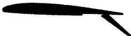
FIGURE 4-30 Operation of the Fowler flap.
