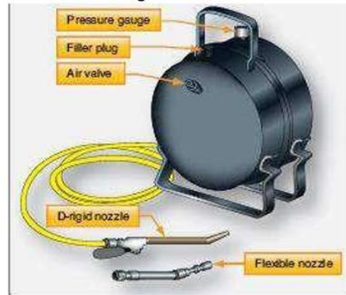
Figure-88 A typical brake bleeder pot or tank contains brake fluid under pressure. It pushes the fluid through system to displace any air that may be present.
