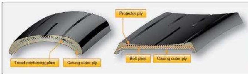
Figure-101 Tread wear on a bias ply tire (left) and a radial tire (right) show wear beyond limits of serviceability but still eligible to be retreaded
