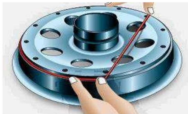
Figure-114 The wheel half O-ring for a tubeless tire wheel assembly must be in good condition and lubricated to seal for the entire life of the tire. The mating surfaces of the wheel halves must also be in good condition.
