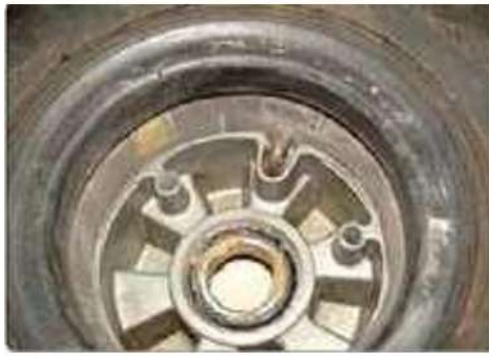
Figure-115 Mounting a tube type tire with the tube valve stem positioned to pass through the outboard wheelhalf.
