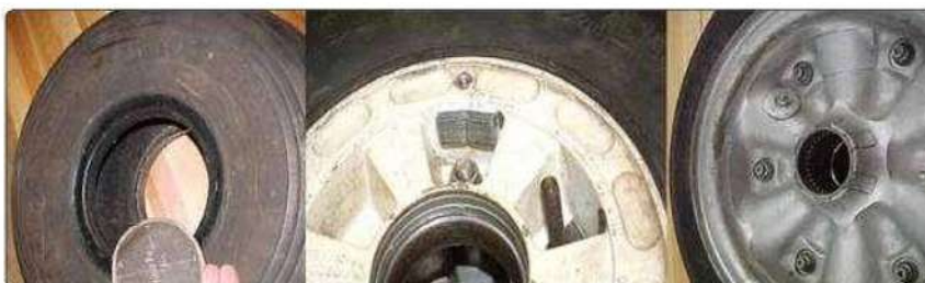
Figure 118 A tire balancing patch (left), adhesive wheel weights (center), and a bolted wheel weight
