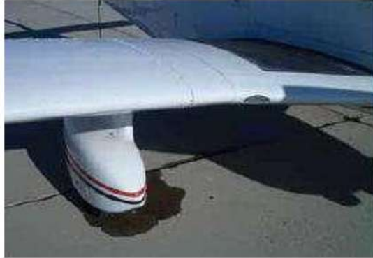
Figure-91 The cause of all aircraft brake leaks must be investigated, repaired, and tested before releasing the aircraft for flight.
