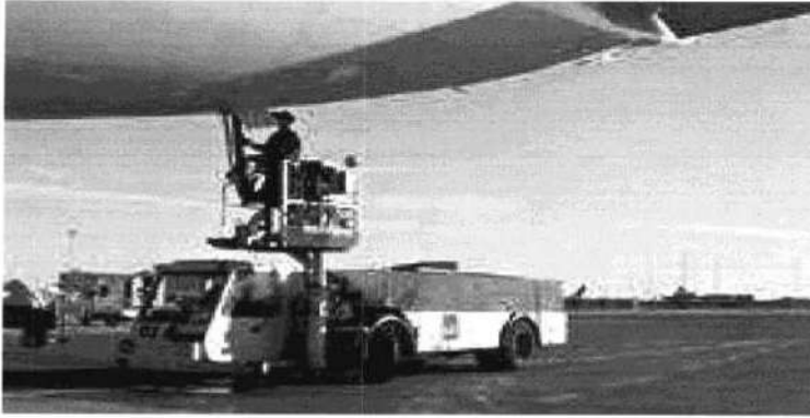
Fig.17.19 Toilet draining and flushing
