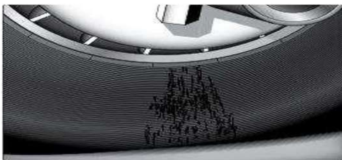
Figure-108 Cracking and checking in the sidewall of a tire is acceptable for service as long as it does not extend to or
