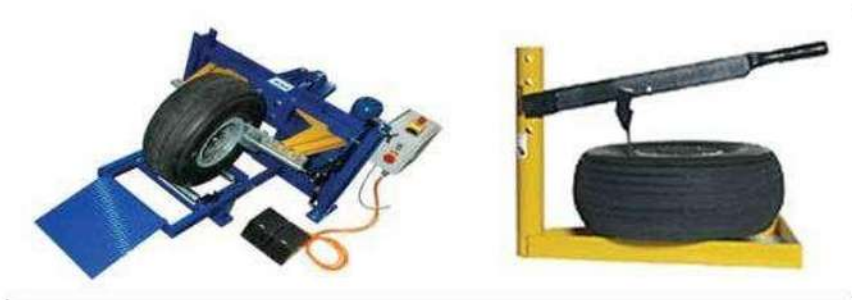
Figure-111 An electrohydraulic tire bead breaker (left) used on large tires and a manual tire bead breaker (right) used on small tires.
