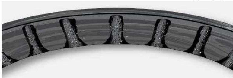
Figure 48- Bruising is caused by fine particle contamination possibly from a bad seal or improper maintenance of bearing cleanliness. It leaves a less than smooth surface on the bearing cup. The bearing cup does not require removal for inspection; however, it must be firmly seated in the wheel half boss. There should be no evidence that a cup is loose or able to spin. [Figure-49] The cup is usually removed by heating the wheel in a controlled oven and pressing it out or tapping it out with a
