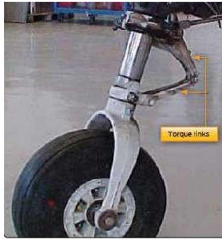
Figure 10- Torque links align the landing gear and retain the piston in the upper cylinder when the strut is extended
