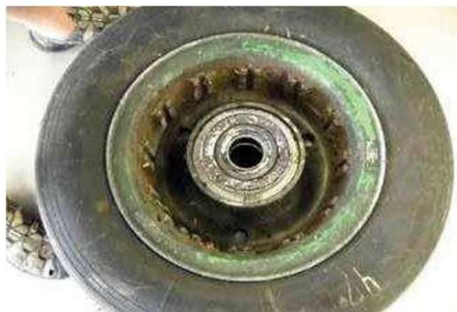
Figure-38 Keys on the inner wheel half of an aircraft wheel used to engage and rotate the rotors of a disc brake.
