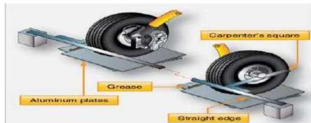
Figure-20 Finding tow-in and two-out on a light aircraft with spring steel struts.
