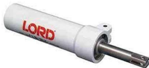
Figure-36 A non-hydraulic shimmy damper uses a rubber piston with lubricant that dampens via motion against the inner diameter of the unit housing.
