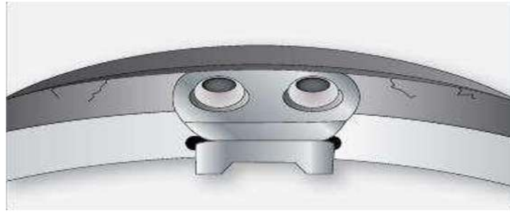
Figure-51 Inspection for cracks in the wheel disc drive key area is performed with dye penetrant on many wheels.
