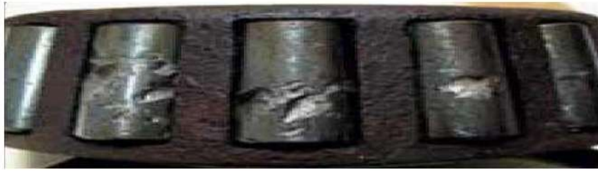
Figure 42 Spalling is a chipped away portion of the hardened surface of a bearing roller or race.
