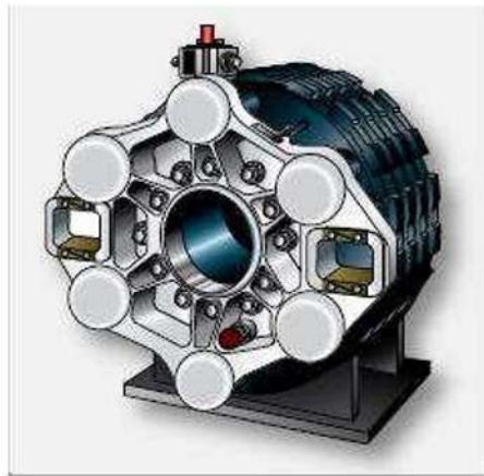
Figure 13-63 A carbon brake for a Boeing 737.
