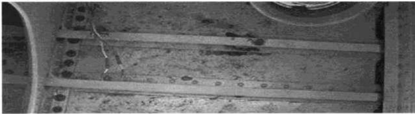
Fig. 10.71 Microbial contamination in a wing tank
