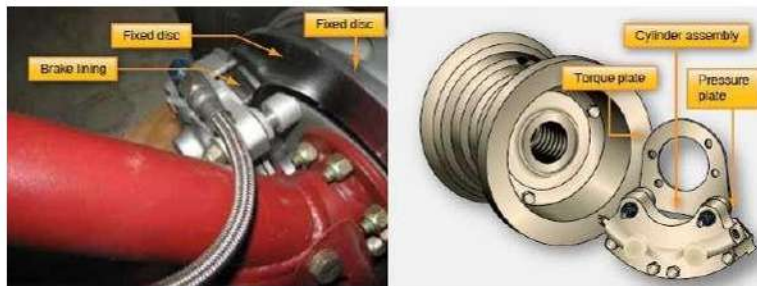
Figure 57-A Cleveland brake on a light aircraft is a fixed-disc brake. It allows the brake caliper to move laterally on anchor bolts to deliver even pressure to each side of the brake disc.
