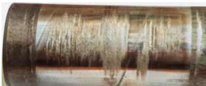
Figure 41 Galling is caused by rubbing of mating surfaces. The metal gets so hot it welds, and the surface metal is destroyed as the motion continues and pulls the metal apart in the direction of motion.
