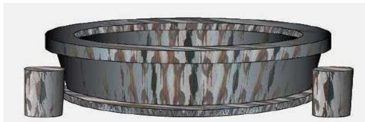
Figure 47 Etching and corrosion is caused when water, and the damage caused by water, penetrates the surface treatment of the bearing element. It appears as a reddish/brown discoloration.
