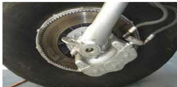
Figure 54A single disc brake is a floating-disc, fixed caliper brake.
