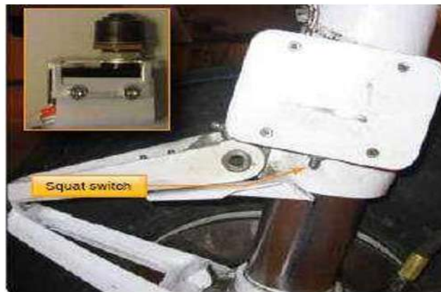
Figure 13-27. Typical landing gear squat switches.
