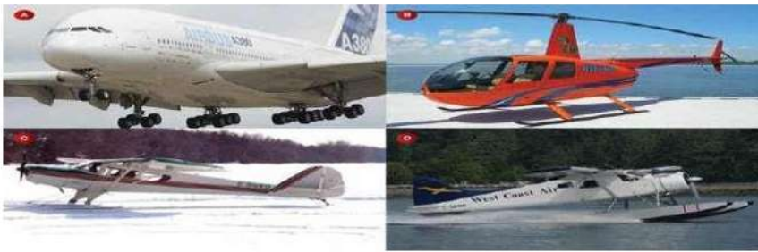
Figure 1- Basic landing gear types include those with wheels (a), skids (b), skis (c), and floats or pontoons (d).
