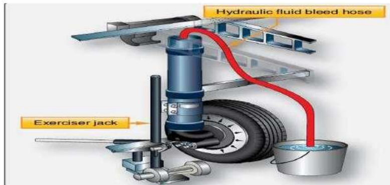
Figure-18 Air trapped in shock strut hydraulic fluid is bled by exercising the strut through its full range of motion while the end of an air-tight bleed hose is submerged in a container of hydraulic fluid.
