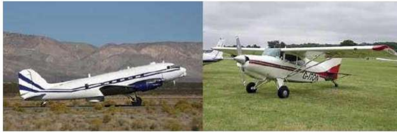
Figure 2- Tail wheel configuration landing gear on a DC-3 (left) and a STOL Maule MX-7-235 Super Rocket
