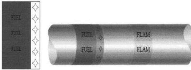
Fig. 10.87 Fuel pipeline identification label
