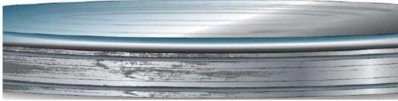
Figure-49 Bearing cups should be tight in the wheel boss and should never rotate. The outside of a bearing cup that was spinning while installed in the wheel is shown.
