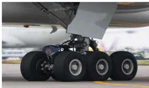
Figure 5- Triple bogie main landing gear assembly on a Boeing 777.
