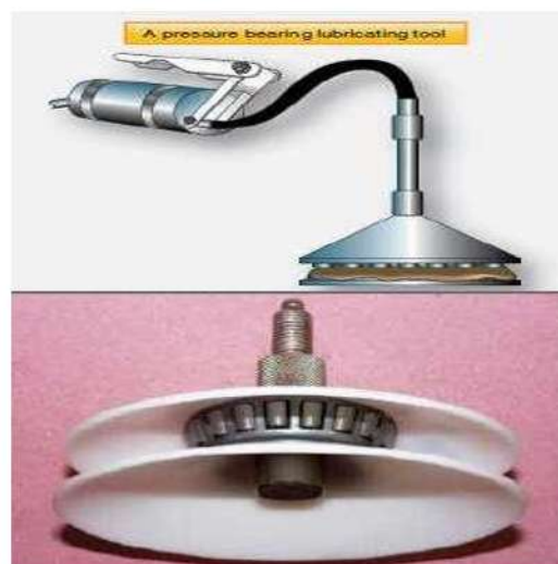
Figure-50 A pressure bearing lubricating tool.
