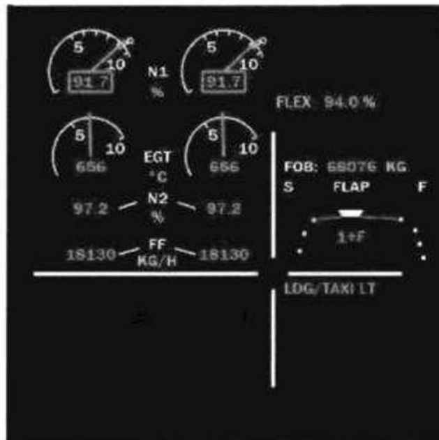
Fig. 9.39 Modern Indication Display Position and Asymmetry Monitoring
