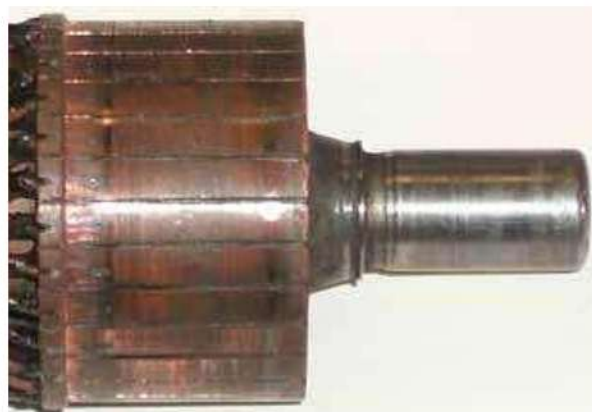
Figure 15: Commutator with Portion Removed to Show Construction
