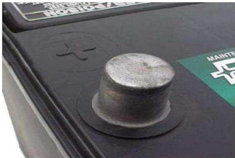
Figure 15 : Battery + ve Terminal
