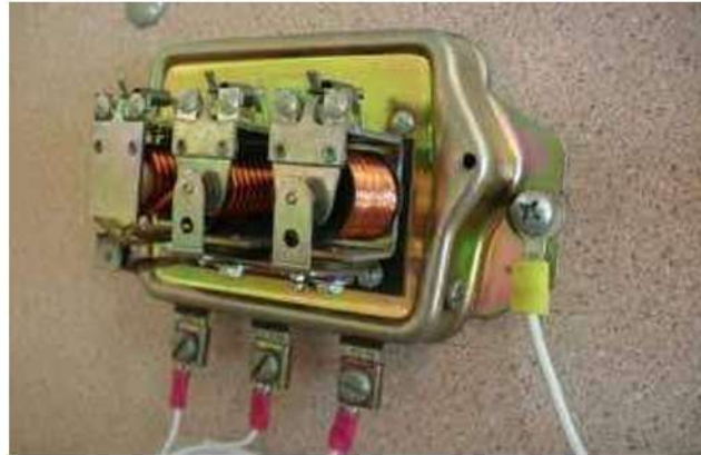
Figure-20, The three relays found on this regulator are used to regulate voltage, limit current, and prevent reversecurrent flow
