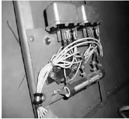
Figure 108 : Relay Installation (GA Aircraft)
