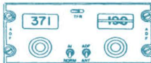
Fig. 2.68 ADF Control Panel
