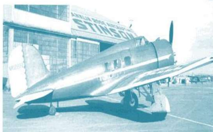
Figure 2.35: Plywood Monocoque Aeroplane (Lockheed Orion)
