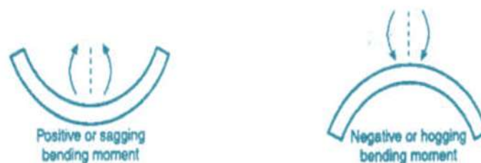
Fig. 2.30: Bending Electrical Bonding
