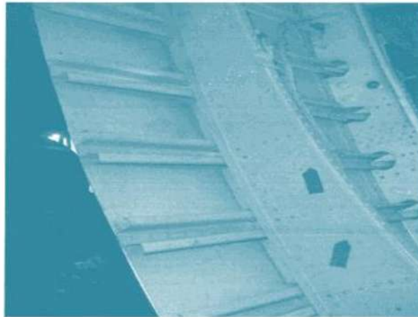
Fig. 3.3: Fuselage stringers, skin and frame
