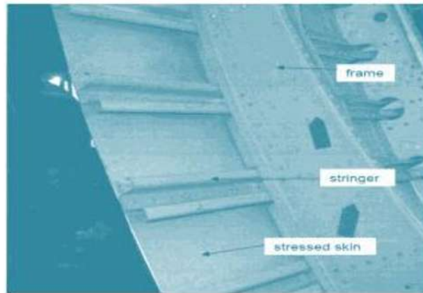
Fig. 2.39: Metal semi-monocoque structure
