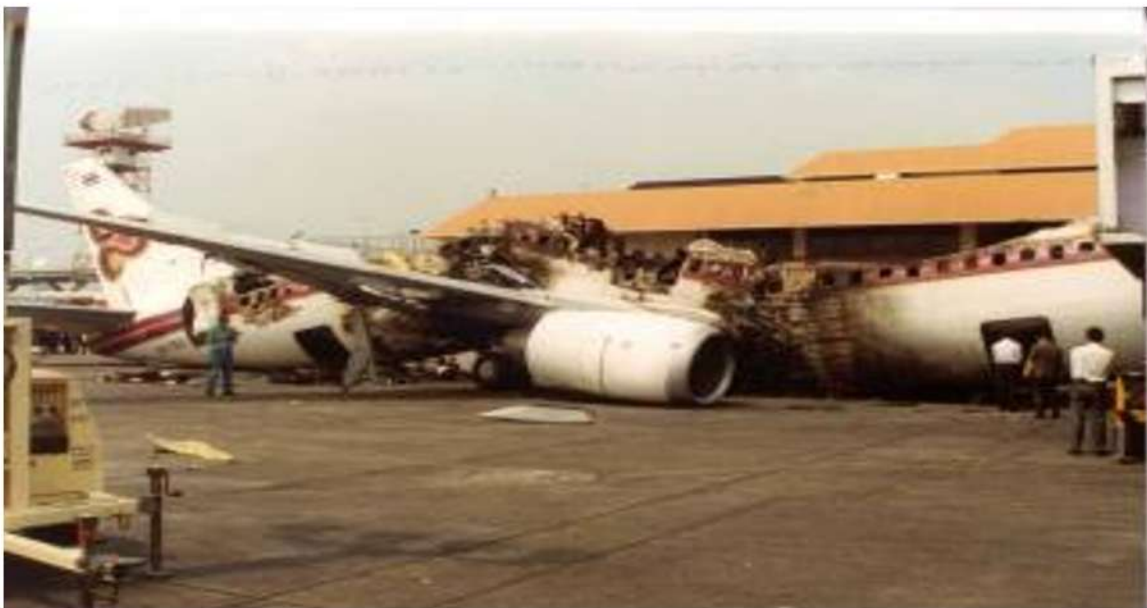
737 Manila (Philippine Airlines) While pushing back from gate, empty centre fuel tank exploded
