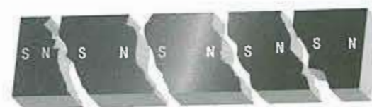
Figure 10-9. Magnetic poles in a broken magnet.
