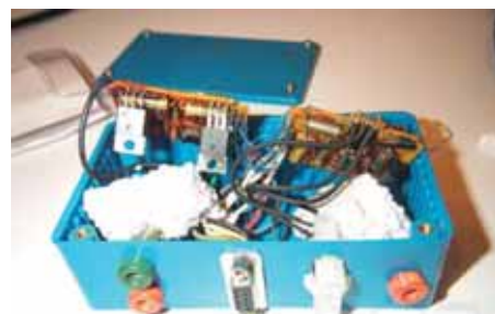
Two comparator integrated circuits.
