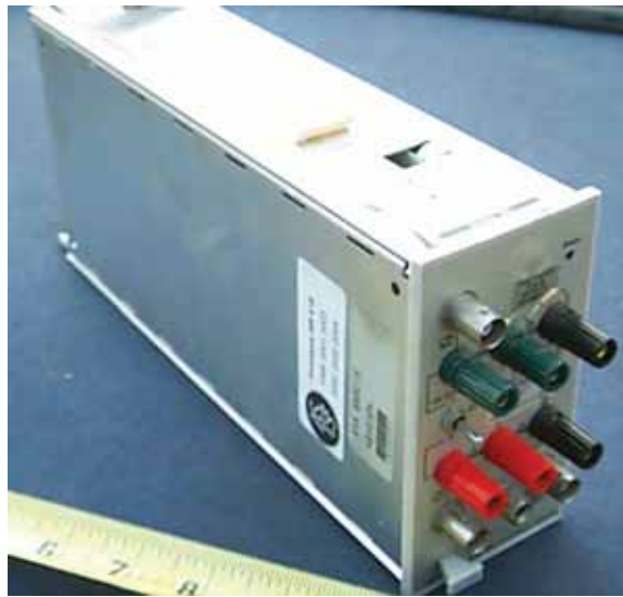
Non-inverting operational amplifier.
