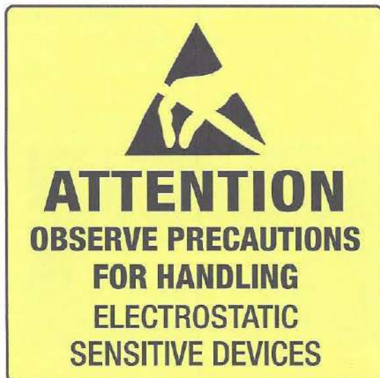
Figure 12-3. Warning sign for an ESD controlled area.
