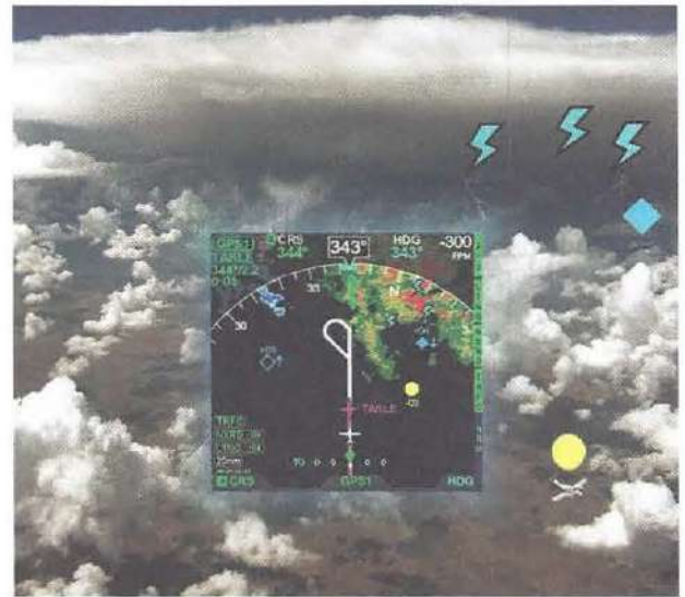
Figure 14-3. Lightning detection overlaid on a MFD weather radar page.
