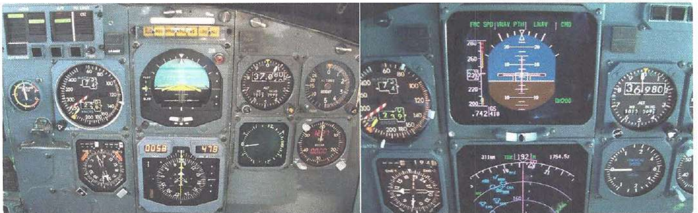
Figure 1-3. Equivalent Electromechanical Flight and Navigation Instruments on the left.
