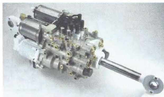
Figure 15-16. Electrostatic Actuator used on the F-35 horizontal tail.
