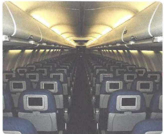
Figure 10-9. Panasonic IFE system installed on a Boeing 737-800.
