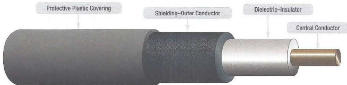
Figure 10-1. Coaxial Cable typically used for data rates of 2Mbps to 50Mbps.
