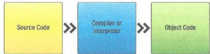
Figure 6-6. High-level source code converted in to object code (machine language).
