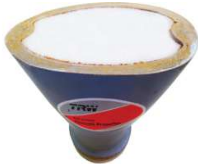
Cross section of composite propeller blade.
