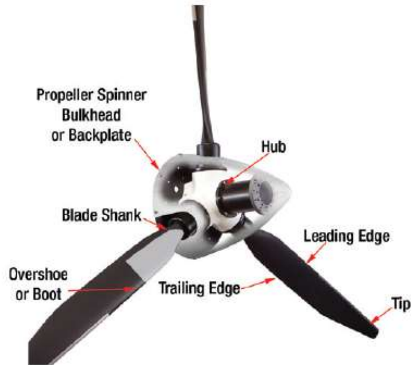
Parts of a Propeller.
