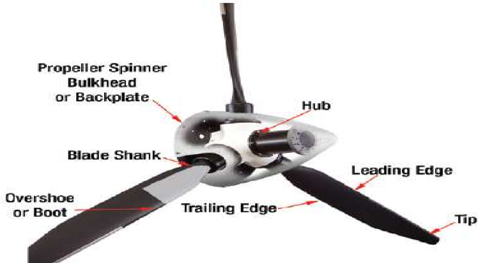
Parts of a Propeller.
