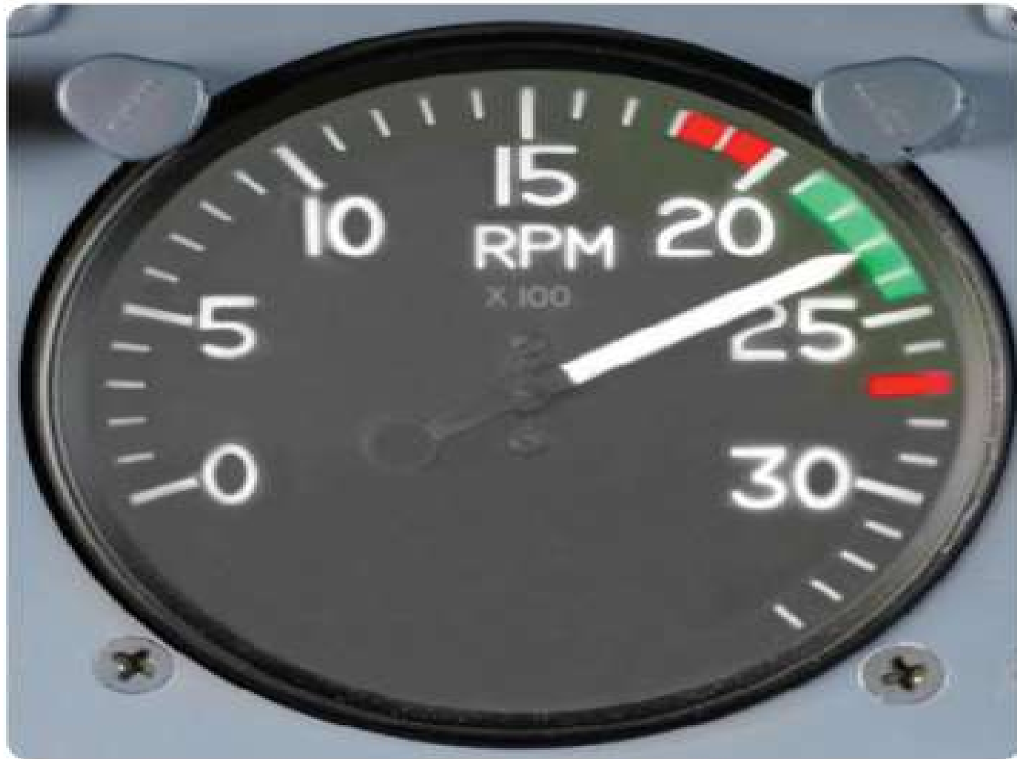
Red arc from 1 800 to 2 000 rpm.
