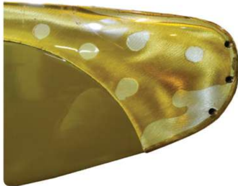
Tip on wooden propeller revealing soldered attachment hardware and drain holes.
