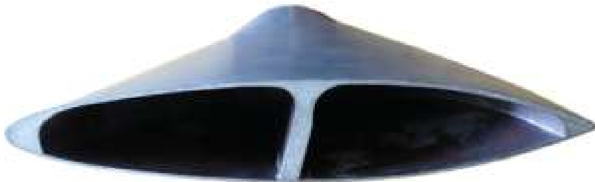
Cross section of steel propeller blade.
