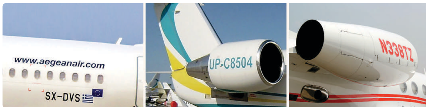
Figure 5-12. Example of national aircraft registration prefixes; SX for Greece, UP for Kazakhstan, N for United States.
