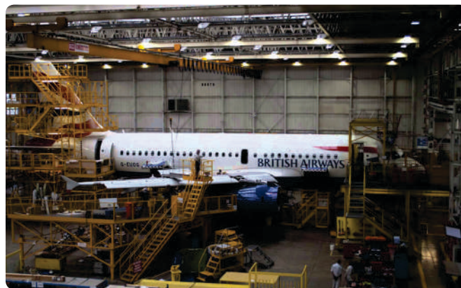
Figure 7-1. "C" Check inspection.
