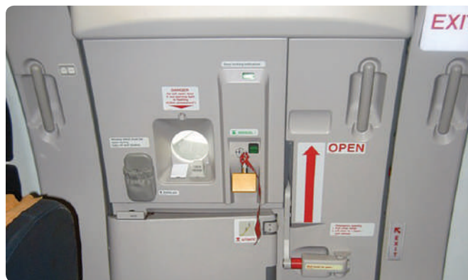
Figure 4-5. Required emergency exit markings.
