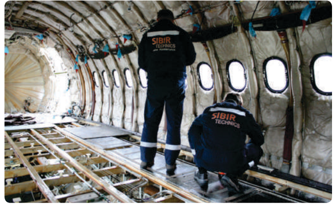
Figure 7-2. "D" Check inspection.
