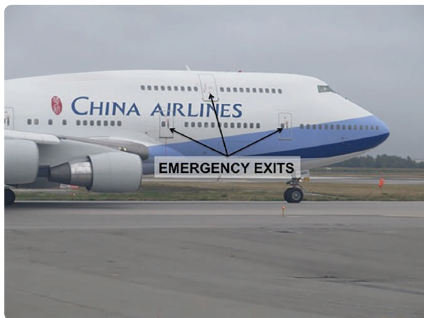
Figure 4-6. Required external emergency exit markings.
