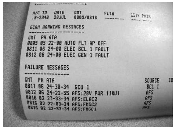
Figure 15.16 ECAM cockpit print out showing warning and failure messages
