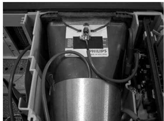
Figure 11.2 Rear view of a CRT display showing external graphite coating and mumetal magnetic shielding
