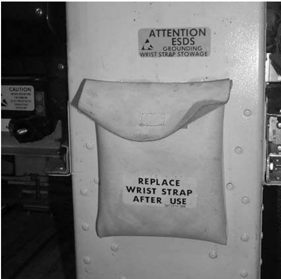
Figure 12.5 Typical on-board storage for a wrist strap
