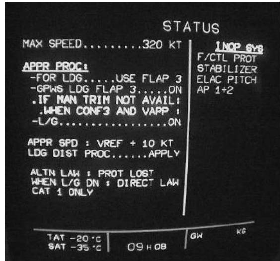
Figure 11.1 An example of information displayed on a flight deck CRT
