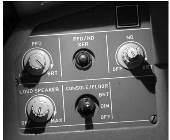
Figure 15.4 A320 PFD and ND brightness and transfer controls
