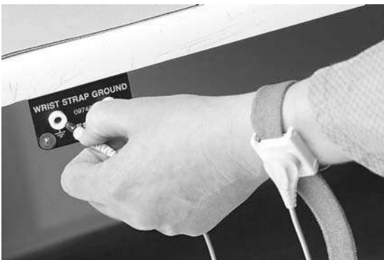
Figure 12.6 Using a wrist strap for a bench operation (note the grounding jack connector)
