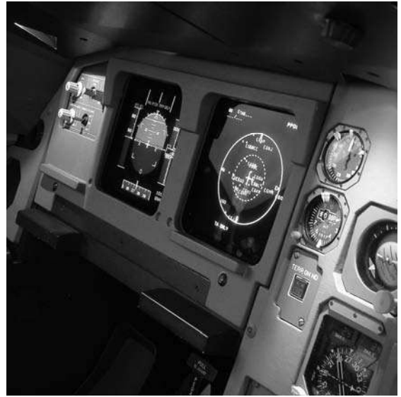
Figure 15.3 'Glass cockpit' (EFIS) displays in an A320
