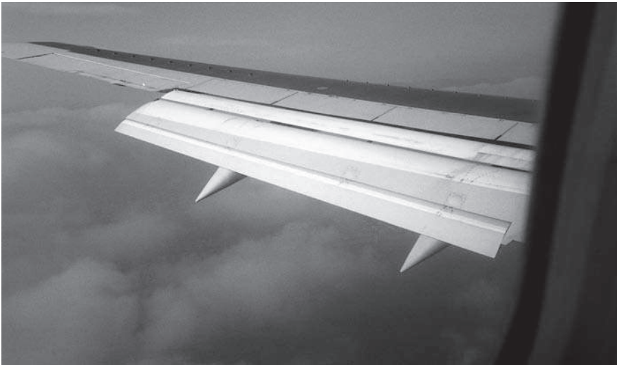
Fig 3H Multi-element slotted flaps Three-element slotted Fowler-type flaps extend rearwards and down as this Boeing 737 prepares to land.
