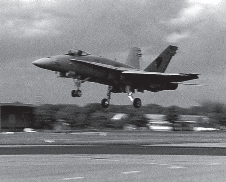
Fig 12E Another supersonic configuration The McDonnell Douglas F-18 Hornet which features a wing with only moderate rearward sweep on the leading edge, and a small forward sweep on the trailing edge. The sharply swept strakes also generate lift, and control the flow over the main wing.
