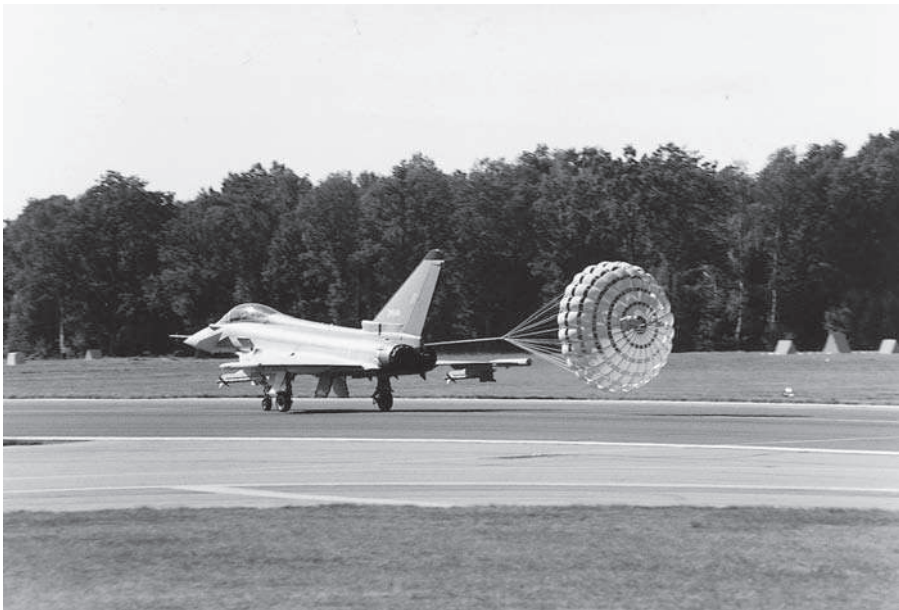
Fig 6K Pulling up after landing Eurofighter Typhoon using an arrester parachute to reduce the landing run.
