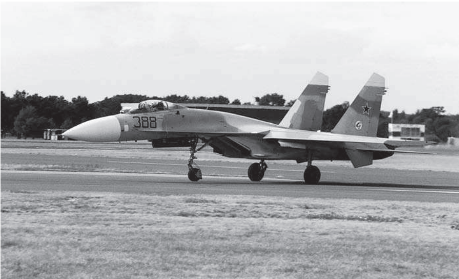
Fig 9G Fin and directional stability A Sukhoi Su-27 blasting down the runway with nosewheel lifting clear of the ground. Note the two large fins with dorsal extension below the tailplane. This aircraft displays exceptional manoeuvrability and control at low speed.
