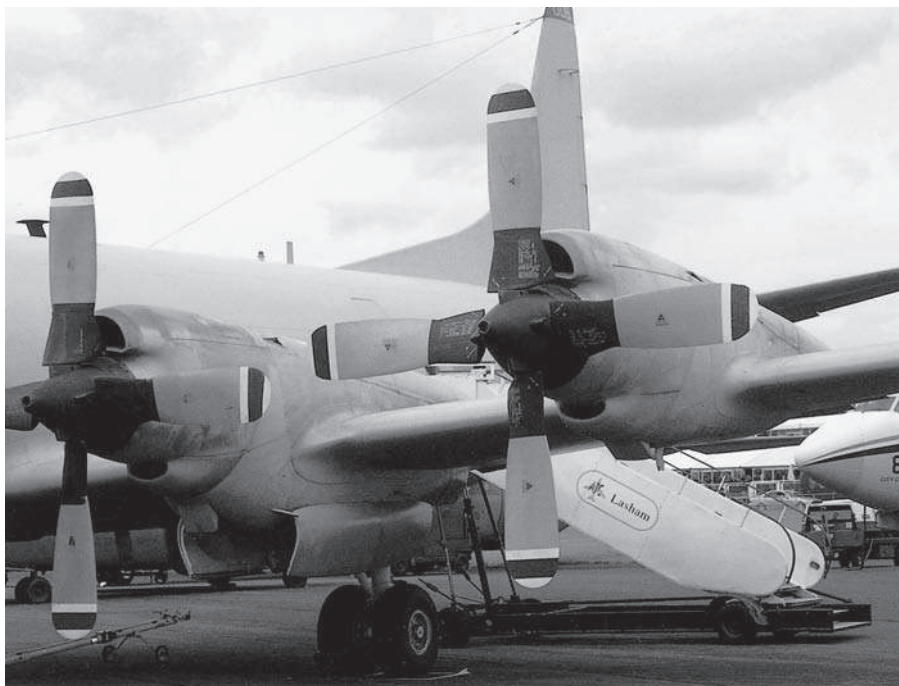
Fig 4B Turboprop propulsion The Lockheed Orion with four turboprops. Note the huge wide-chord 'paddle-blade' propellers.
