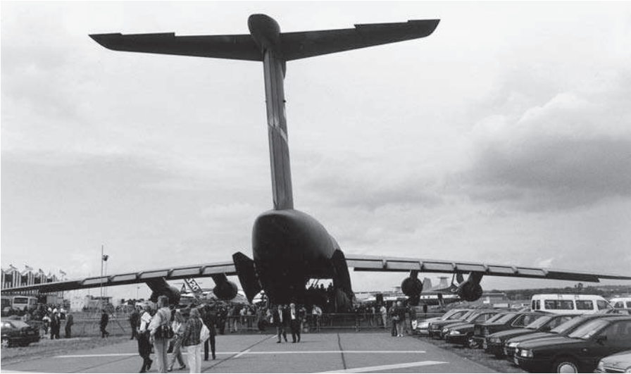
Fig 5F High tail The tail of a Lockheed C-5 Galaxy. The elevators are split into a number of sections to provide redundancy for reasons of safety.
