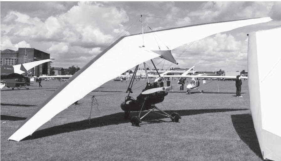
Fig 5D Tail-less – new type This popular form of powered microlight aircraft has been derived from hang-glider technology.
