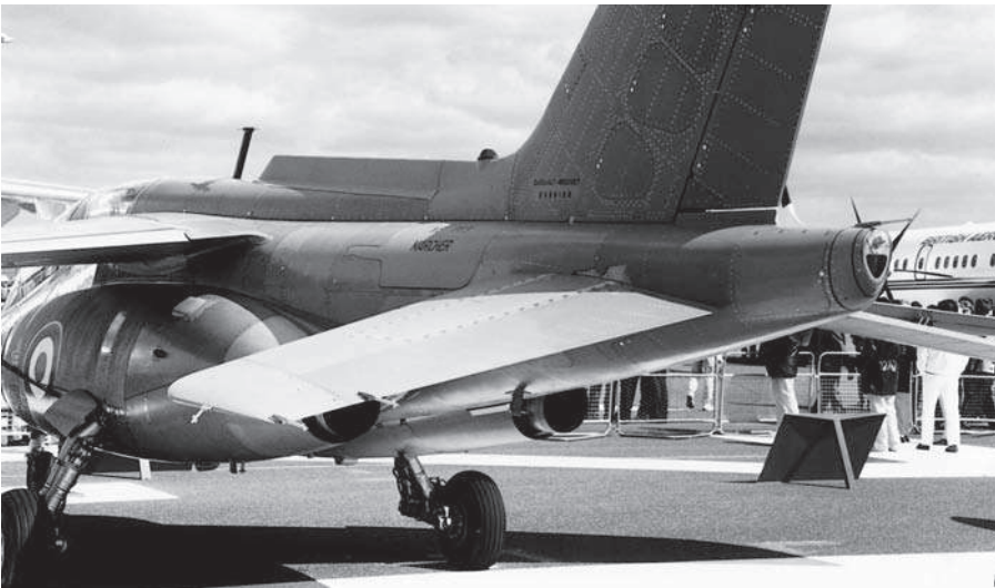
Fig 5G Low tail The Alpha-Jet has a relatively low tail plane with pronounced anhedral.
