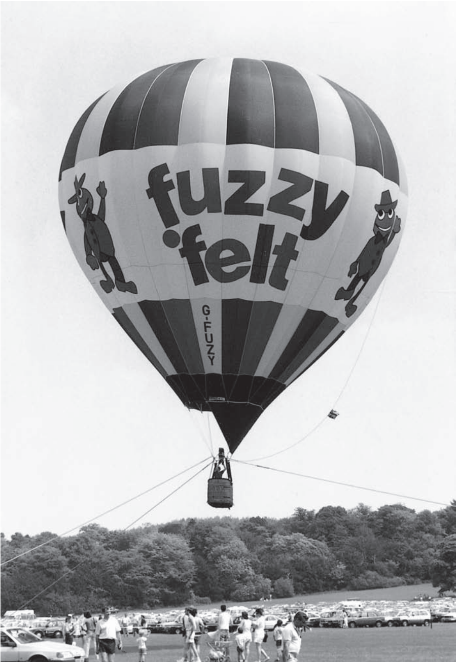
Fig 6H VTOL – another way After a century of neglect, the hot-air balloon has made a major comeback. This one is tethered and is being used for pilot training. The wicker basket provides good impact absorption on landing.
