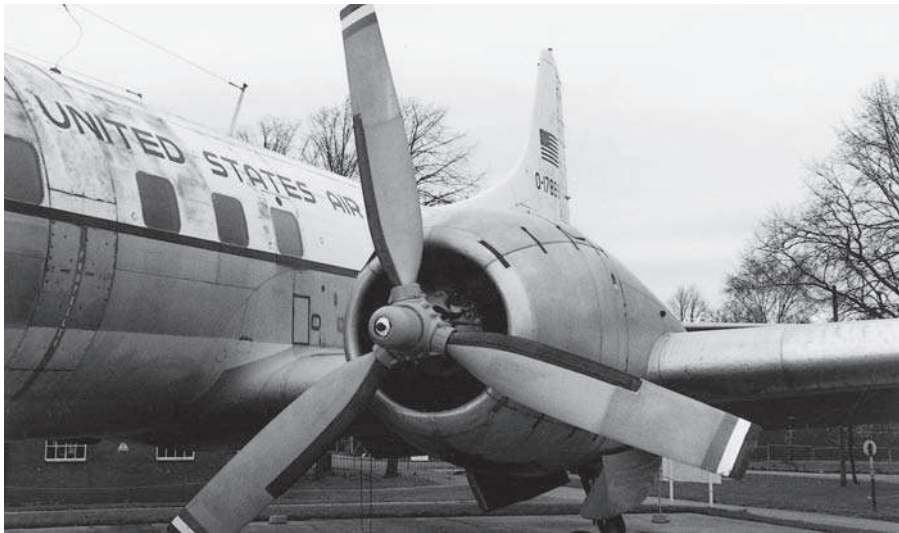
Fig 4J Constant-speed propeller
