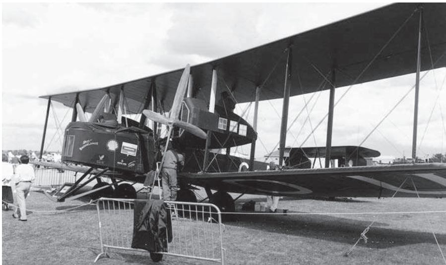
Fig 2A Parasite drag A flying replica of the Vickers Vimy bomber which was the first aeroplane to make a non-stop flight across the Atlantic (in 1919). The extensive use of bracing wires and struts creates a great deal of parasite drag.
