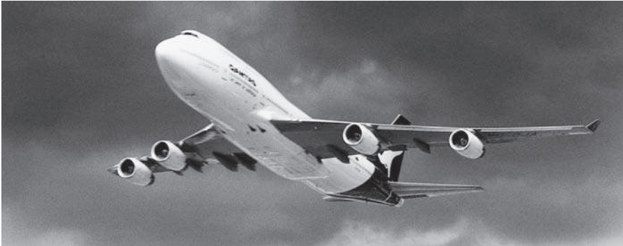
Fig 5A Long haul, large capacity This Boeing 747-400 'Jumbo' has 350 seats, and a range of 13 528 km that could take it from Europe to Australia non-stop.
