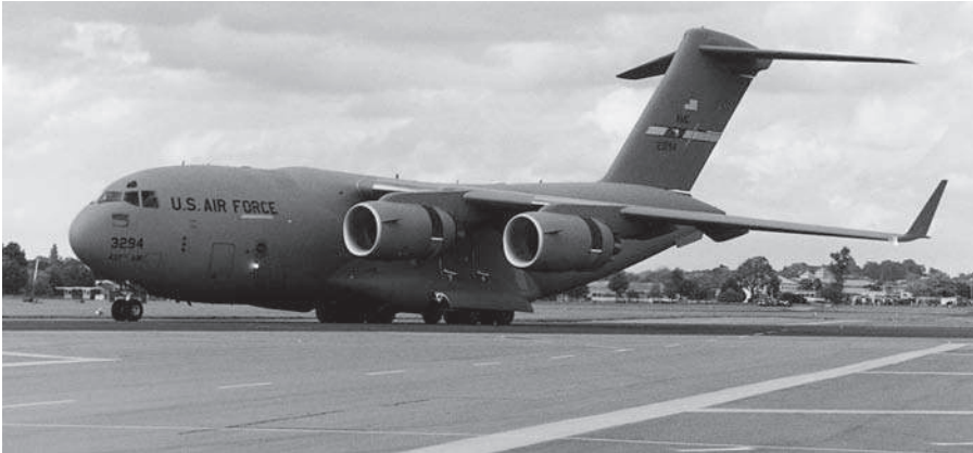
Fig 9E High fin A massive high fin and pronounced anhedral are evident on the McDonnell Douglas C-17.
