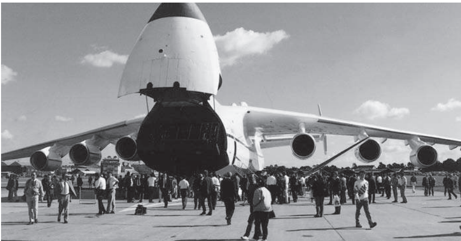
Fig 1A Weight and thrust The massive Antonov An-255 Mriya, with a maximum take-off weight of 5886 kN (600 tonnes). The six Soloviev D-18T turbofans deliver a total maximum thrust of 1377 kN.
