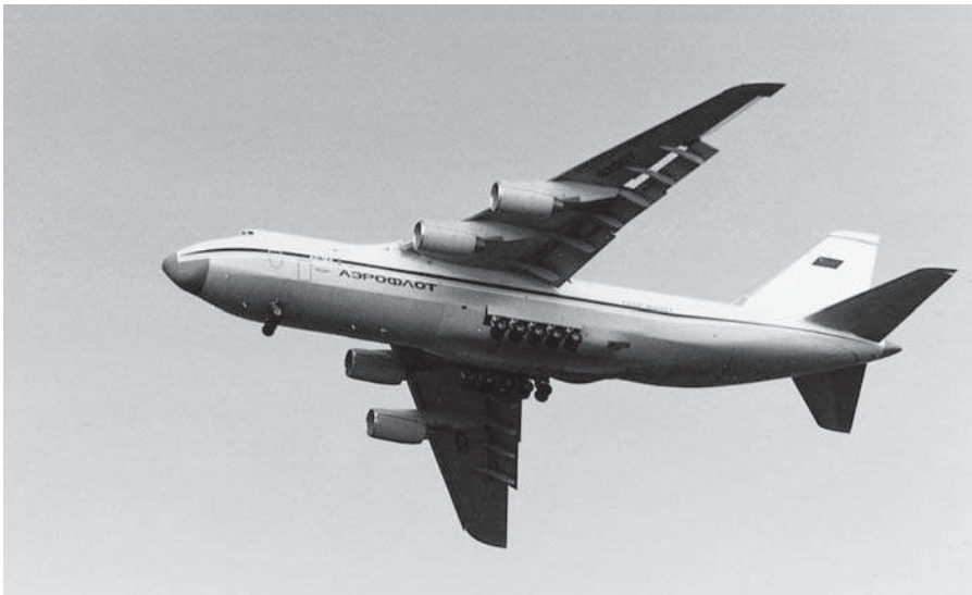
Fig 6I Ready for landing The huge Antonov AN-124 with Fowler flaps and leading edge slats extended, and undercarriage lowered, showing the ten pairs of main wheels.
