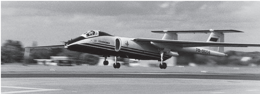
Fig 7A Taking-off The Myasischev M-55 high-altitude aircraft for surveillance and geophysics research.
