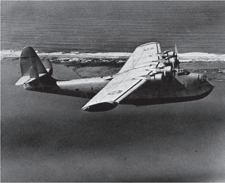
Fig 9F A classic flying boat (By courtesy of the General Dynamics Corporation, USA) The large side area of the hull was balanced, from the lateral stability point of view, by the dihedral on the main planes and the high fin at the rear.
