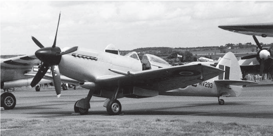
Fig 9A Dihedral Pronounced dihedral is evident on this Spitfire: a very late post-war model.
