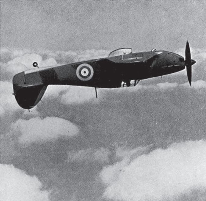
Fig 8C Inverted flight (By courtesy of 'Flight') And to illustrate upside-down flight, the Hurricane of the Second World War; note the tail-down attitude usually associated with inverted flight.
