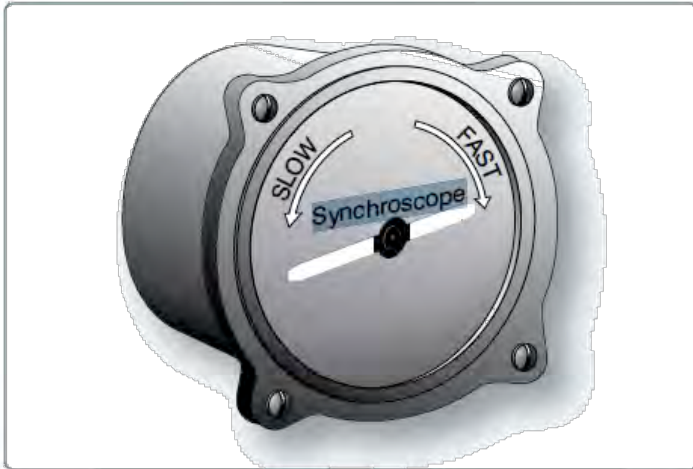
Figure 10-59. This synchroscope indicates the relative speed of the slave engine to the master.
