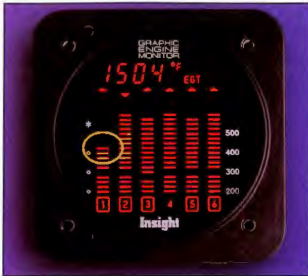
Figure 14-18. A low EGT may be the result of inadequate airflow into the cylinder.
