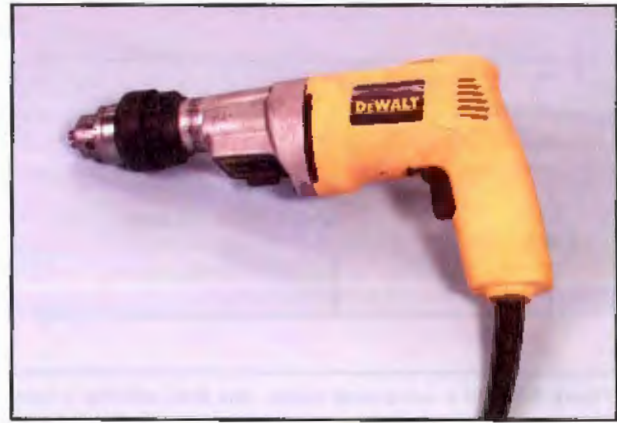
Figure 8-60. An electric drill uses a universal motor that is similar in construction to a series-wound DC motor.
