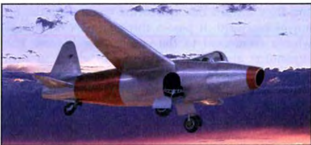
Figure 3-4. German engineer Hans Von Ohain designed and built the turbojet engine that powered the Heinkel He-178 in the world's first jet-powered flight in 1939.
