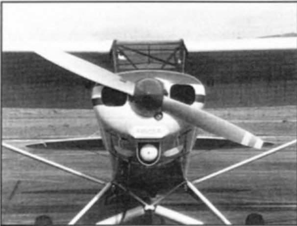
Figure 12-83. When installing a propeller on a four-cylinder opposed engine, one of the blades should come to rest at the ten o'clock position to reduce vibration and facilitate hand propping.
