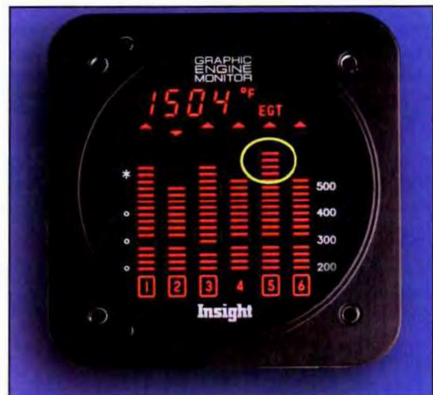
Figure 14-15. A rise in EGT in one cylinder may be the result of a lean mixture in that cylinder.
