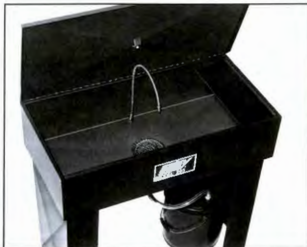
Figure 2-37. Several manufacturers produce fixtures that circulate an approved solvent for cleaning engine parts. These fixtures limit solvent splashes and provide containment for small parts that could otherwise be misplaced or lost.
