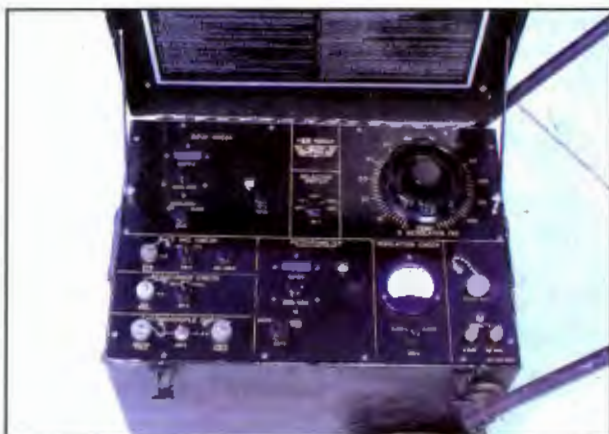
Figure 13-21. Engine indicating systems should be periodically checked during maintenance run-ups using special calibration equipment such as this Jetcal ® Analyzer.
