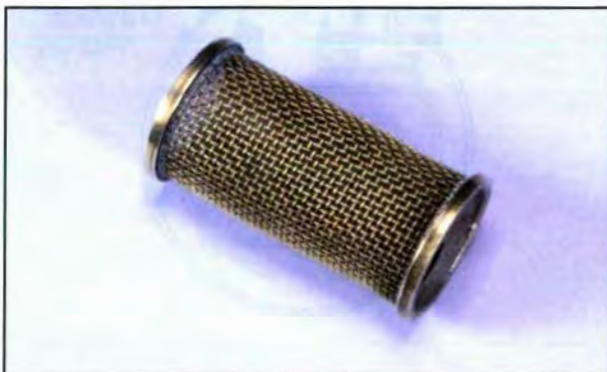
Figure 9-17. Many aircraft engines use a screen surface filtration oil strainer. An oil strainer filters out large particles and helps prevent other filtering elements from becoming clogged.
