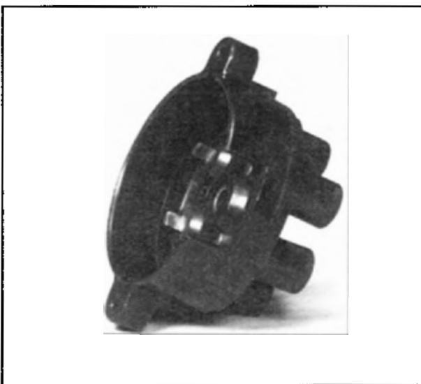
Figure 8-120. The distributor block of a typical magneto is made of an insulating material with electrodes on one side and receptacles for spark plug on the other.
