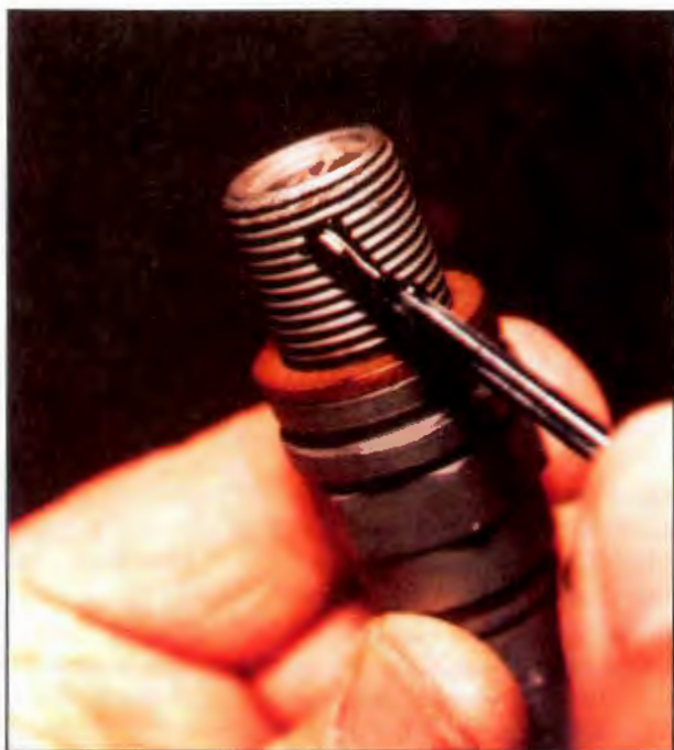
Figure 8-158. Sparingly apply antiseize compound to the second thread of each spark plug before installation.
