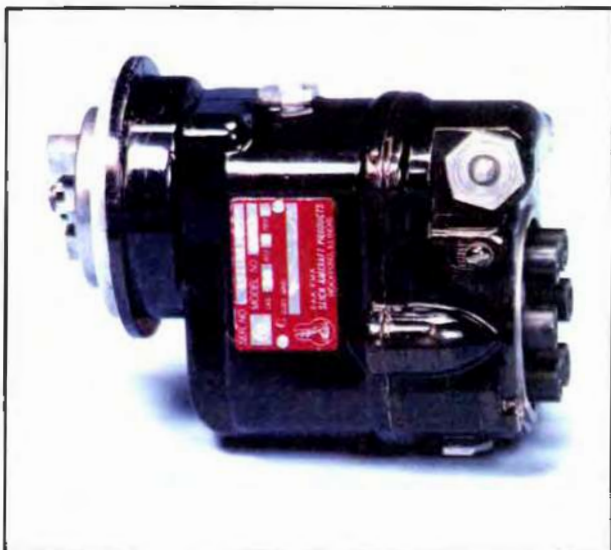
Figure 8-109. A single magneto uses a multi-pole magnet to induce current in a coil. The voltage pulse of current is stepped up and distributed to the spark plugs.
