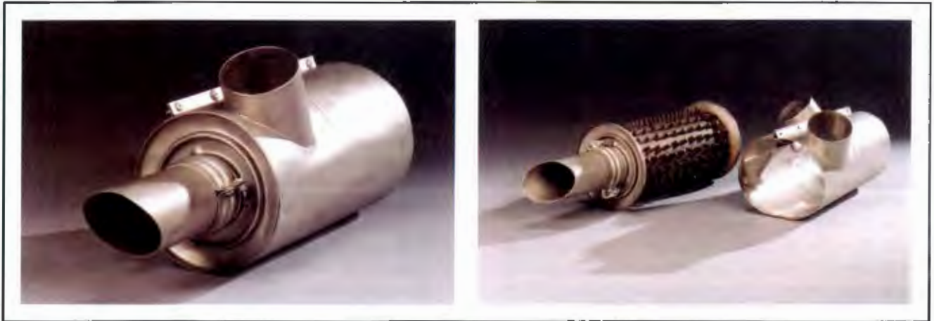
Figure 6-5. On the left, the shroud is installed on the muffler. The shroud is typically held to the muffler with stainless steel screws. On the right, the shroud is removed. The knobs on the muffler transfer heat from the muffler to the air space within the shroud.
