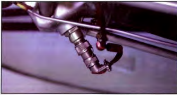
Figure 13-17. Inspect the condition and operation of all magnetic chip detectors. Operational checks are performed by removing the detector from the engine or accessory case and with the wiring still connected to the detector, bridge across the detector's poles with a metallic tool. When bridged, the chip detection warning light should illuminate.
