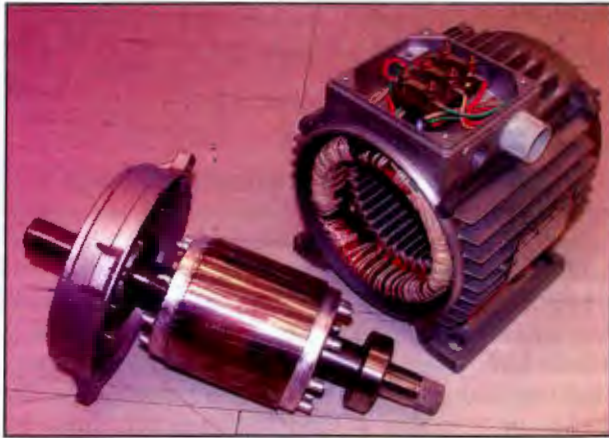
Figure 8-61. There is no electrical connection between the rotor and the stator of an induction motor.
