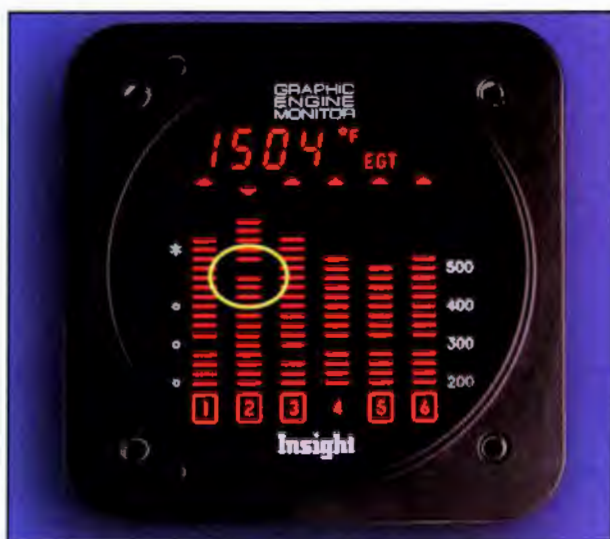
Figure 14-16. A high CHT in one cylinder may be the result of cracked cylinder fins.
