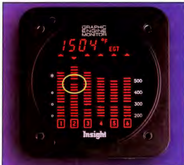
Figure 14-19. A broken or cracked exhaust manifold may direct hot exhaust gases on a CHT probe, causing an extremely high CHT in one cylinder.
