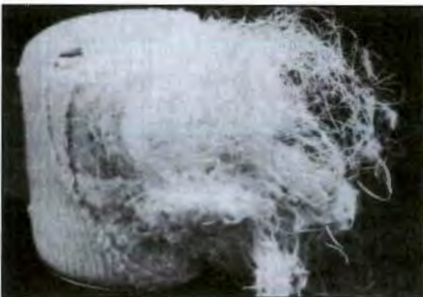
Figure 9-14. A depth filter consists of a closely-packed fiber matrix element.
