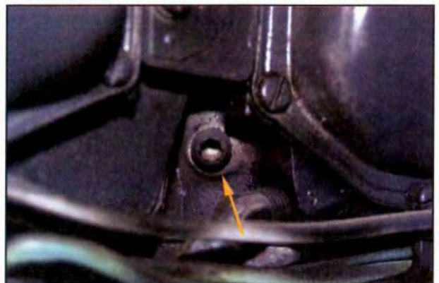
Figure 14-13. A missing primer plug allows ambient air to be drawn into the intake port of the cylinder, causing an excessively lean mixture.
