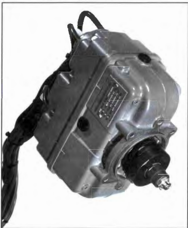
Figure 8-110. The Bendix D-3000 dual magneto contains two separate and independent ignition systems that share a common driveshaft and four pole rotating magnet.
