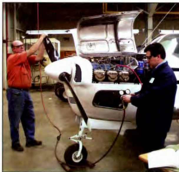
Figure 13-13. A compression test is used to help determine the internal condition and "health" of an engine.
