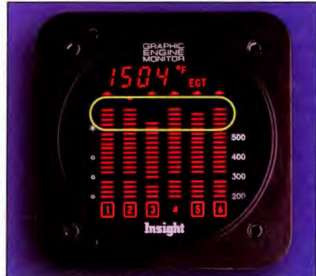
Figure 14-20. A temperature increase or decrease in all cylinders may be the results of improper timing.
