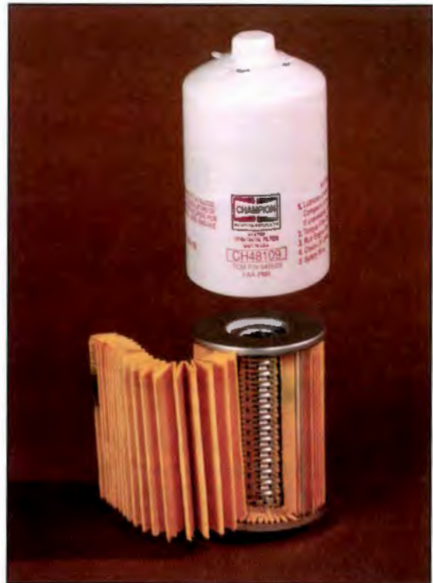
Figure 9-15. A typical spin-on, semi-depth filter consists of a pleated sheet of resin-impregnated fibers arranged around a perforated steel core. The entire element is contained within a thin metal housing.
