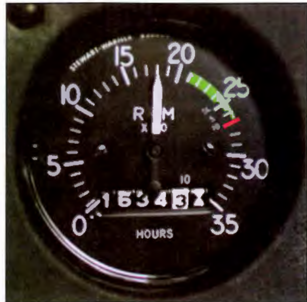
Figure 2-17. The tachometer is a primary engine instrument which provides engine r.p.m. indications. A typical tachometer instrument face is calibrated in hundreds of r.p.m. and has both a green arc and red line.
