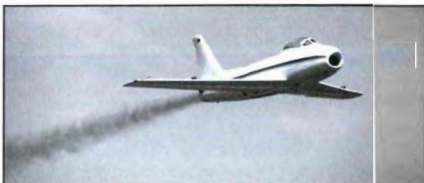
Figure 3-19. The single-entrance inlet duct takes full advantage of ram effect much like engine-mounted air inlet ducts. Although the aircraft is aerodynamically clean, the length of the duct makes it less efficient than engine-mounted types.
