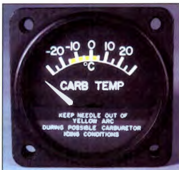
Figure 2-3. This carburetor air temperature gauge highlights the danger of induction system icing when the temperature is between -15^{\circ}\text{C} to +5^{\circ}\text{C} .
