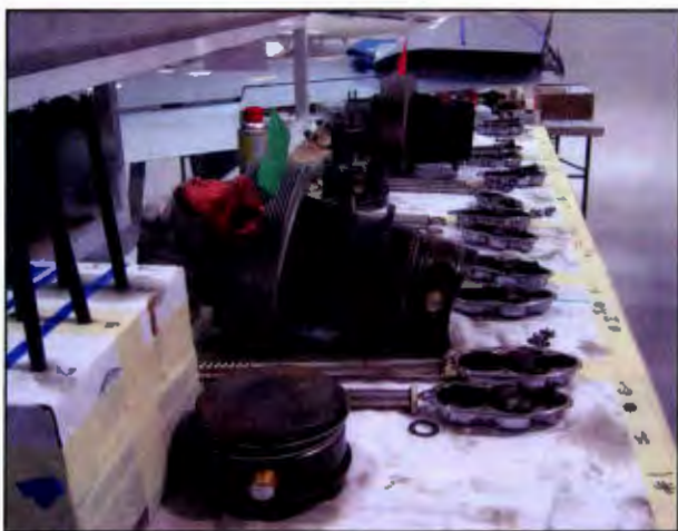
Figure 2-36. Engine parts are laid out in an orderly fashion on a clean workbench after cleaning to facilitate inspection. Keeping parts arranged in an orderly manner minimizes loss or accidental damage.
