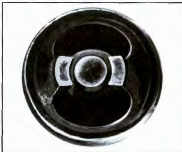
Figure 8-149. A light deposit of dull brown material on a spark plug insulator indicates normal combustion is occurring in the cylinder.
