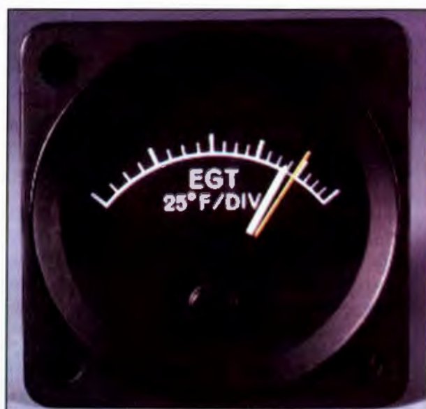
Figure 2-16. The fuel/air mixture can be set for best fuel efficiency by using an EGT gauge and following the aircraft checklist instructions.
