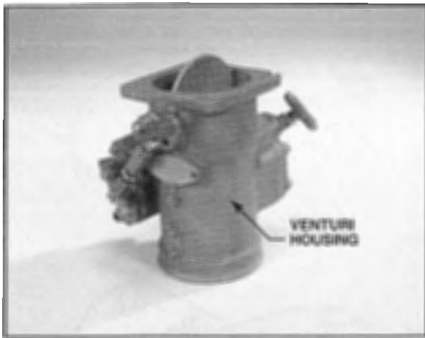
Figure 7-49. A typical venturi housing is a single piece of cast aluminum with a venturi pressed into one end. A throttle valve is installed on the other end.
