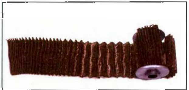
Figure 13-16. When changing oil during an inspection, the oil filter should be opened so you can check for metal particles or other contamination.
