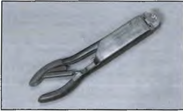
Figure 8-95. When a pin or socket is inserted into the crimper, insert the wire until it bottoms out before squeezing the handles. The handles will not release until the crimping process is complete. Ratchet-type crimping tools are periodically calibrated to ensure that a quality crimp is provided.
