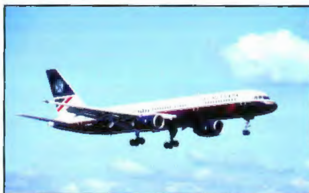
Figure 5-18. A Boeing 757 has wing-mounted engines that use engine-mounted inlet ducts directly in front of the compressor.
