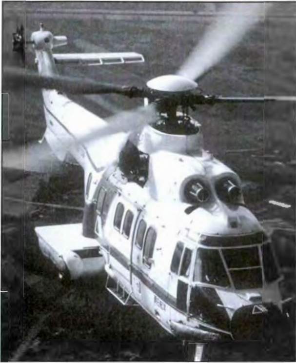
Figure 3-21. Several makes of helicopters and turboprop aircraft use inlet screens to help prevent foreign object damage.
