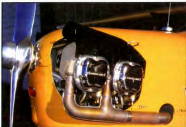
Figure 10-3. The cowling on early horizontally opposed engines consisted of a thin sheet metal hood that forced cooling air through the cylinder fins.
