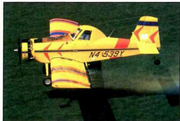
Figure 10-1. A Townend ring, or speed ring, reduces the drag caused by air flowing over the cylinders of radial engines.
