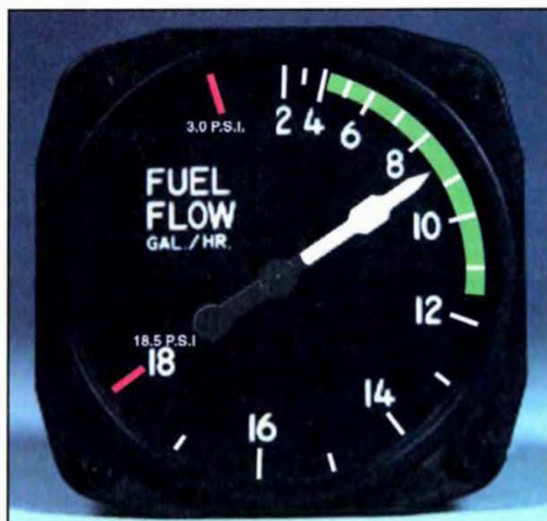
Figure 2-8. A typical fuel flow indicator displays the number of gallons (or pounds) per hour an engine consumes. Normal fuel flow indicated by this gauge is between 4.25 and 11.5 g.p.h.
