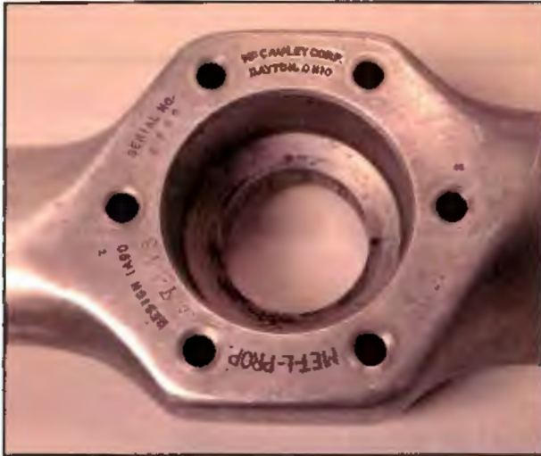
Figure 12-18. An aluminum propeller has information stamped on the hub to identify hub design, blade design, blade length, and pitch. The number 1 stamped on the blade root identifies installation position.
