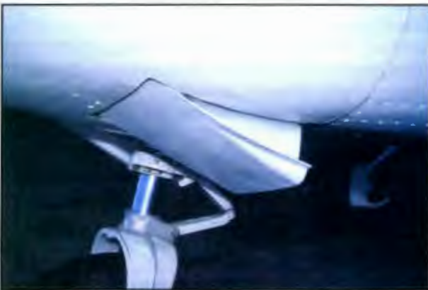
Figure 10-6. By adjusting cowl flap position on an aircraft, the operator can control the amount of air that flows through the cowling.
