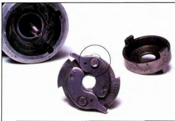
Figure 14-10. A broken flyweight spring prevents an impulse coupling from retarding ignition for starting.
