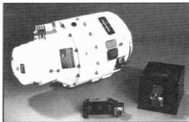
Figure 8-44. The constant speed drive unit is included in the housing with the Sundstrand Integrated Drive Generator. The generator requires the use of a control unit and a current transformer assembly.
