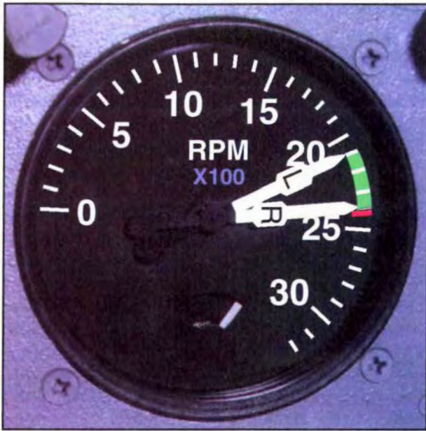
Figure 2-21. Multi-engine aircraft are sometimes equipped with a single tachometer that provides r.p.m. indications for both engines. The needle with an "R" represents the right engine while the needle with an "L" represents the left engine.
