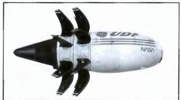
Figure 3-13. Research in unducted fan engines points to greater fuel efficiency for future transport aircraft.
