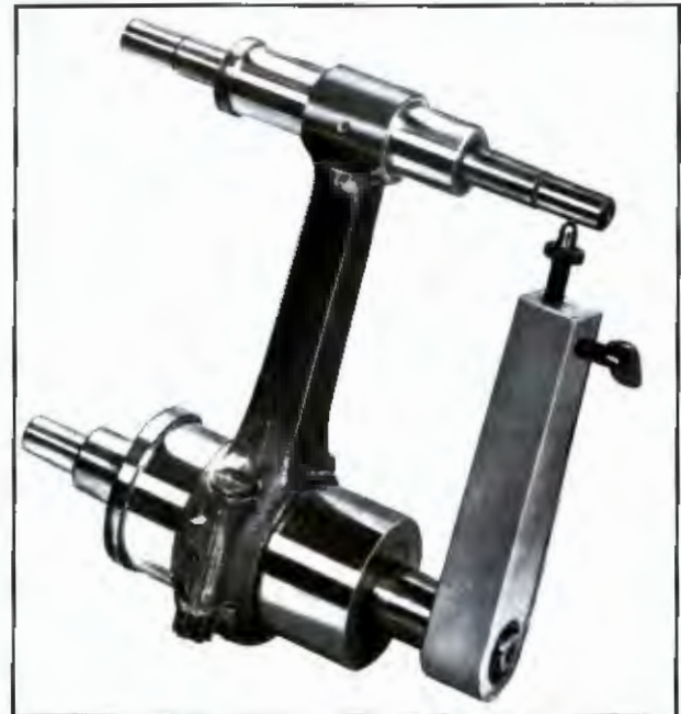
Figure 2-48. To check a connecting rod for convergence, mount a parallelism gauge to one end of the large arbor and measure the distance between the arbors on both sides. The difference in the measurements is the amount of bend in the rod.
