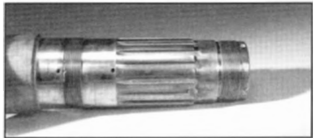
Figure 1-56. All splined propeller shafts are identified by an SAE number. For example, SAE 50 identifies a splined shaft that meets SAE design specifications for a 50 size shaft. The SAE number does not refer to the number of splines.
