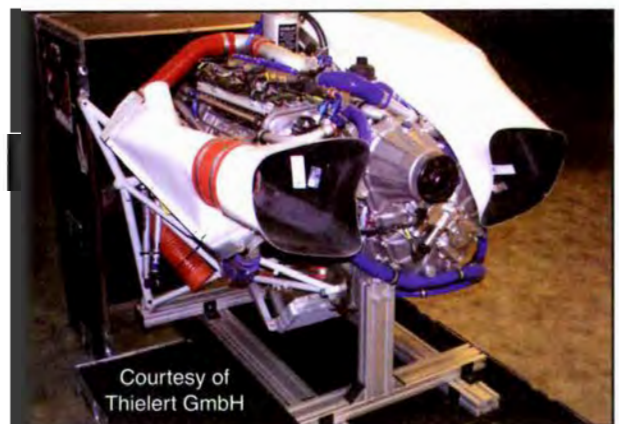
Figure 2-71. Engines that need repairs or overhaul must be protected during storage and shipment. For this reason, shipping crates or containers tailored to a specific engine model must always be used to transport the engine.
