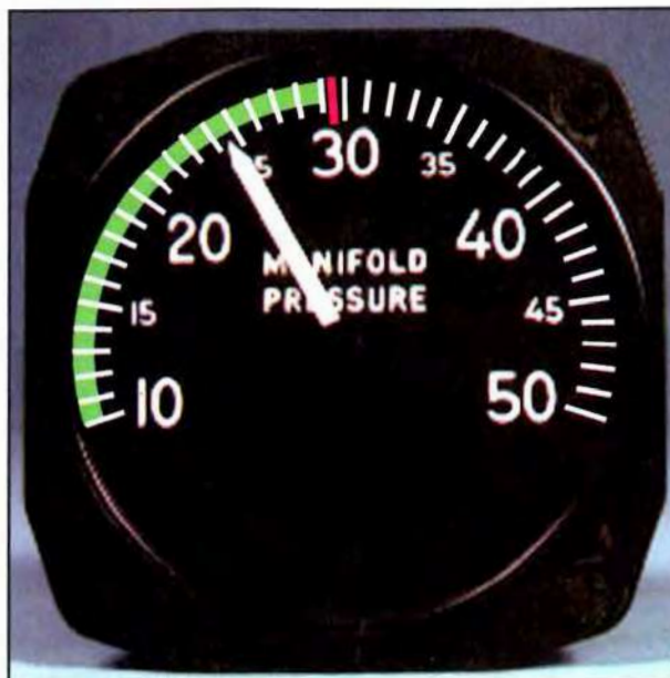
Figure 2-9. A manifold absolute pressure gauge displays absolute air pressure in the engine's intake manifold in inches of mercury. The green arc indicates the normal operating range and the red line indicates maximum allowable manifold pressure.
