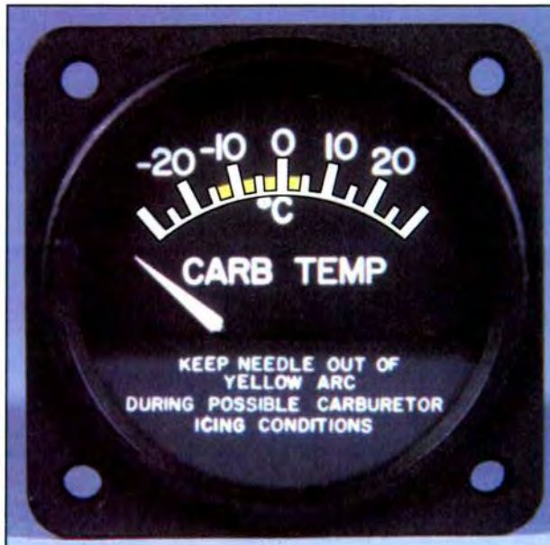
Figure 5-3. This carburetor air temperature gauge indicates that the danger of induction system icing exists when the temperature is between -15^{\circ}\text{C} to +5^{\circ}\text{C} .
