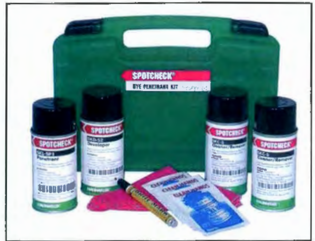
Figure 2-44. Portable test kits of dye penetrant are available for inspecting localized areas on an aircraft.
