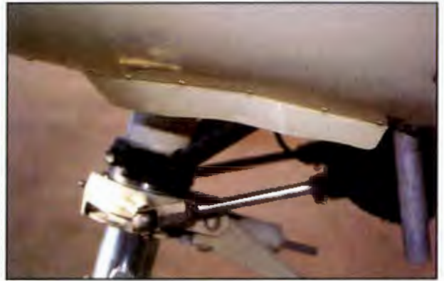
Figure 10-4. The flared portion of a lower cowl helps produce a low-pressure area at the cowl exit, which draws inlet air down through the cylinders.
