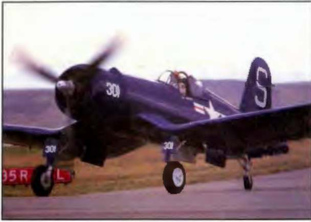
Figure 10-2. Radial engines enclosed in NACA cowlings produce less drag and have improved engine cooling.
