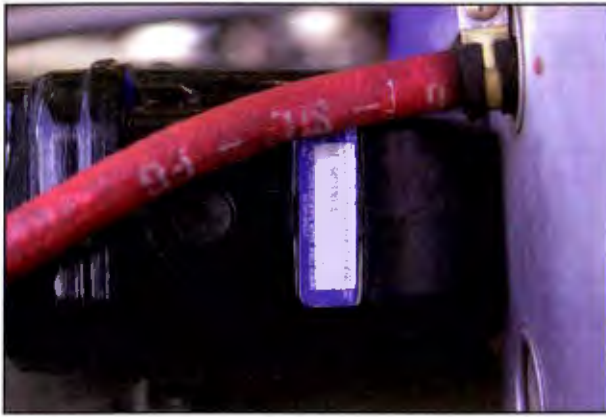
Figure 13-5. Visually confirm appliance data tag information and record it on a form during appliance AD checks.
