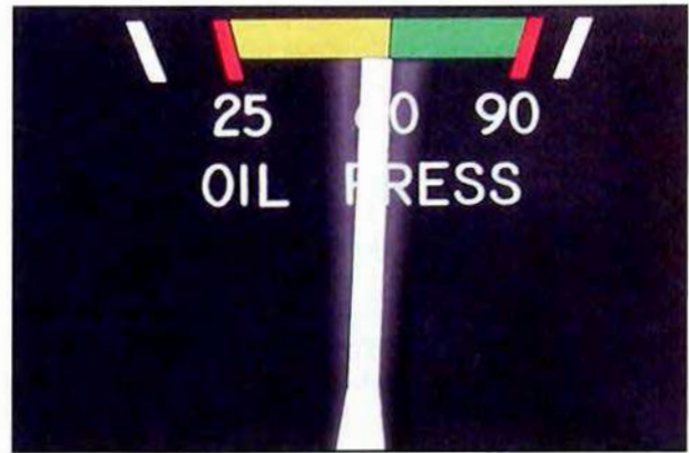
Figure 14-11. A fluctuating oil pressure gauge may indicate an impending failure in the engine.
