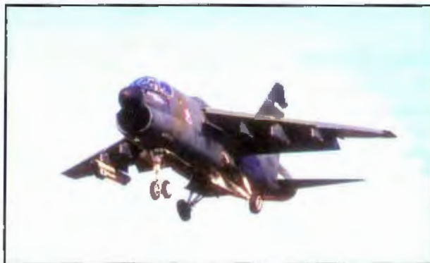
Figure 5-20. The single-entrance inlet duct takes full advantage of ram effect much like engine-mounted air inlets. Although the aircraft is aerodynamically clean, the length of the duct makes it slightly less efficient than the shorter length of side-mounted types or those ahead of wing-mounted engines.
