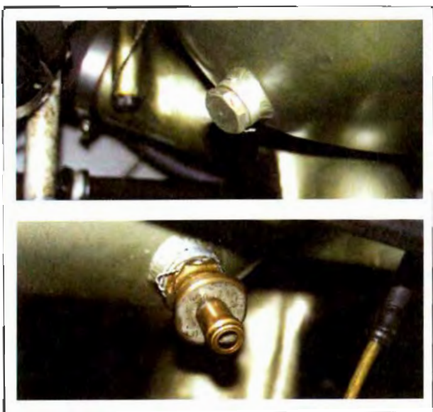
Figure 9-24. Most of the engine oil in a typical horizontally opposed engine is drained by removing one or more oil drain plugs or by opening a drain valve.
