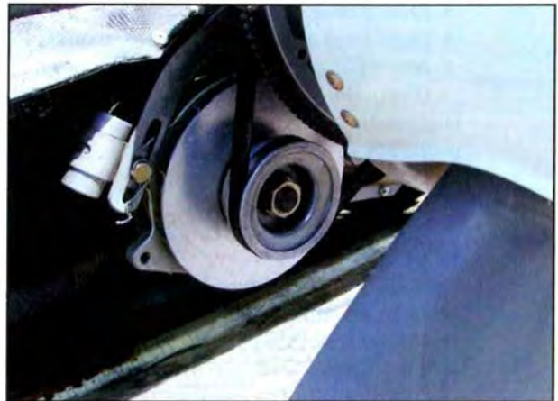
Figure 14-6. Inadequate belt tension is a possible cause of low voltage on the electrical system of a small airplane.
