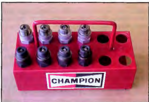
Figure 8-148. Spark plug trays provide a secure, organized place to store spark plugs when you remove them for service.
