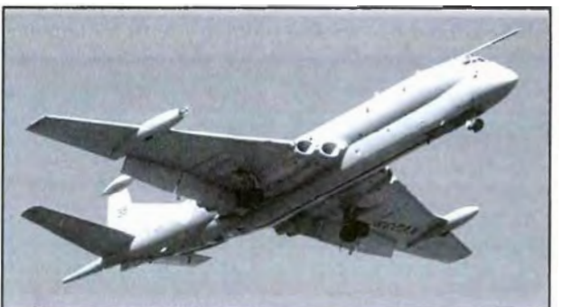
Figure 3-18. The Hawker-Siddeley 801 "Nimrod" uses aerodynamically shaped, wing-mounted air inlet ducts to reduce drag.
