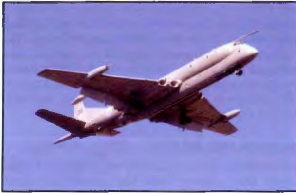
Figure 5-19. The Hawker-Siddeley 801 Nimrod was developed from the de Havilland Comet airframe and uses wing-mounted air inlets that are aerodynamically shaped to reduce drag.
