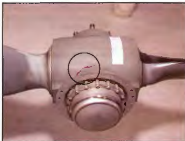
Figure 13-26. For some constant-speed propellers, red-colored oil coming from the propeller hub is indicative of a crack. If red oil is detected, the propeller must be removed for servicing at an authorized propeller repair facility.
