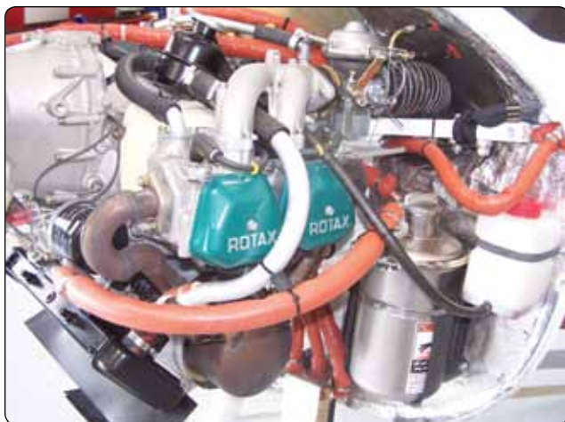
Figure 11-6. Typical four cylinder, four-stroke horizontally opposed engine.
