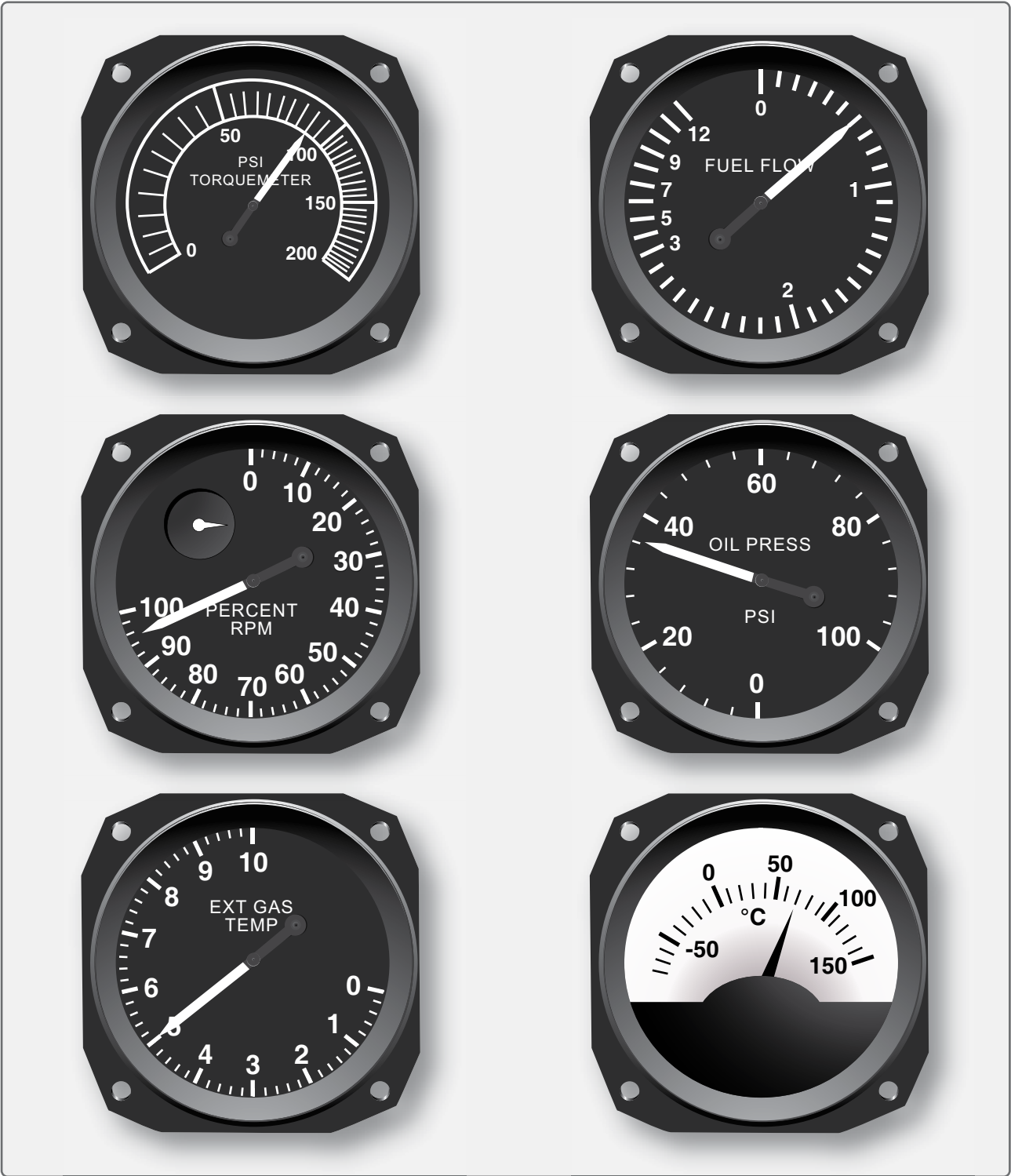
Figure 10-73. Typical turbine engine instruments.
