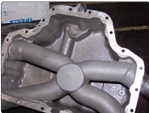
Figure 6-17. Wet-sump system's sump with intake tube running through it.
