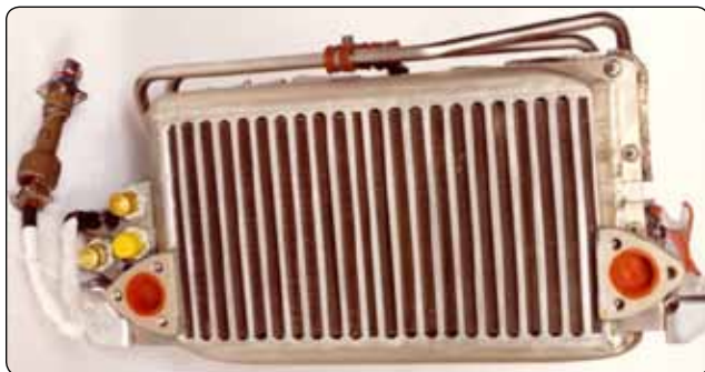
Figure 6-42. Air oil cooler.
