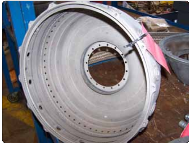
Figure 10-63. Combustion case inspection.
