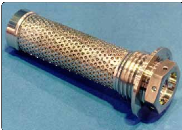
Figure 6-36. Last-chance filter before spray nozzle.
