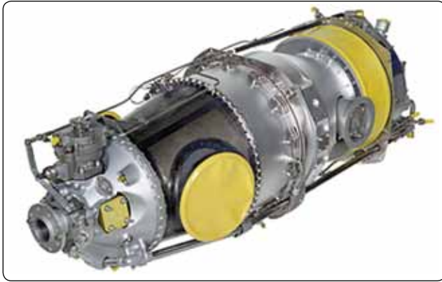
Figure 7-44. Pratt & Whitney PT6 engine.
