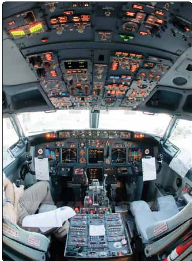
Figure 9-12. Engine fire switches.
