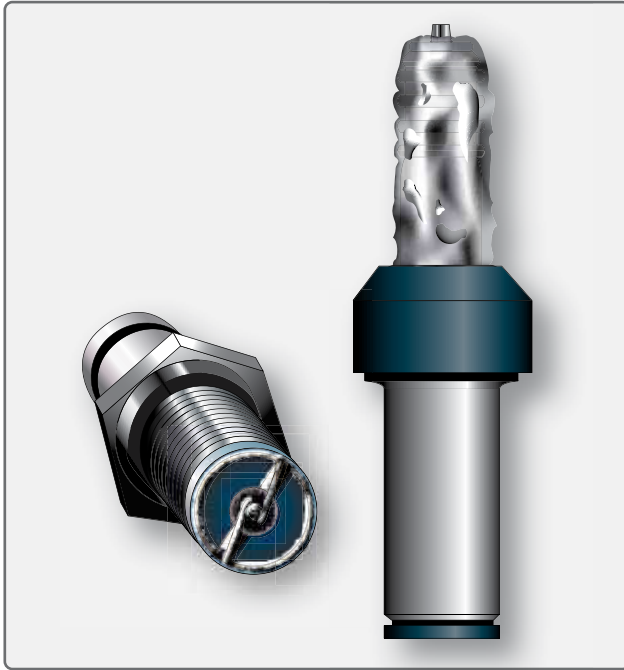
Figure 4-49. Lead fouled spark plug.
