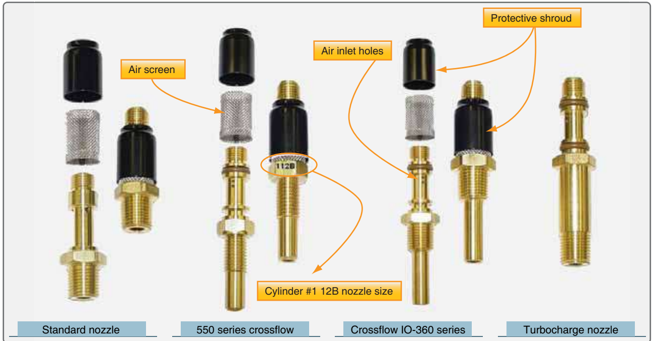
Figure 2-45. Fuel discharge nozzles.
