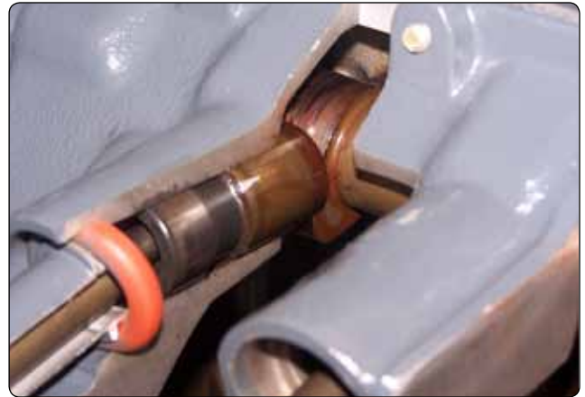
Figure 1-29. Cam load on lifter body.
