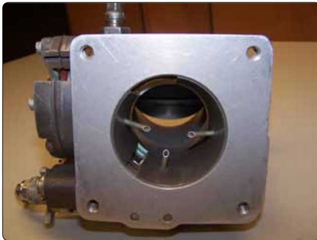
Figure 2-32. Impact tubes for inlet air pressure.
