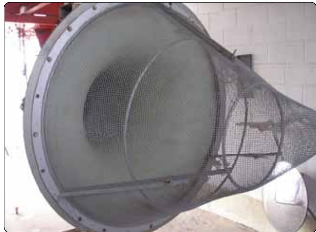
Figure 3-30. A bellmouth inlet used during system tests.
