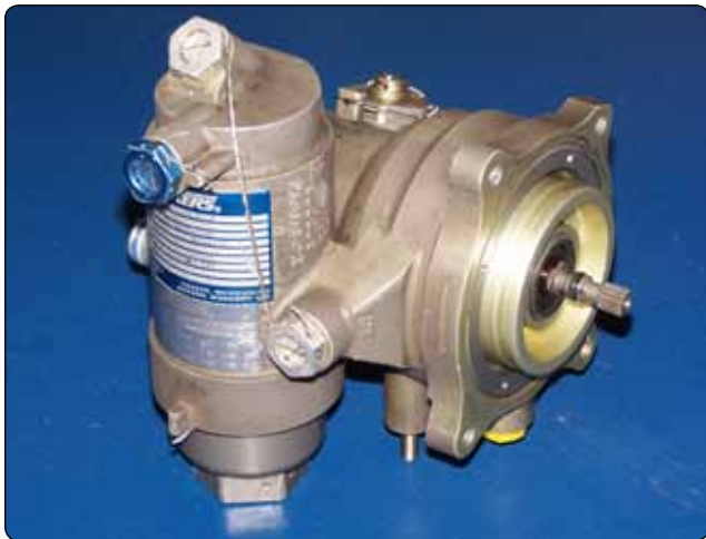
Figure 2-50. Fuel pump and filter.
