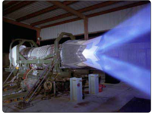
Figure 3-51. A pilot can direct thrust via the vectoring nozzle 20^\circ up or down to increase flight maneuverability.
