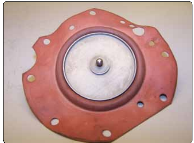
Figure 2-33. Fuel diaphragm with ball valve attached.
