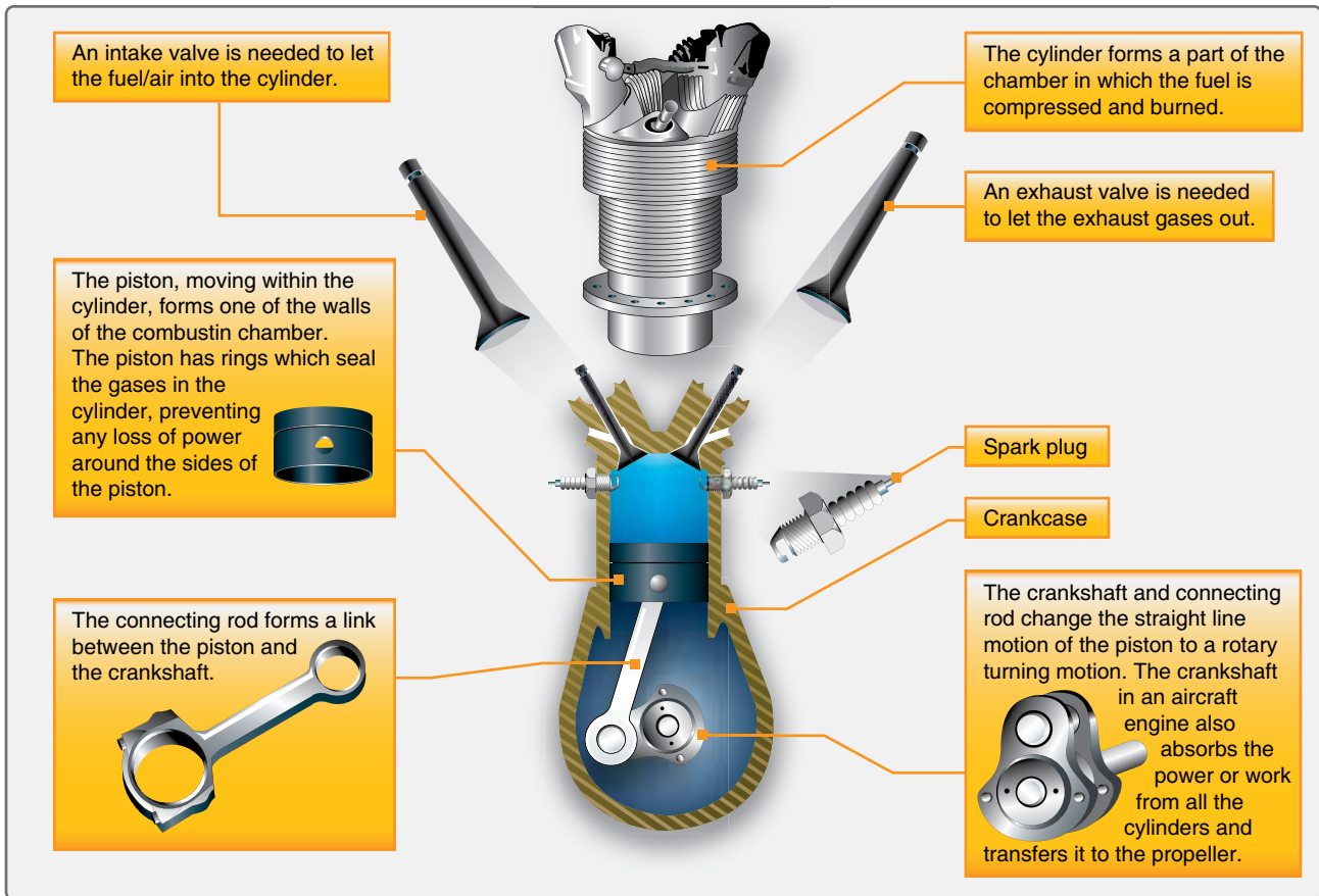
Figure 1-4. Basic parts of a reciprocating engine.
