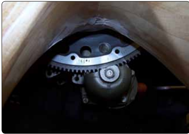
Figure 4-46. Timing marks aligned.
