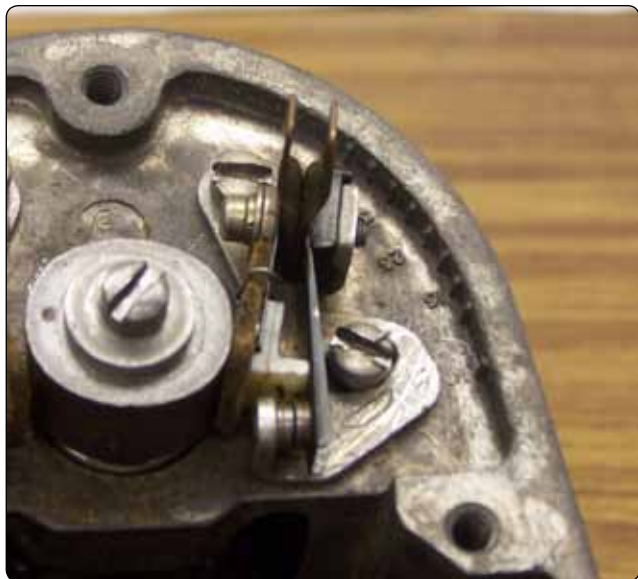
Figure 4-8. Pivotless type breaker assembly and cam.
