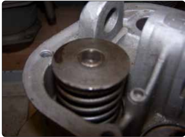
Figure 1-22. Stem keys forming a lock ring to hold valve spring retaining washers in place.
