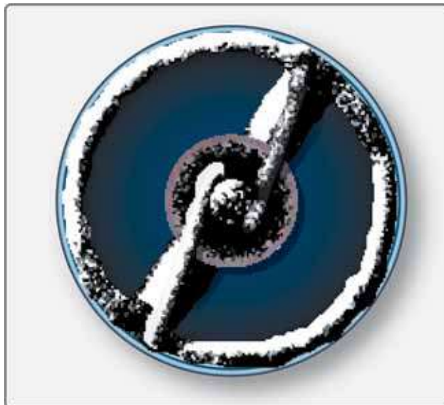
Figure 4-48. Carbon fouled spark plug.
