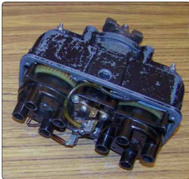
Figure 4-18. A dual magneto with two distributors.
