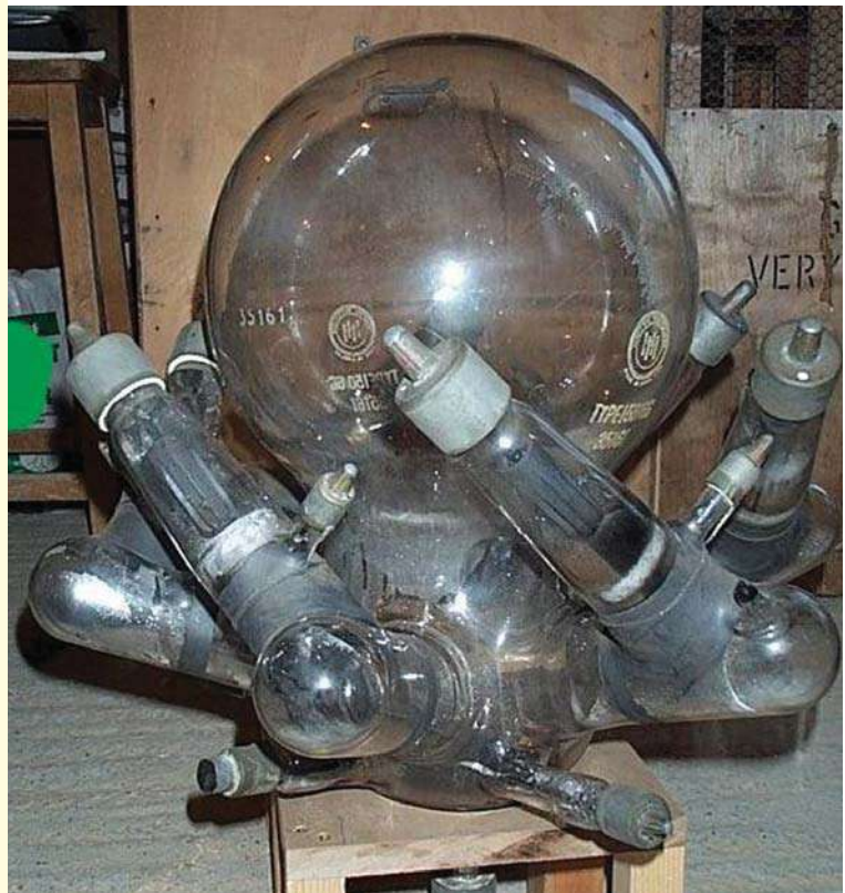
↑ This is a mercury arc rectifier 6-phase device, 150 A rating with grid control
