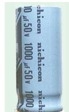
A cylindrical Capacitor
