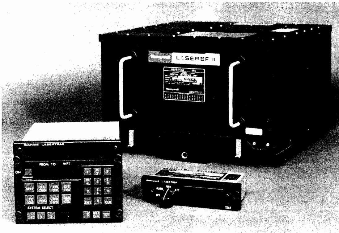
FIGURE 17-44 The components of a laser inertial reference system. (Honeywell Sperry Commercial Flight Systems Division)
