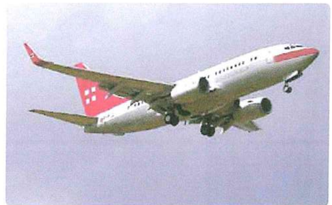
Figure 3-17. A winglet reduces induced drag caused by air spilling off of the wingtip.
