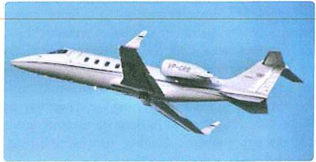
Figure 2-20. Winglets help reduce induced drag.
