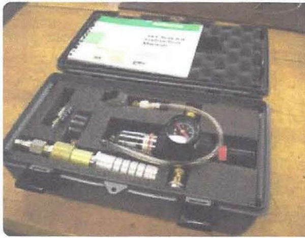
Figure 12-33. Test equipment used to test a wing de-ice system (left), and test equipment installed in the aircraft for testing (right).
