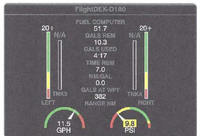
Figure 10-42. An electronic display of fuel parameters, including fuel pressure.
