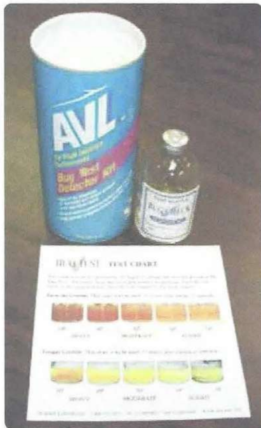
Figure 10-59. Fuel bug test kits identify the level of bacteria and fungus present in a fuel load by comparing the color of a treated sample with a color chart.
