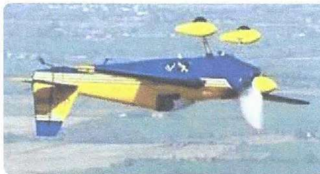
Figure 10-1. Aircraft fuel systems must deliver fuel during any maneuver for which the aircraft is certified.
