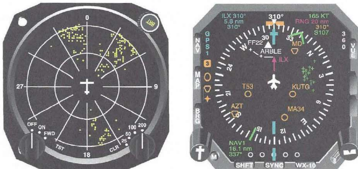
Figure 5-162. A dedicated stormscope lightning detector display (left), and an electronic navigational display with lightning strikes overlaid in the form of green "plus" signs (right).
