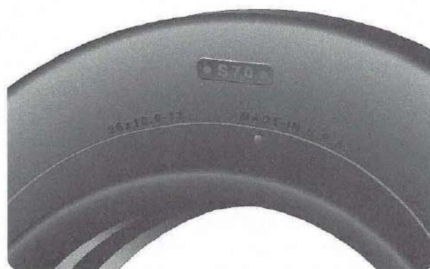
Figure 13-120. A sidewall vent marked by a colored dot must be kept free from obstruction to allow trapped air or nitrogen to escape from the carcass plies of the tire.
