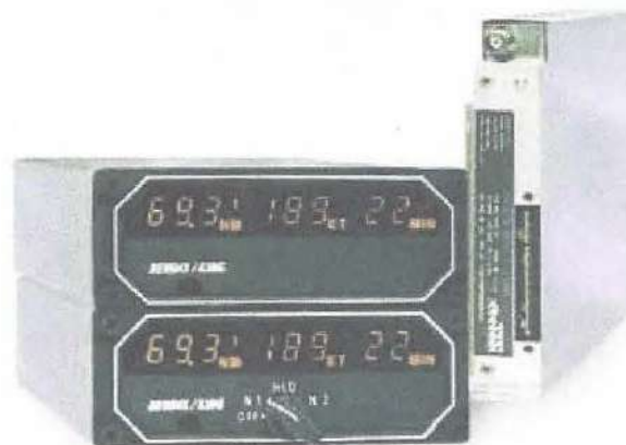
Figure 5-137. Distance information from the DME can be displayed on a dedicated DME instrument or integrated into any of the electronic navigational displays found on modern aircraft. A dual display DME is shown with its remote mounted receiver.
