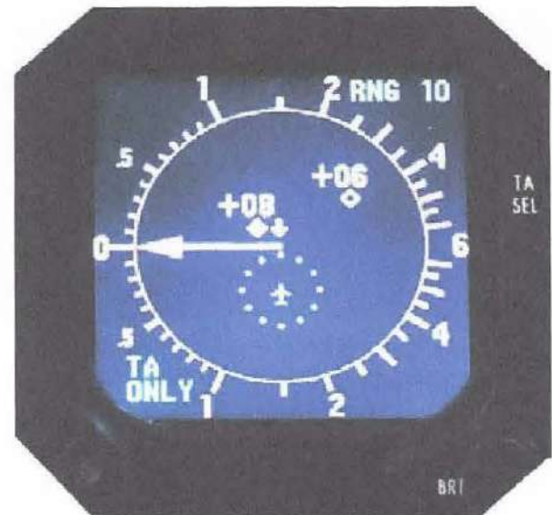
Figure 5-149. TCAS information displayed on an electronic vertical speed indicator.
