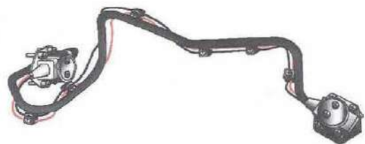
Figure 8-7. Pneumatic dual fire/overheat detector assembly.
