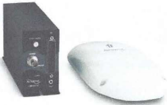
Figure 5-161. A receiver and antenna from a lightning detector system.
