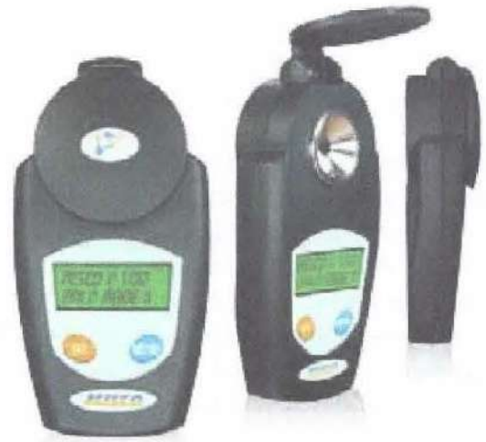
Figure 10-53. A hand-held refractometer with digital display measures the amount of fuel anti-ice additive contained in a fuel load.
