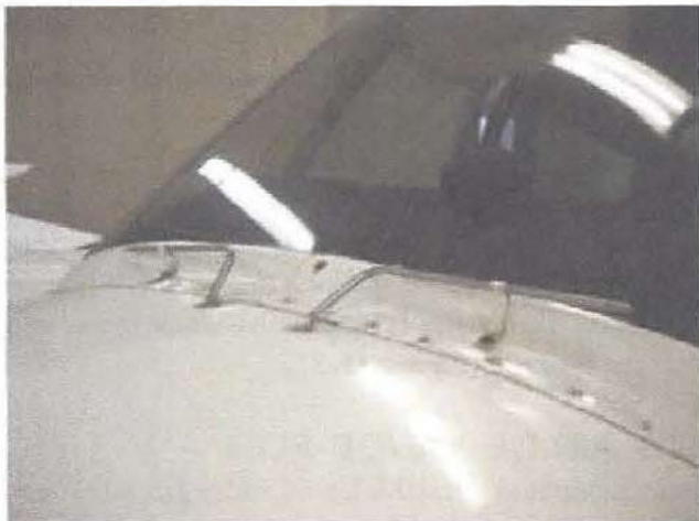
Figure 12-38. Chemical de-icing spray tubes.
