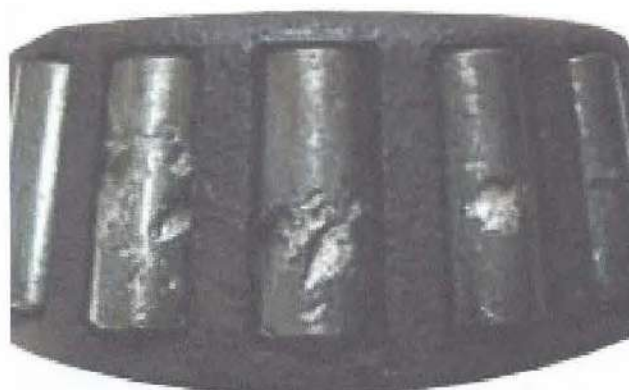
Figure 13-60. Spalling is a chipped away portion of the hardened surface of a bearing roller or race.
