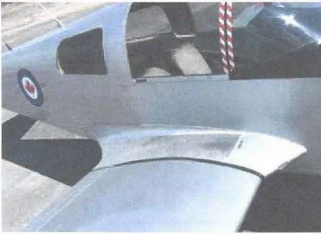
Figure 3-20. Wing root fairings smooth airflow and hide wing attach fittings.
