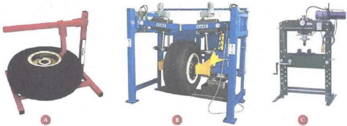
Figure 13-54. Tire beads must be broken from the wheel to remove the tire. A mechanical removal tool designed for breaking the bead is shown in (A); a hydraulic press designed with the capacity for large aircraft wheels is shown in (B); and an arbor press is shown in (C). All are tools available to the technician for this purpose.
