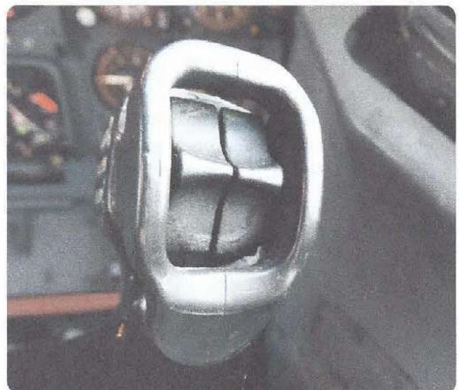
Figure 9-19. Trim Switches for the Horizontal Stabilizer. Both switches must be activated simultaneously to engage the trim motor. Upward movement of the switches commands a nose down reaction and downward movement of the switches provide a nose up change in flight attitude.
