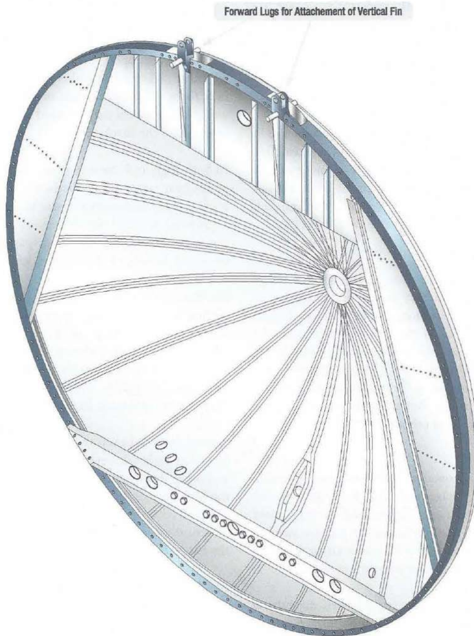
Figure 3-2. Vertical stabilizer attach points on the top of a pressure bulkhead.
