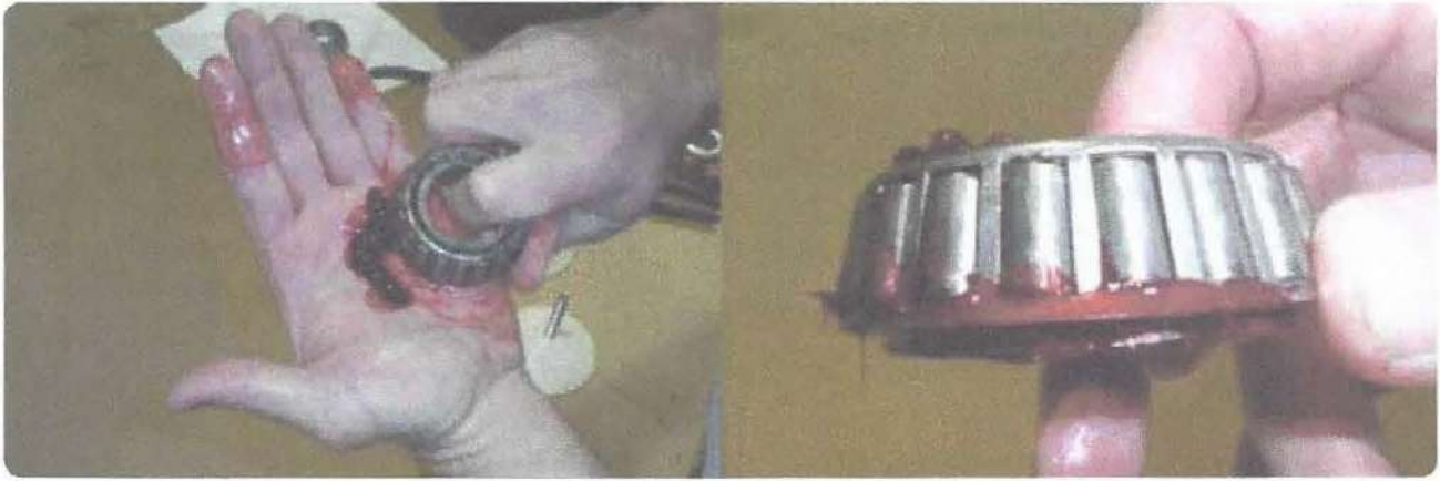
Figure 13-69. Packing grease into a clean, dry bearing can be done by hand in the absence of a bearing grease tool. Press the bearing into the grease on the palm of the hand until it passes completely through the gap between the rollers and the inner race all the way around the bearing.
