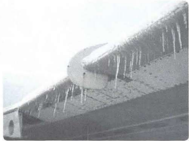
Figure 12-1. Formation of ice on aircraft leading edge.
