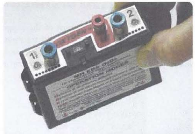
Figure 15-24. A portable two person electronic pulse-demand (EPD) oxygen regulating unit.
