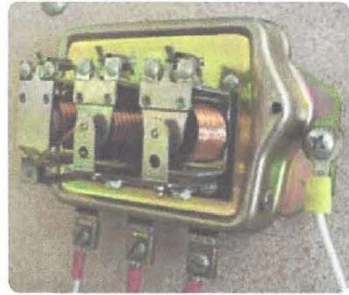
Figure 6-26. The three relays found on this regulator are used to regulate voltage, limit current, and prevent reverse current flow.
