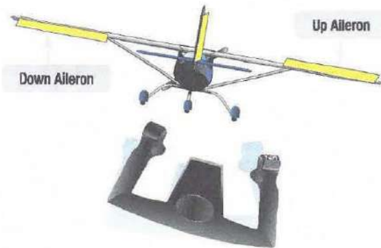
Figure 1-6. Differential aileron control movement. When one aileron is moved down, the aileron on the opposite wing is deflected upward.
