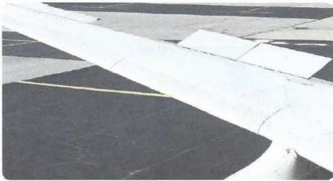
Figure 9-2. Flight Spoilers. Note how the flight spoilers, outboard of the engine, move up with the aileron (shown near the tip of the wing).
