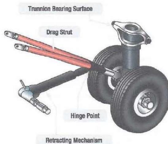
Figure 13-17. A hinged drag strut holds the trunnion and gear firm for landing and ground operation. It folds at the hinge to allow the gear to retract.
