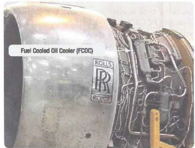
Figure 10-39. Jet transport aircraft fly at high altitudes where temperatures can reach -50^{\circ}\text{F} . Most have fuel heaters somewhere in the fuel system to help prevent fuel icing. This fuel-cooled oil cooler on an RB211 turbofan engine simultaneously heats the fuel while cooling the oil.
