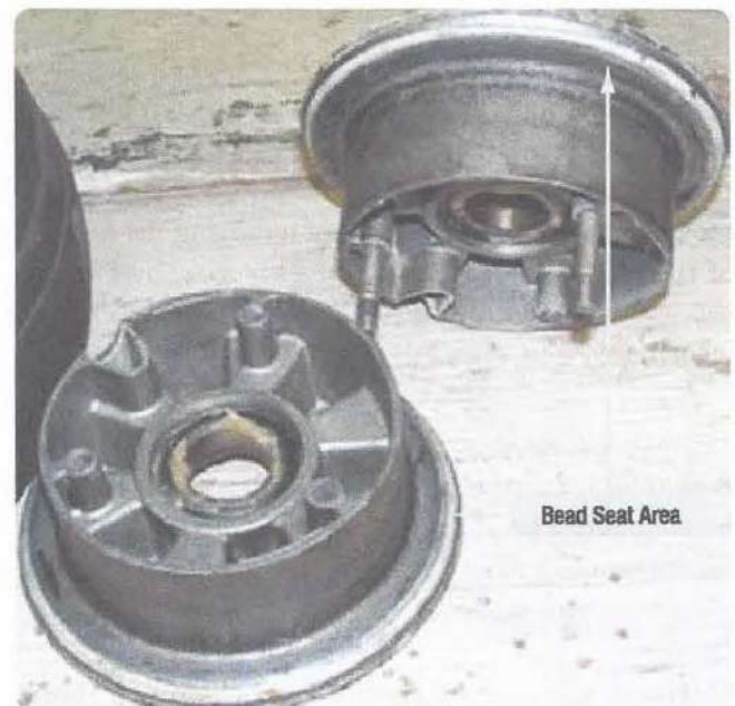
Figure 13-55. The bead seat areas of a light aircraft wheel set. Eddy current testing for cracks in the bead seat area is common.
