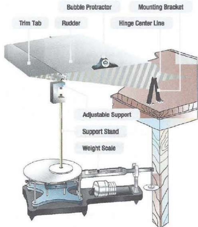
Figure 9-29. Scale measuring balance condition of control surface.
