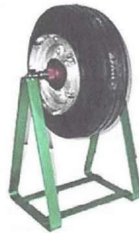
Figure 13-146. A typical aircraft tire and wheel balancing stand.
