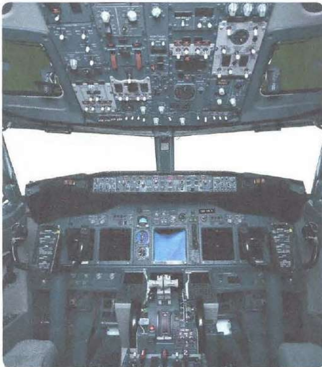
Figure 19-2. An instrument panel with fewer, integrated instruments.
