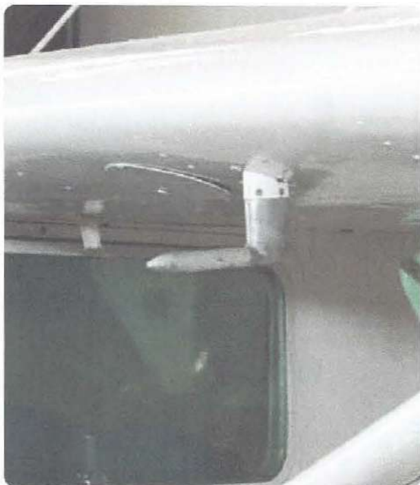
Figure 5-24. Pitot static system heads, or pitot tubes, can be of various designs and locations on airframes.
