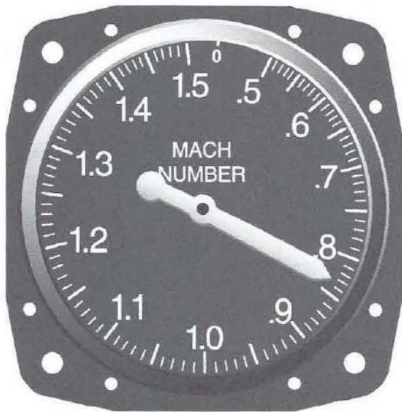
Figure 5-45. A Machmeter indicates aircraft speed relative to the speed of sound.
