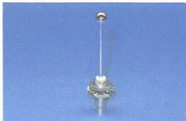
Figure 5-144. Aircraft radar beacon transponder antennas transmit and receive UHF and SHF radio waves.
