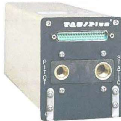
Figure 5-28. Teledyne's 90004 TAS/Plus air data computer (ADC) computes air data information from the pitot-static pneumatic system, aircraft temperature probe, and barometric correction device to help create a clear indication of flight conditions.
