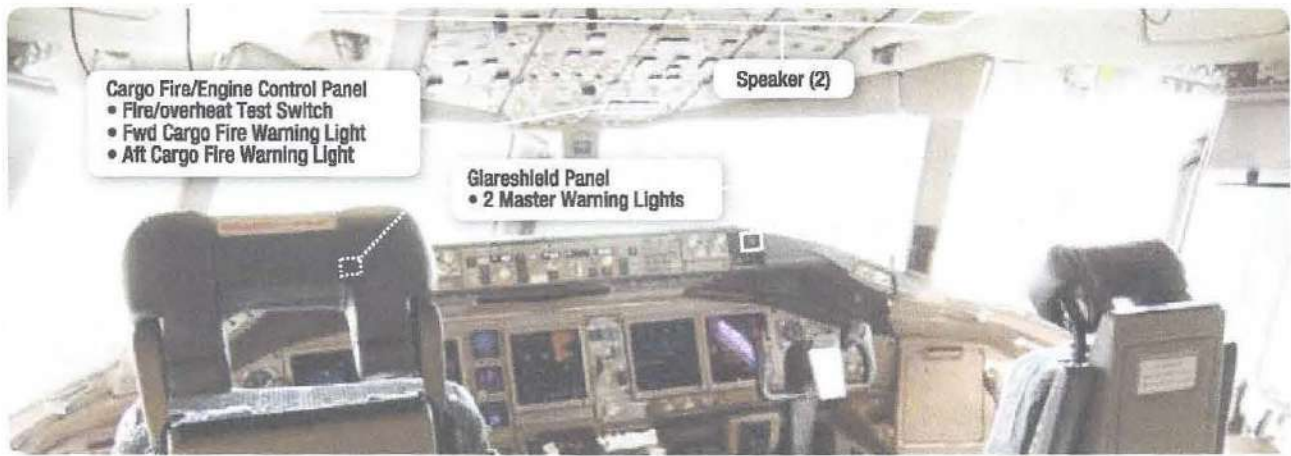
Figure 8-18. Cargo fire detection warning.
