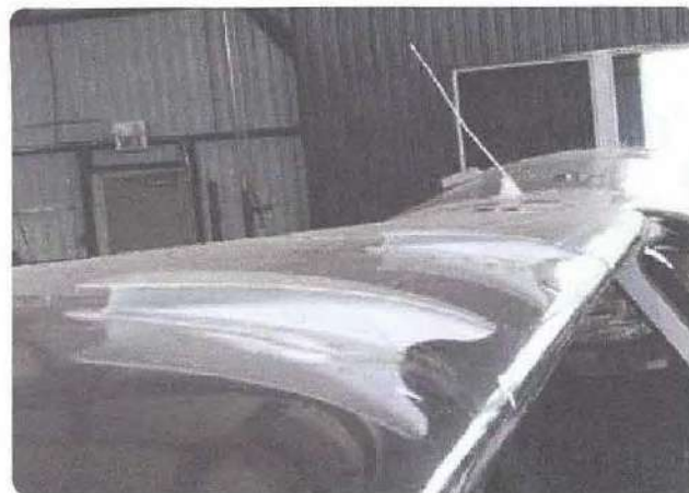
Figure 1-34. The Symphony SA-160 has two unique vortex generators on its wing to ensure aileron effectiveness through the stall.
