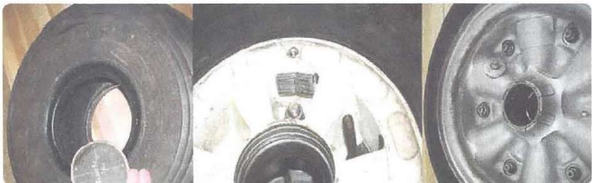
Figure 13-147. A tire balancing patch (left), adhesive wheel weights (center), and a bolted wheel weight (right) are all used to balance aircraft tire and wheel assemblies per the manufacturer's instructions.
