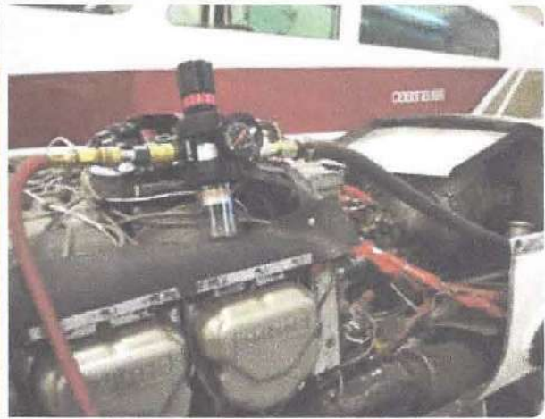
Figure 12-33. Test equipment used to test a wing de-ice system (left), and test equipment installed in the aircraft for testing (right).
