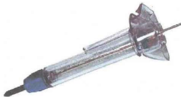
Figure 10-52. A sump drain tool used to open and collect fuel and contaminants from the fuel system sumps. Daily sump draining is part of the procedures needed to remove water from fuel that is to be delivered to the engine(s).
