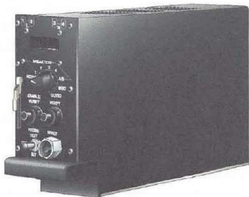
Figure 13-100. A rack mounted anti-skid control unit from an airliner.
