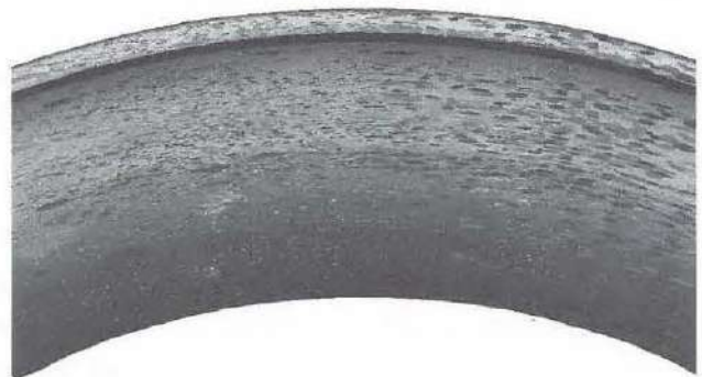
Figure 13-66. Bruising is caused by fine particle contamination possibly from a bad seal or improper maintenance of bearing cleanliness. It leaves a less than smooth surface on the bearing cup.
