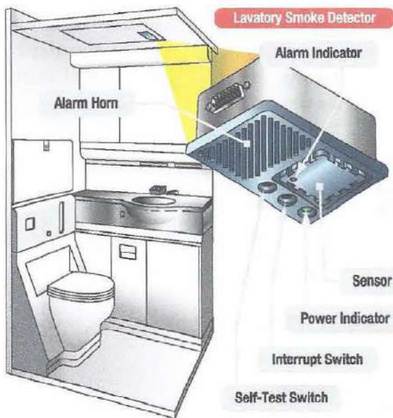
Figure 8-21. Lavatory smoke detector.
