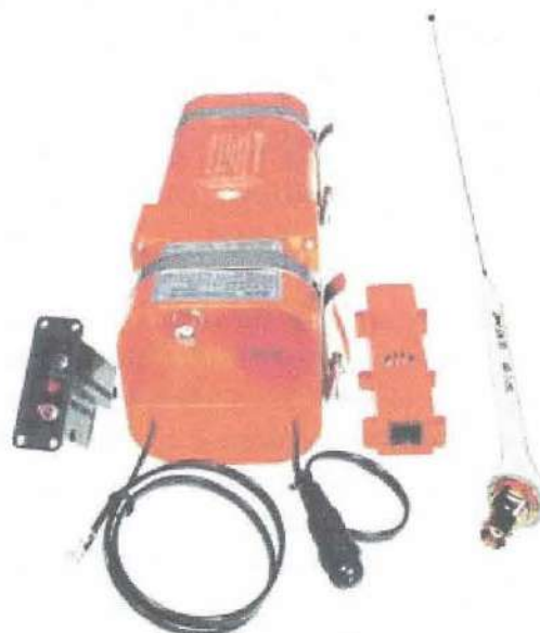
Figure 5-167. An ELT and its components including a cockpit-mounted panel, the ELT, a permanent mount antenna, and a portable antenna.
