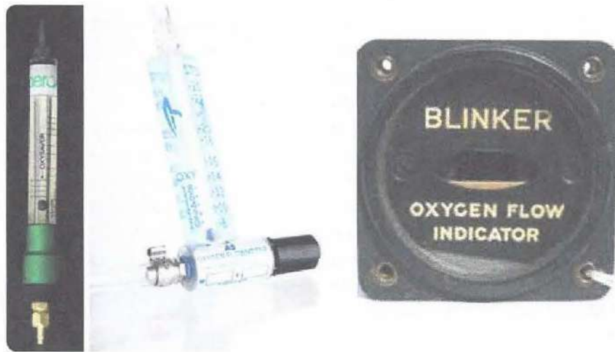
Figure 15-29. Different flow indicators are used to provide verification that the oxygen system is functioning: continuous-flow, in-line (left); continuous-flow, in-line with valve adjuster (center); and old style demand flow (right).
