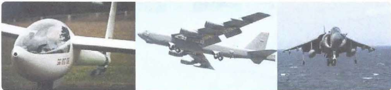
Figure 13-5. Tandem landing gear along the longitudinal axis of the aircraft permits the use of flexible wings on sailplanes (left) and select military aircraft like the B-52 (center). The VTOL Harrier (right) has tandem gear with outrigger type gear.
