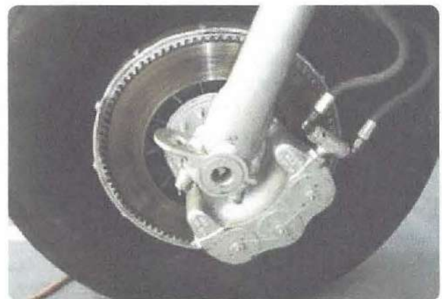
Figure 13-70. A single disc brake is a floating disc, fixed caliper brake.
