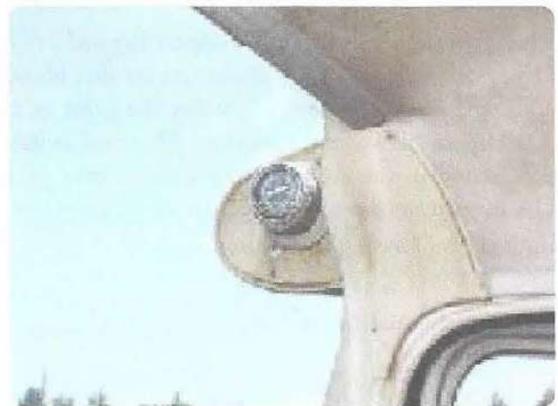
Figure 5-67. A bimetallic outside air temperature gauge and its installation on a light aircraft.
