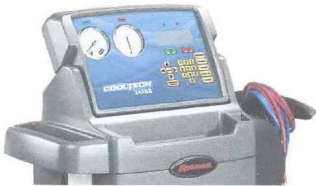
Figure 4-29. A modern refrigerant recovery/charge/recycle service unit. Electronic control of solenoid activated valves combine with a built-in system for recovering, recycling, and recharging. A built-in vacuum pump and heated refrigerant reservoir are also included.
