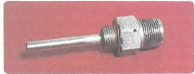
Figure 5-68. An electric resistance thermometer sensing bulb.
