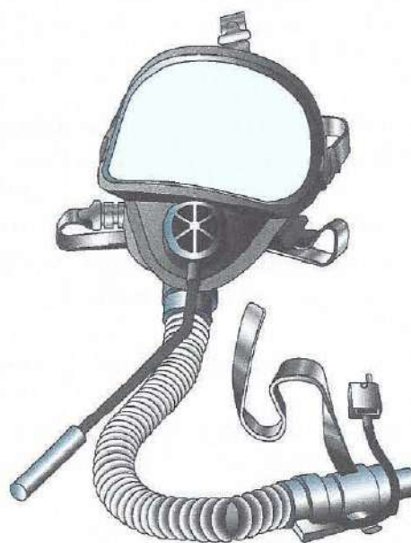
Figure 15-33. Smoke masks cover the eyes as well as the nose and mouth of the user.
