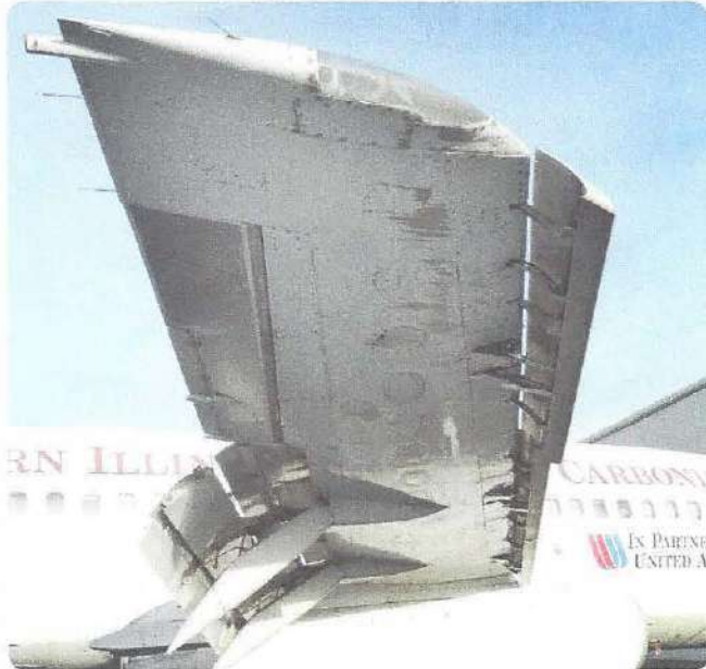
Figure 9-7. Outboard Trailing Edge Flaps and Slats Extended. Note how the extension of the flaps and slats increase the surface area of the wing in addition to altering the shape of the wing to enhance low-speed performance and lift production.
