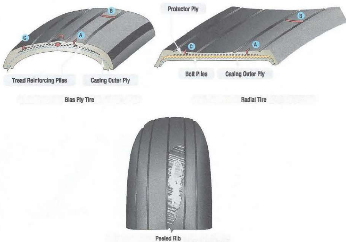
Figure 13-127. Remove an aircraft tire from service when the depth of a cut exposes the casing outer plies of a bias ply tire or the outer belt layer of a radial tire (A); a tread rib has been severed across the entire width (B); or, when undercutting occurs at the base of any cut (C). These conditions may lead to a peeled rib.
