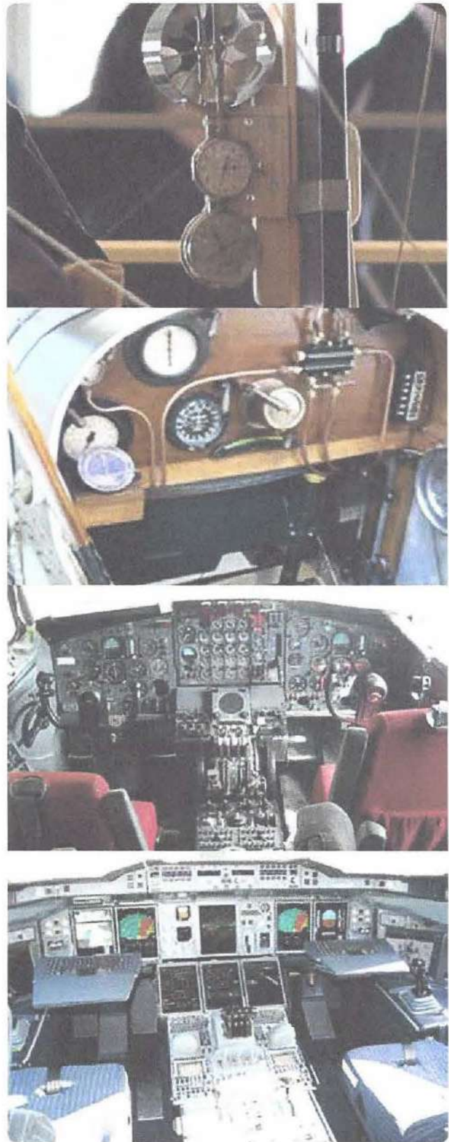
Figure 5-1. From top to bottom: instruments of the Wright Flyer, instruments on a World War I era aircraft, a late 1950s/early 1960s Boeing 707 airliner cockpit, and an Airbus A380 glass cockpit.
