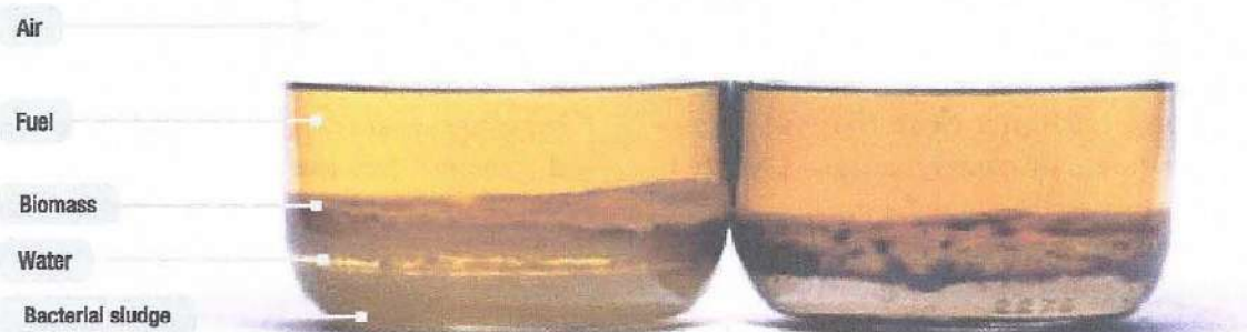
Figure 10-55. This fuel-water sample has microbial growth at the interface of the two liquids.
