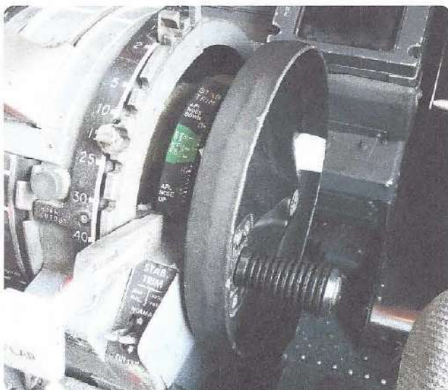
Figure 9-20. Mechanical Trim System and Trim Position Indicator for Horizontal Stabilizer. The protruding handle may be stowed within the trim wheel. The green band is used to signify the proper position of the horizontal stabilizer for takeoff. Trimming the horizontal stabilizer outside the green band provides an unsafe for takeoff warning scenario.
