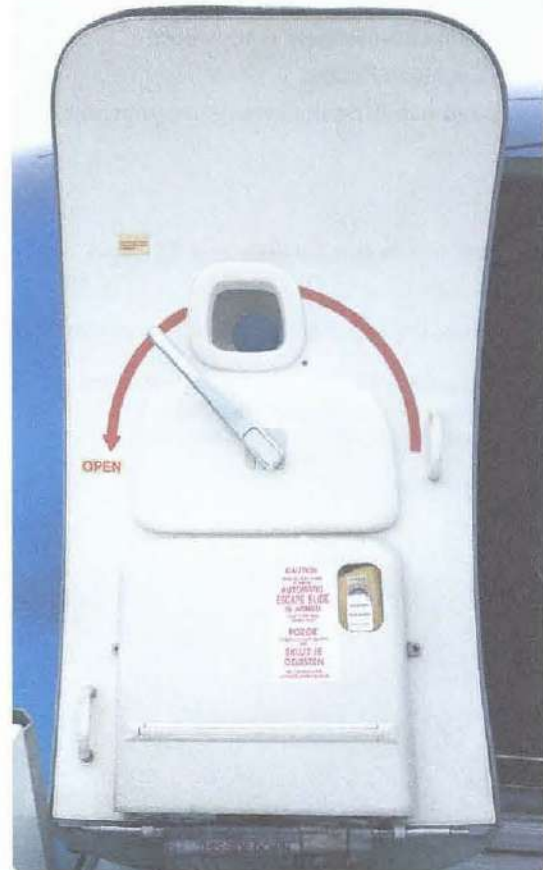
Figure 7-2. Emergency slide inflation canister pressure is checked regularly on the gauge in the lower window (mostly yellow). A life-limit removal date sticker partially obscures the gauge in the photo.
