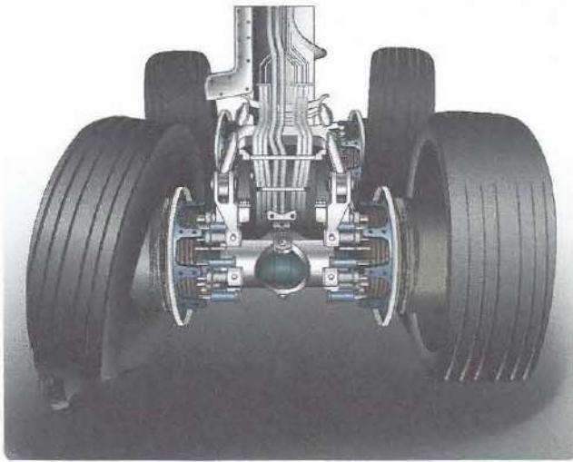
Figure 13-148. Heavy braking during an aborted takeoff caused these tires to fail.
