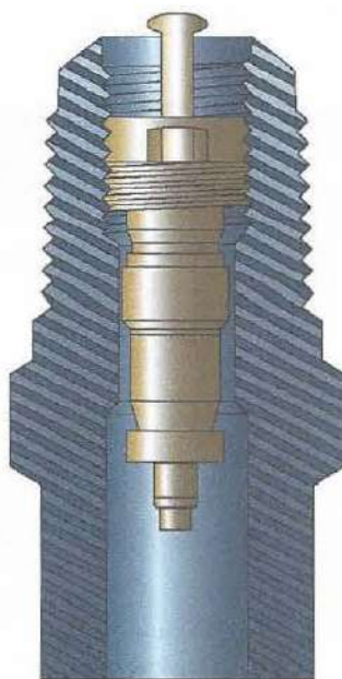
Figure 4-25. Cross-section of an R12 refrigerant service valve.
