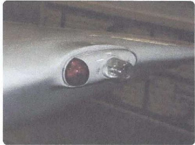
Figure 14-1. A left wing tip position light (red) and a white strobe light.
