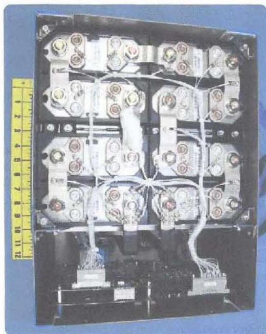
Figure 6-7. Cells and wiring in a lithium ion aircraft battery.
