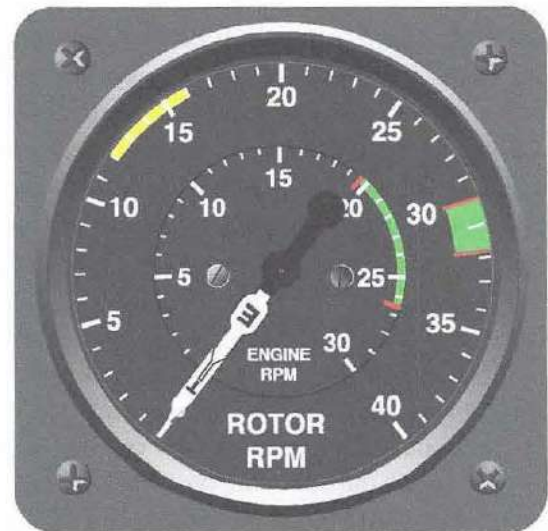
Figure 5-57. A helicopter tachometer with engine rpm, rotor rpm, and slippage indications.
