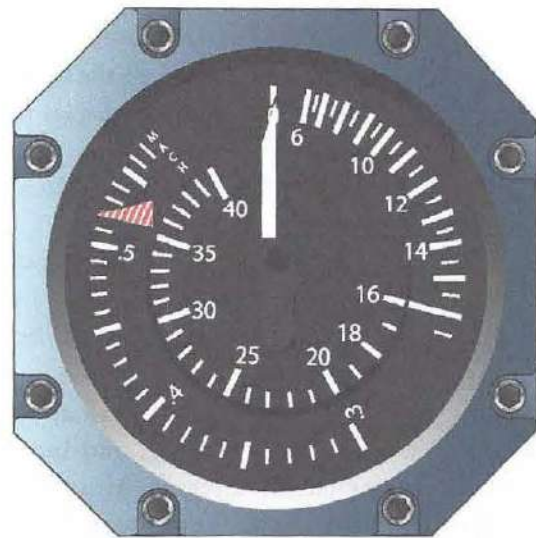
Figure 5-46. A combination Mach/airspeed indicator shows airspeed with a white pointer and Mach number with a red and white striped pointer. Each pointer is driven by separate internal mechanisms.
