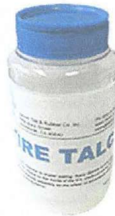
Figure 13-143. Tire talc is used on the inside of tube type tires and the outside of aircraft tubes. This prevents binding and allows the tube to expand without stress into place within the tire.
