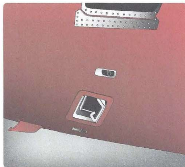
Figure 4-53. This outflow valve on a transport category aircraft is normally operated by an ac motor controlled by a pressure controller in the electronics equipment bay. A second ac motor on the valve is use when in standby mode. A DC motor also on the valve is used for manual operation.
