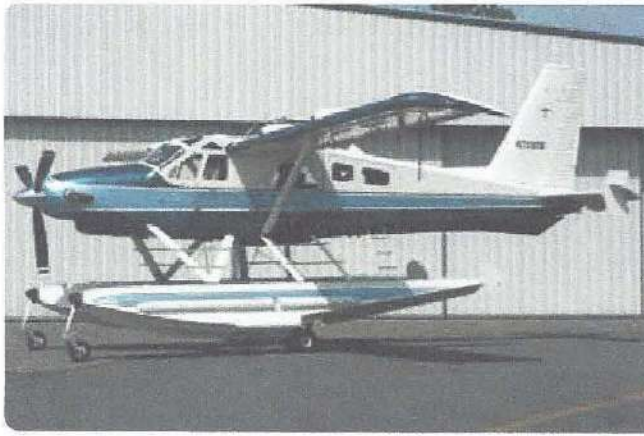
Figure 13-2. An amphibious aircraft with retractable wheels (left) and an aircraft with retractable skis (right).
