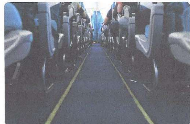
Figure 14-10. Emergency light strips in the aisle floor guide passengers and crew to the exits in case of emergency.
