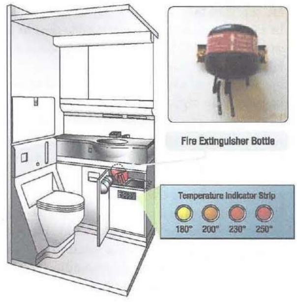
Figure 8-23. Lavatory fire extinguishing bottle.
