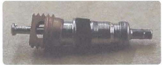
Figure 13-136. The tire valve core should be removed after the tire is completely deflated and before the tire and wheel assembly is removed from the aircraft.
