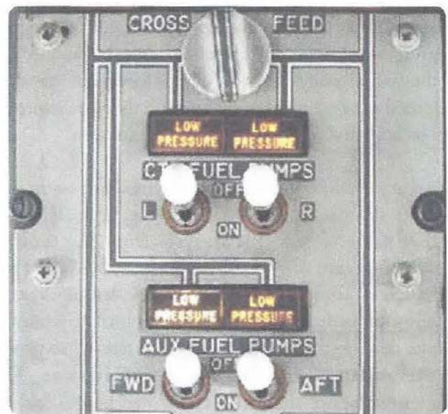
Figure 10-44. A transport category aircraft fuel panel with low pressure warning lights for each fuel boost pump.
