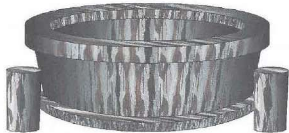
Figure 13-65. Etching and corrosion is caused when water, and the damage caused by water, penetrates the surface treatment of the bearing element. It appears as a reddish/brown discoloration.
