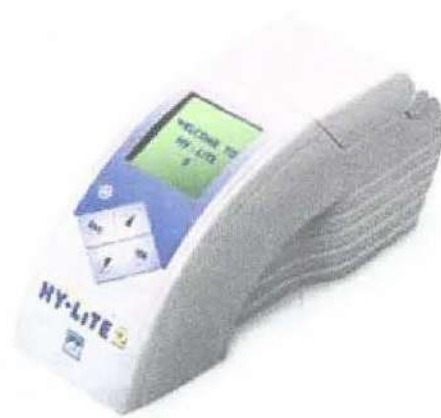
Figure 10-58. A capture solution is put into a 1 liter sample of fuel and shaken. The solution is then put into the analyzer shown to determine the level of microorganisms in the fuel.
