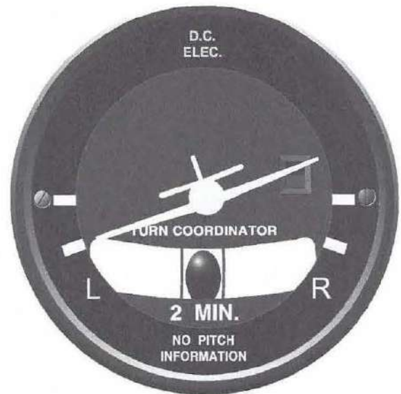
Figure 5-98. A turn coordinator senses and indicates the rate of both roll and yaw.
