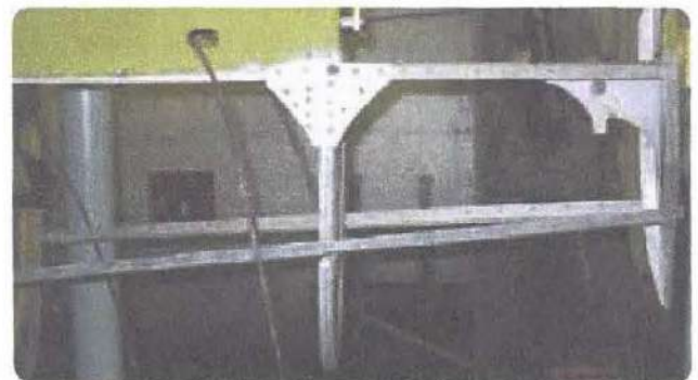
Figure 2-12. Gussets are used to increase strength.
