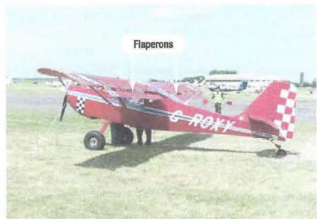
Figure 1-27. Flaperons on a Skystar Kitfox MK 7.
