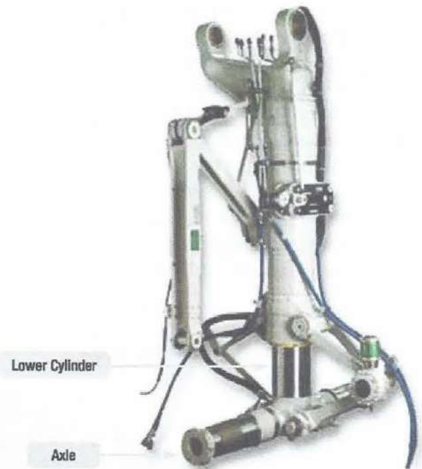
Figure 13-20. Axles machined out of the same material as the landing gear lower cylinder.
