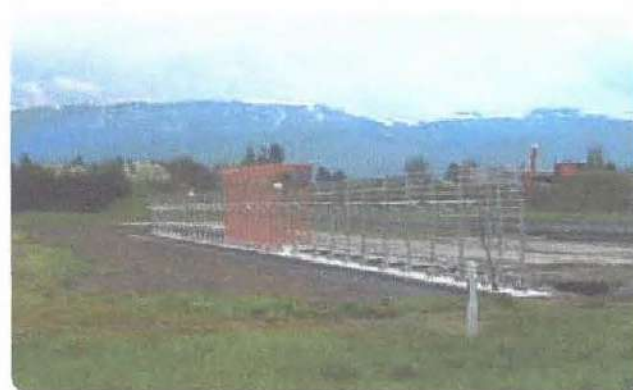
Figure 5-128. An ILS localizer antenna.
