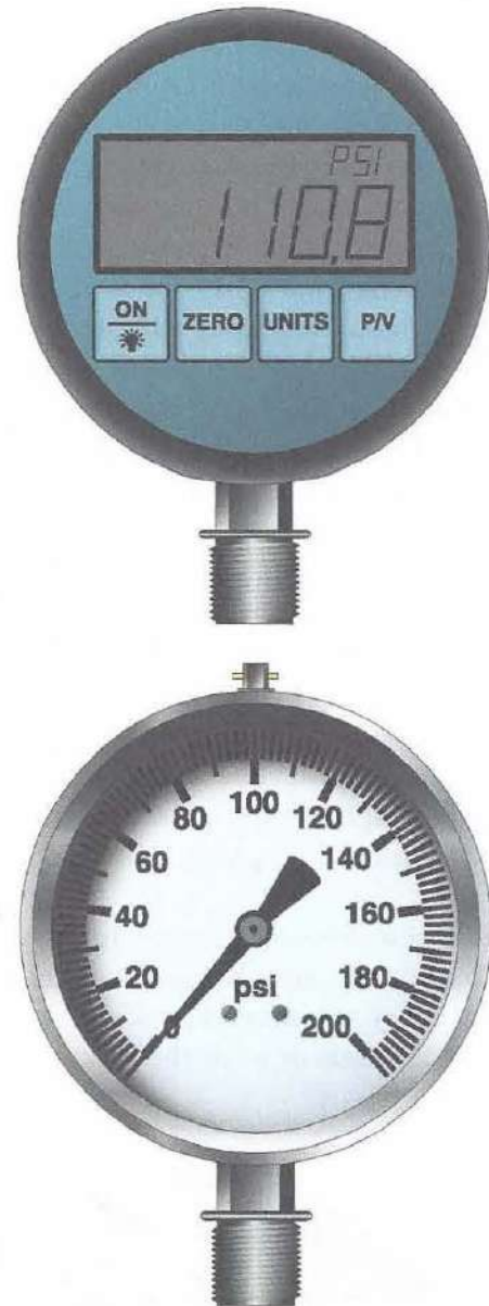
Figure 13-121. A calibrated bourdon tube dial type pressure gauge or a digital pressure gauge is recommended for checking tire pressure.
