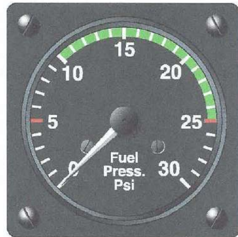
Figure 10-41. A typical fuel gauge that uses a signal from a sensing transducer to display fuel inlet pressure at the metering device.
