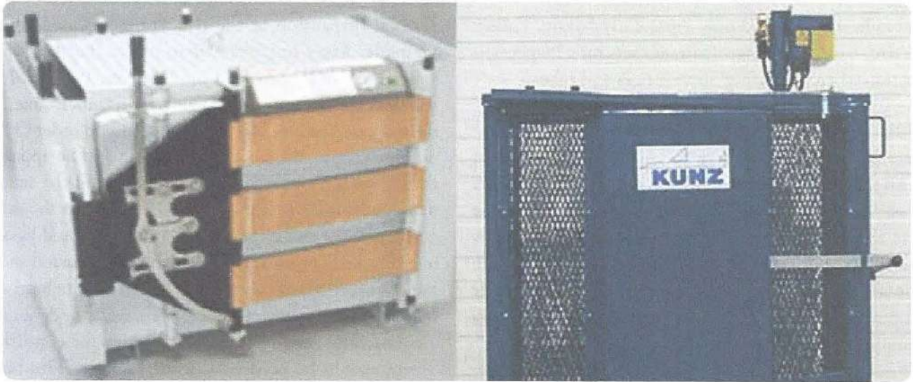
Figure 13-142. Modern tire inflation cages have been tested to withstand catastrophic failure of a tire and wheel assembly during inflation. All newly mounted tires should be inflated in such a cage.
