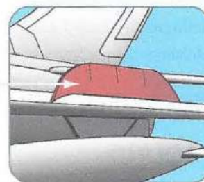
Figure 1-35. A stall fence aids in maintaining chordwise airflow over the wing.
