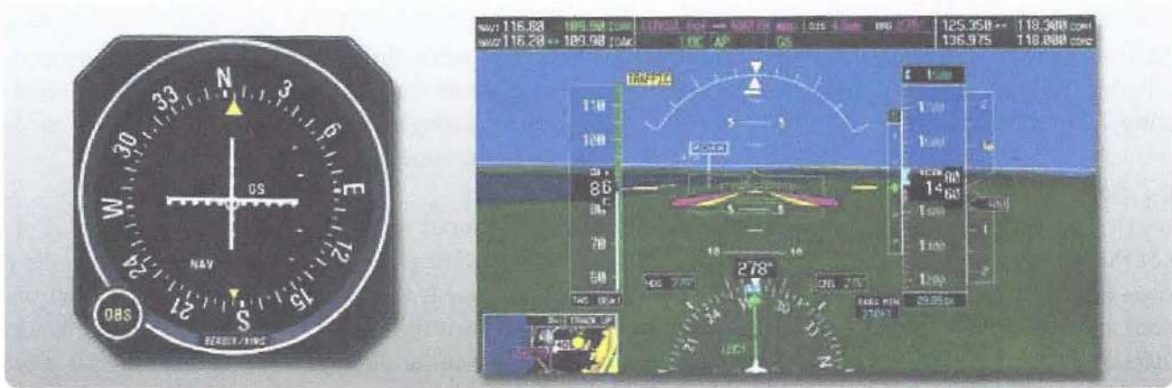
Figure 5-130. A traditional course deviation indicator is shown on the left. The horizontal white line is the deviation indicator for the glideslope. The vertical line is for the localizer. On the right, a Garmin G-1000 PFD illustrates an aircraft during an ILS approach. The narrow vertical scale on the right of the attitude indicator with the "G" at the top is the deviation scale for the glideslope. The green diamond moves up and down to reflect the aircraft being above or below the glidepath. The diamond is shown centered indicating the aircraft is on course vertically. The localizer CDI can be seen at the bottom center of the display. LOC1 is displayed to the left of it.
