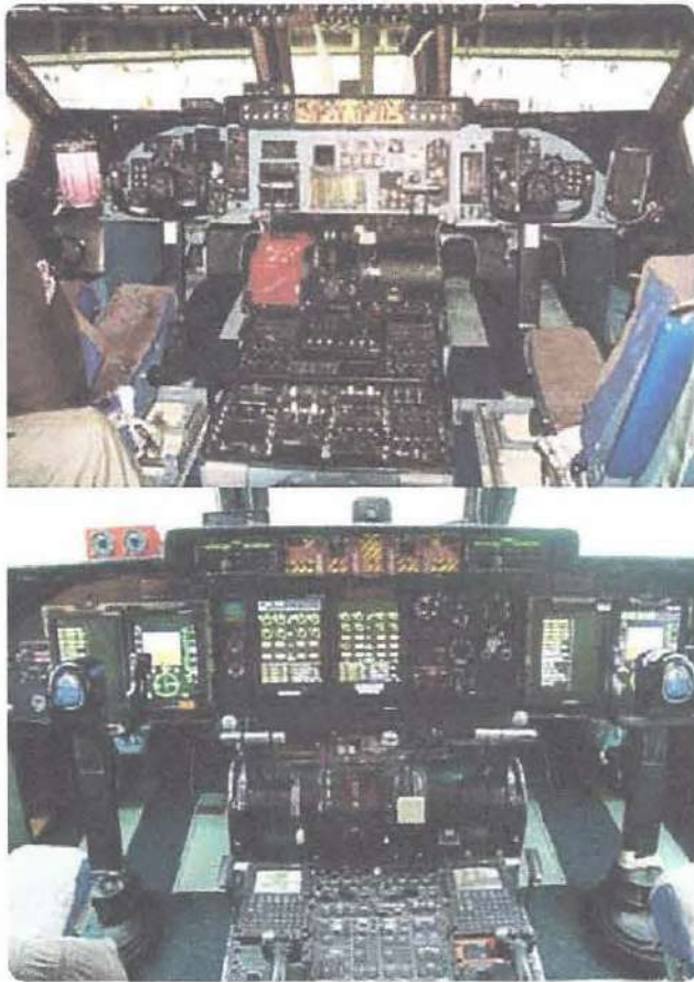
Figure 5-2. A conventional instrument panel of the C-5A Galaxy (top) and the glass cockpit of the C-5B Galaxy (bottom).
