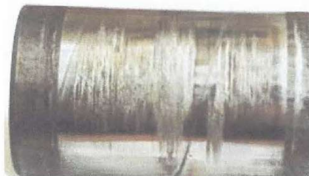
Figure 13-59. Galling is caused by rubbing of mating surfaces. The metal gets so hot it welds, and the surface metal is destroyed as the motion continues and pulls the metal apart in the direction of motion.
