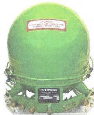
Figure 15-8. A spherical liquid oxygen on-board container used by the military.
