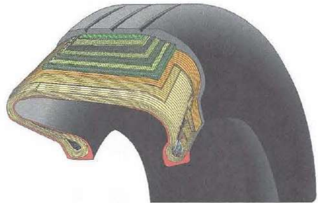
Figure 13-117. A radial tire has the fiber strands of the ply fabric oriented with and at 90 degrees to the direction of rotation and the tire sidewall. This restricts flexibility directionally and the flexibility of the sidewall while it strengthens the tire to carry heavy loads.
