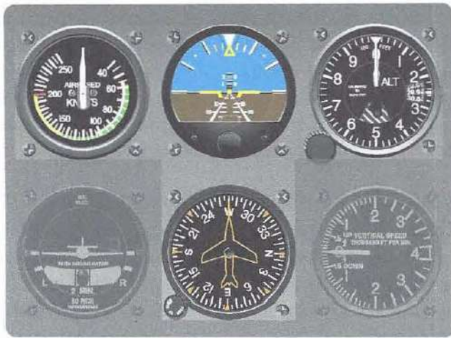
Figure 5-4. The basic T arrangement of analog flight instruments. At the bottom of the T is a heading indicator that functions as a compass but is driven by a gyroscope and not subject to the oscillations common to magnetic direction indicators.
