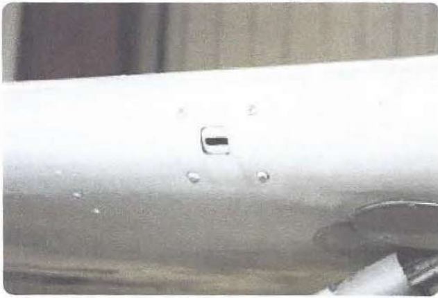
Figure 5-61. A reed type stall warning device is located behind this opening in the leading edge of the wing. When the angle of attack increases to near the point of a stall, low-pressure air flowing over the opening causes a suction, which audibly vibrates the reed.
