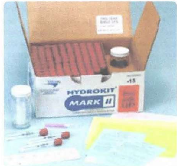
Figure 10-57. This kit allows periodic testing for water in fuel.
