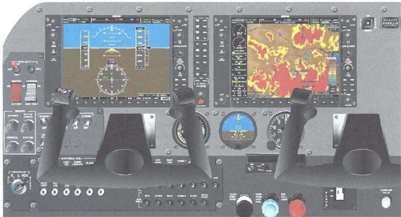
Figure 5-93. Instrumentation displayed within a glass cockpit using an attitude heading and reference system (AHRS) computer.
