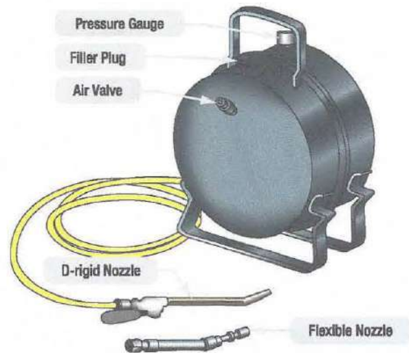
Figure 13-108. A typical brake bleeder pot or tank contains pure brake fluid under pressure. It pushes the fluid through the brake system to displace any air that may be present.
