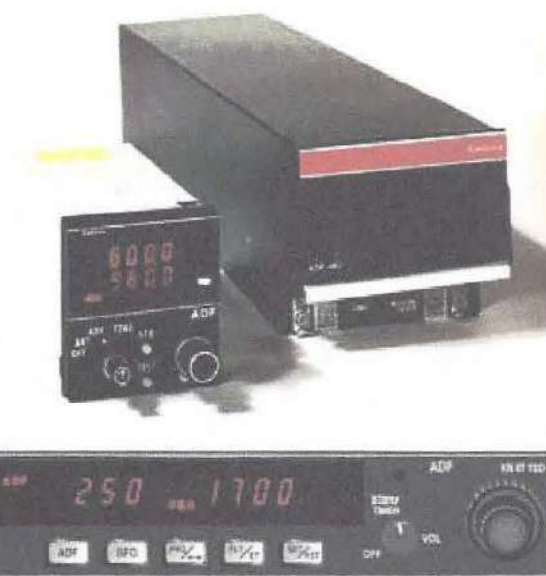
Figure 5-124. A cockpit mountable ADF receiver used on general aviation aircraft.
