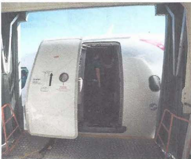
Figure 3-5. A plug type cabin entry door.
