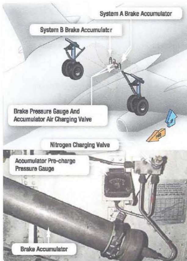
Figure 13-93. Emergency brake hydraulic fluid accumulators are precharged with nitrogen to deliver brake fluid to the brakes in the event normal and alternate hydraulic sources fail.
