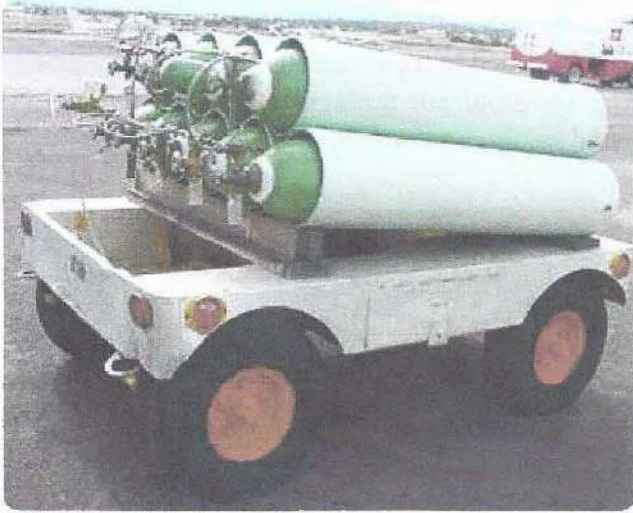
Figure 15-9. Typical oxygen servicing cart used to fill an aircraft system.
