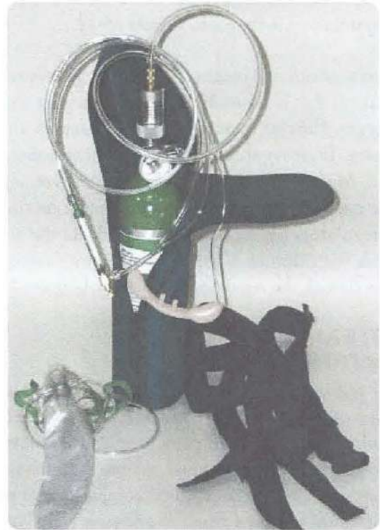
Figure 15-11. A typical portable gaseous oxygen cylinder complete with valve, pressure gauge, regulator/reducer, hose, adjustable flow indicator, and rebreather cannula. A padded carrying case/bag can be strapped to the back of a seat in the cabin to meet certification and testing specifications.
