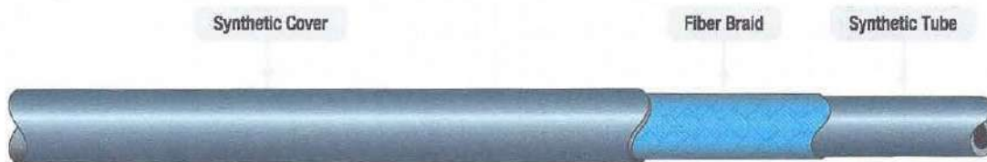
Figure 10-13. A typical flexible aircraft fuel line with braided reinforcement.
