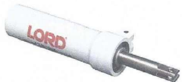
Figure 13-43. A non-hydraulic shimmy damper uses a rubber piston with lubricant that dampens via motion against the inner diameter of the unit housing.
