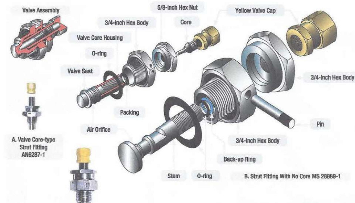
Figure 13-26. Valve core type (A) and core-free valve fittings (B) are used to service landing gear shock struts.
