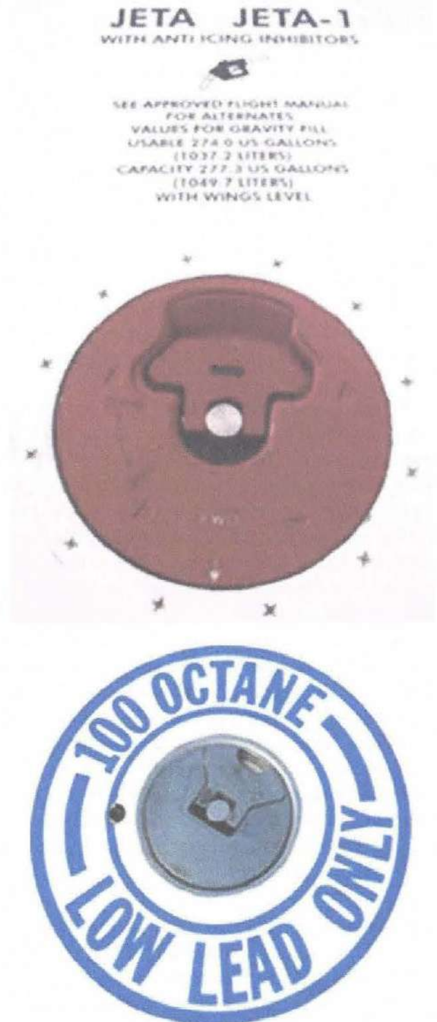
Figure 10-56. All entry points of fuel into the aircraft are marked with the type of fuel to be used. Never introduce any other fuel into the aircraft other than that which is specified.
