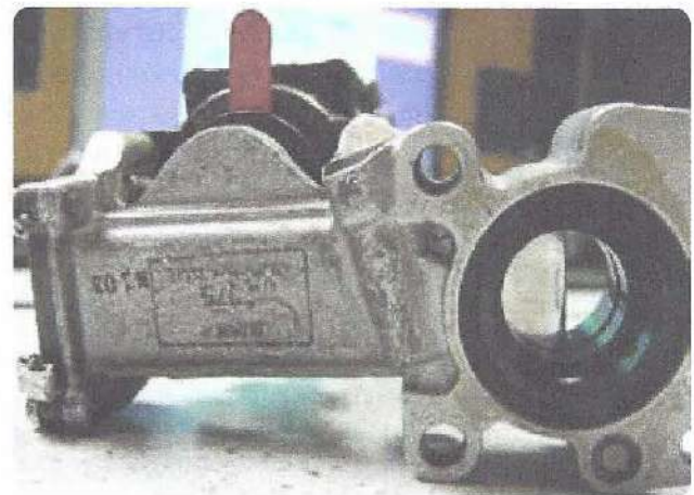
Figure 10-18. This motor operated gate valve has a red position indicating lever that can be used by maintenance personnel to identify the position of the valve. The lever can be moved by the technician to position the valve.
