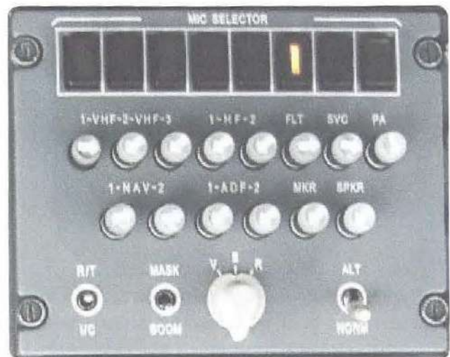
Figure 5-111. A typical airliner audio control panel.
