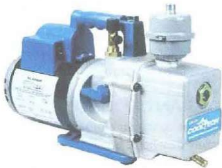
Figure 4-32. A vacuum pump is used to lower the pressure in the vapor cycle air conditioning system. This reduces the boiling point of water in the system, which vaporizes and is drawn out by the pump.
