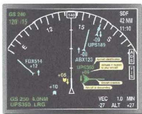
Figure 5-154. A cockpit display of ADS-B generated targets (left) and an ADS-B airborne receiver with antenna (right).
