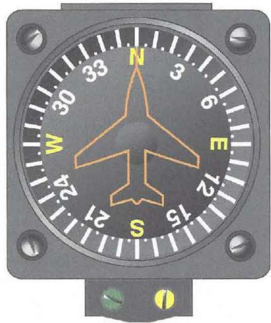
Figure 5-81. A vertical magnetic direction indicator provides a realistic reference of headings.
