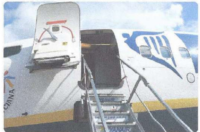
Figure 7-9. Airstairs on an airliner stow under the main cabin floor.
