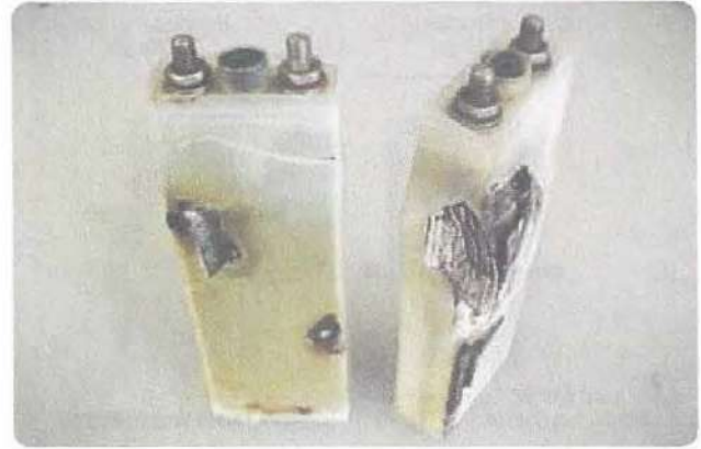
Figure 6-6. Thermal runaway damage.
