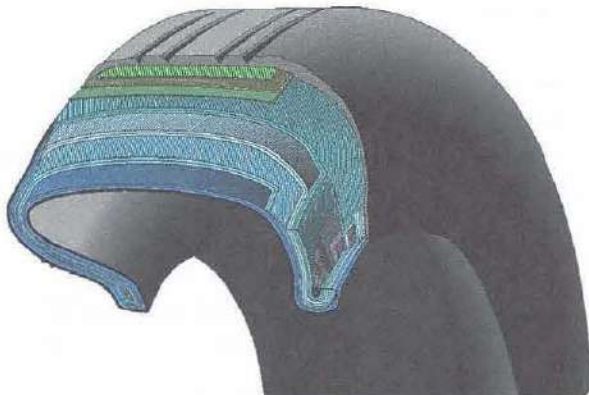
Figure 13-116. A bias ply tire has the fabric bias oriented with and across the direction of rotation and the sidewall. Since fabric can stretch on the bias, the tire is flexible, and can absorb loads. Strength is obtained by adding plies.
