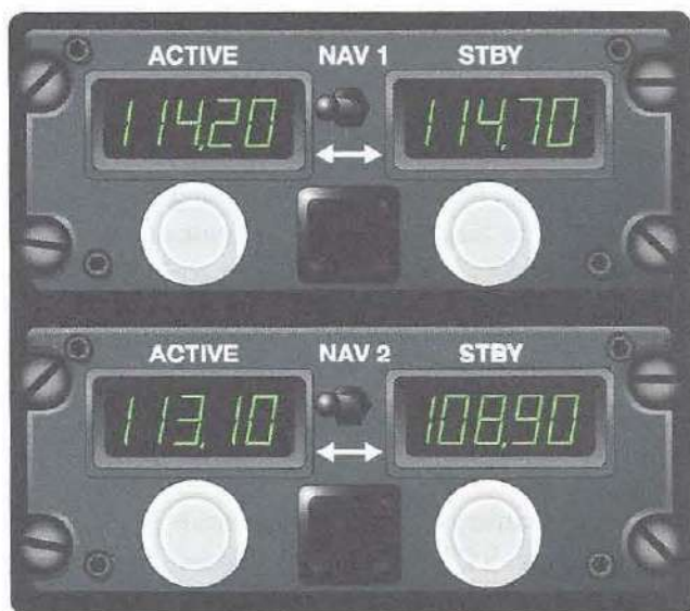
Figure 5-117. An airliner VOR control head with two independent NAV receivers each with an active and standby tuning circuit controlled by a toggle switch.
