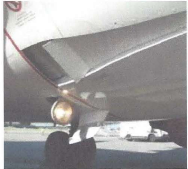
Figure 4-9. A ram air door controls the flow of air through the primary and secondary heat exchangers.
