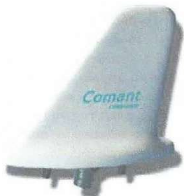
Figure 5-144. Aircraft radar beacon transponder antennas transmit and receive UHF and SHF radio waves.
