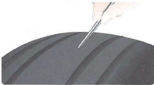
Figure 13-126. Deflate a tire before removing or probing any area where a foreign object is lodged.
