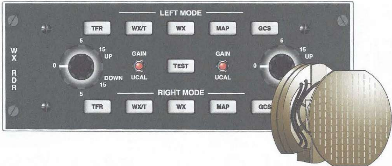
Figure 5-160. A typical on-board weather radar system for a high performance aircraft uses a nose-mounted antenna that gimbals. It is usually controlled by the inertial reference system (IRS) to automatically adjust for attitude changes during maneuvers so that the radar remains aimed at the desired weather target. The pilot may also adjust the angle and sweep manually as well as the gain. A dual mode control panel allows separate control and display on the left or right HSI or navigational display.
