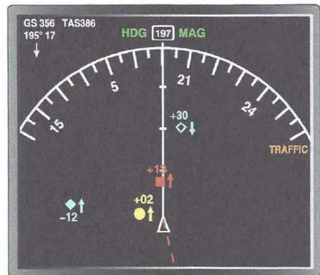
Figure 5-150. TCAS information displayed on a multifunction display. An open diamond indicates a target; a solid diamond represents a target that is within 6 nautical miles of 1 200 feet vertically. A yellow circle represents a target that generates a TA (25-48 seconds before contact). A red square indicates a target that generates an RA in TCAS II (contact within 35 seconds). A (+) indicates the target aircraft is above and a (-) indicates it is below. The arrows show if the target is climbing or descending.
