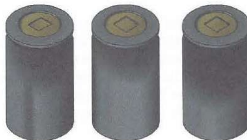
Figure 13-61. Overheating caused by lack of sufficient lubrication results in a bluish tint to the metal surface. The ends of the rollers shown were overheated causing the metal to flow and deform, as well as discolor. The bearing cup raceway is usually discolored as well.
