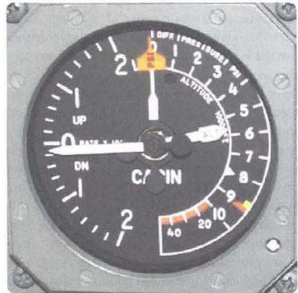
Figure 4-55. This cabin pressurization gauge is a triple combination gauge. The long pointer operates identically to a vertical speed indicator with the same familiar scale on the left side of the gauge. It indicates the rate of change of cabin pressure. The orange PSI pointer indicates the differential pressure on the right side scale. The ALT indicator uses the same scale as the PSI pointer, but it indicates cabin altitude when ALT indicator moves against it.
