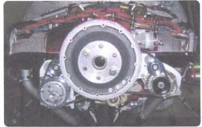
Figure 4-22. A typical belt drive engine driven compressor. The electromagnetic clutch pulley assembly in the front starts and stops the compressor depending on cooling demand.
