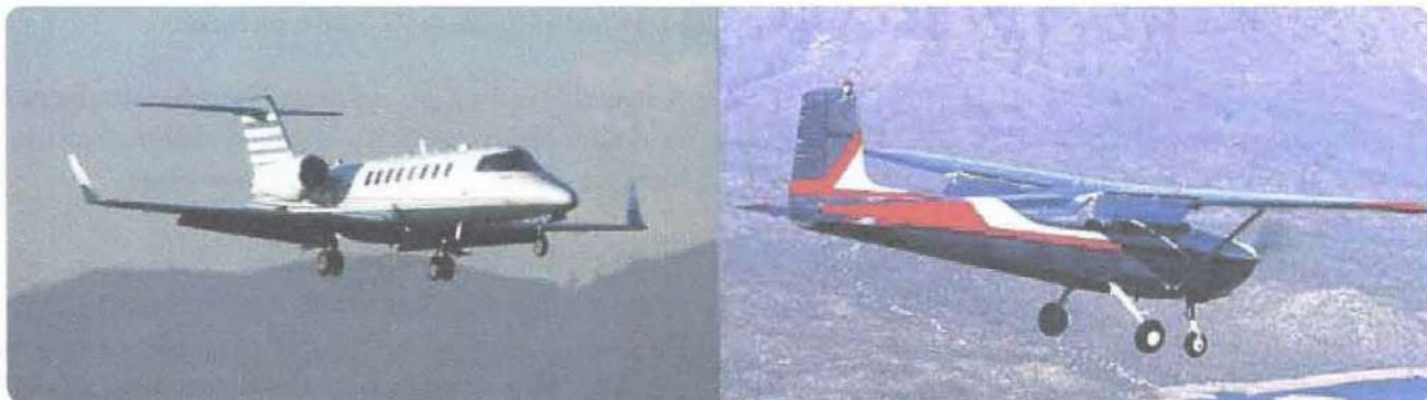
Figure 13-6. Tricycle type landing gear with dual main wheels on a Learjet (left) and a Cessna 172, also with tricycle gear (right).
