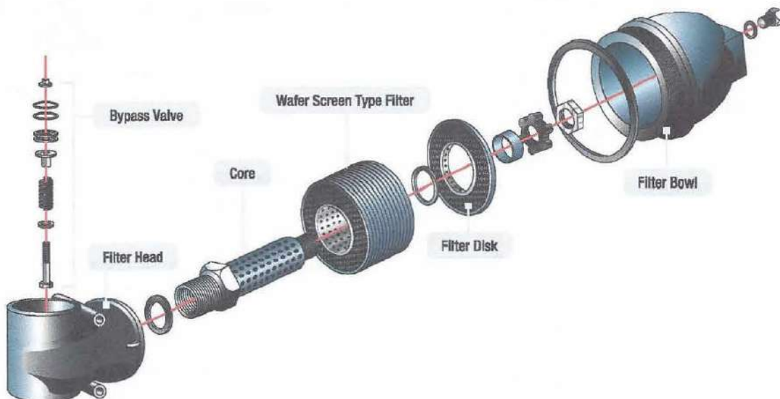
Figure 10-28. A micron wafer filter uses multiple screen wafers through which fuel must pass to exit the filter through the core. A spring loaded bypass valve in the filter housing unseats when the filter is clogged to continue delivery of fuel.
