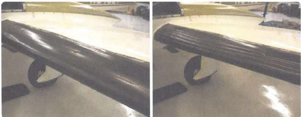
Figure 12-26. De-icing boots inflated (left) and deflated (right).
