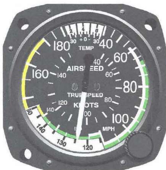
Figure 5-43. An analog true airspeed indicator. The pilot manually aligns the outside air temperature with the pressure altitude scale, resulting in an indication of true airspeed.
