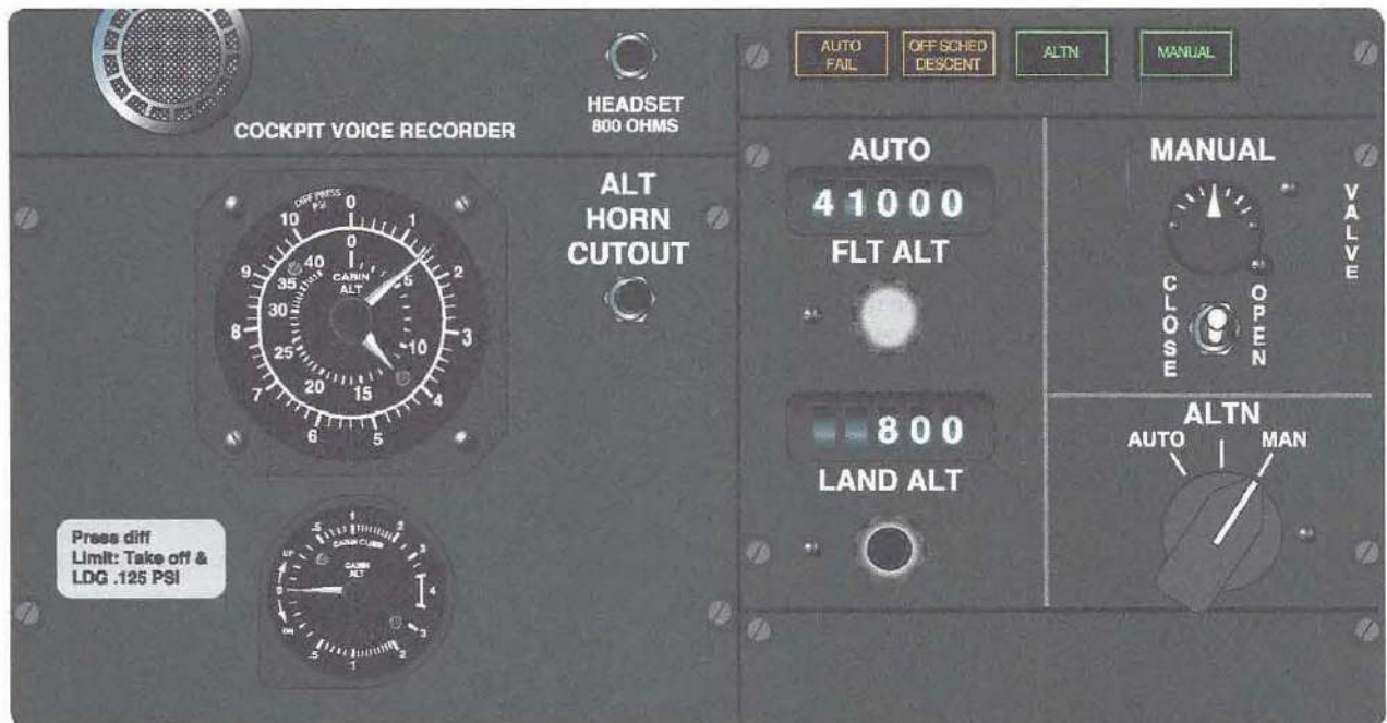
Figure 4-51. This pressurization panel from an 800 series Boeing 737 has input selections of flight altitude and landing altitude.
