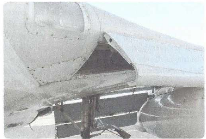
Figure 9-8. Leading edge and trailing edge inboard flaps extended. In addition to the outboard trailing edge flaps and slats shown in the previous illustration, leading edge flaps and inboard trailing edge flaps, seen behind the landing gear, are extended to further enhance low-speed performance.
