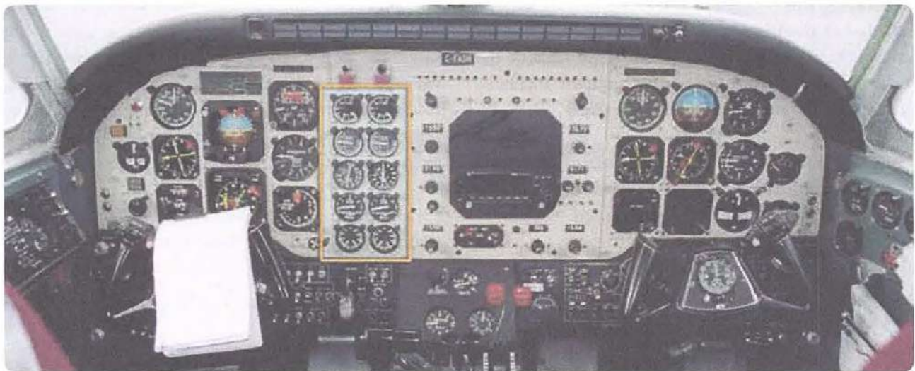
Figure 5-7. An engine instrumentation located in the middle of the instrument panel is shared by the pilot and co-pilot.
