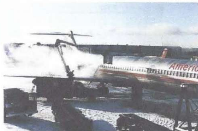
Figure 12-39. Boom truck de-icing of an airliner.
