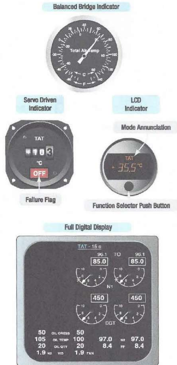
Figure 5-76. Different cockpit TAT displays.
