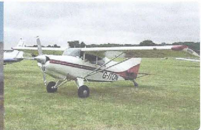
Figure 13-3. Tail wheel configuration landing gear on a DC-3 (left) and a STOL Maule MX-7-235 Super Rocket.
