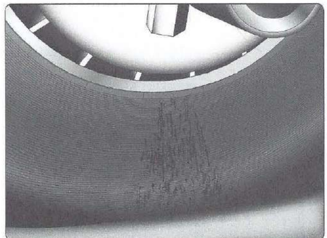
Figure 13-134. Cracking and checking in the sidewall of a tire is acceptable for service as long as it does not extend to or expose the sidewall carcass plies.
