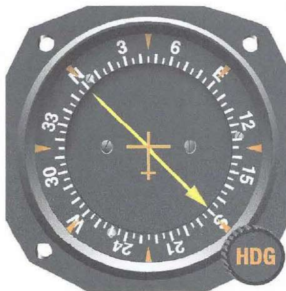
Figure 5-121. A movable card ADF indicator can be rotated to put the aircraft's heading at the top of the scale. The pointer then points to the magnetic bearing the ADF broadcast antenna.
