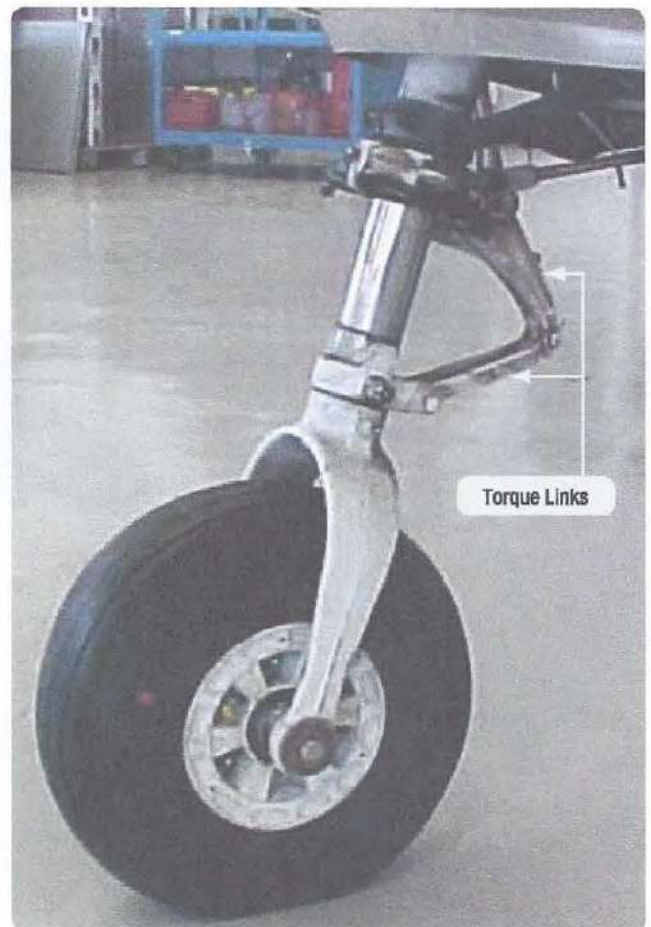
Figure 13-21. Torque links align the landing gear and retain the piston in the upper cylinder when the strut is extended.
