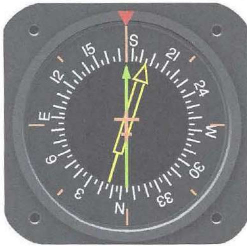
Figure 5-85. A radio magnetic indicator (RMI) combines a slaved gyro heading indication (red triangle at top of gauge) with magnetic bearing information to a VOR station (solid pointer) and an ADF station (hollow pointer).
