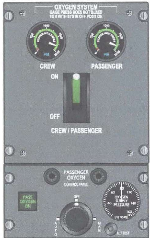
Figure 15-16. The crew can deploy passenger emergency continuous-flow oxygen masks and supply with a switch in the cockpit.
