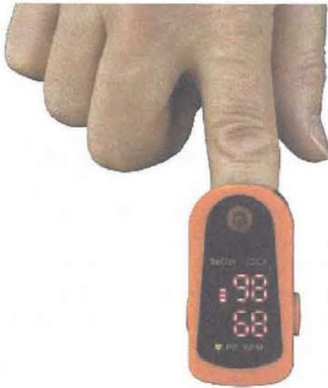
Figure 15-31. A portable pulse type oximeter displays percentage of oxygen saturation of the blood and heart rate. Pilots can adjust oxygen supply levels to maintain saturation and avoid hypoxia.
