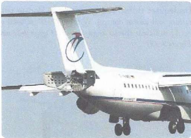
Figure 9-10. Speed brake using the tail cone.
