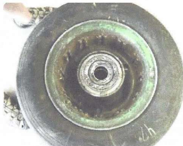
Figure 13-51. Keys on the inner wheel half of an aircraft wheel used to engage and rotate the rotors of a disc brake.
