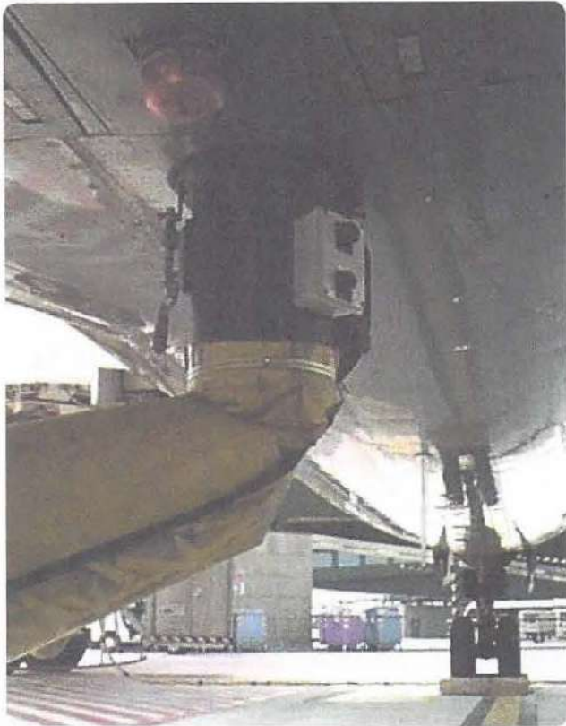
Figure 4-4. A duct hose installed on this airliner distributes hot or cold air from a ground-based source throughout the cabin using the aircraft's own air distribution system ducting.
