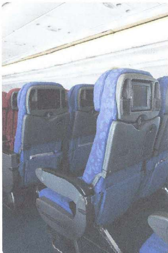
Figure 7-3. Passenger seats are locked into a seat track on the floor of the cabin.
