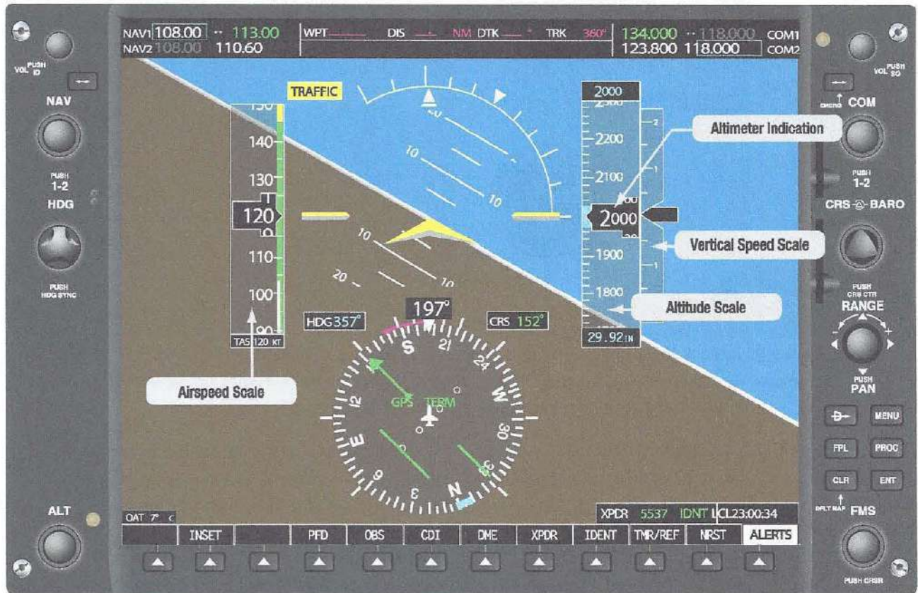
Figure 5-34. This primary flight display unit of a Garmin 1000 series glass cockpit instrumentation package for light aircraft indicates altitude using a vertical linear scale and a numerical counter. As the aircraft climbs or descends, the scale behind the black numerical altitude readout changes.
