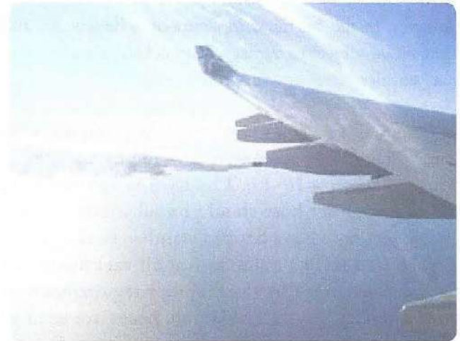
Figure 10-12. Fuel being jettisoned free of the airframe on a transport category aircraft.
