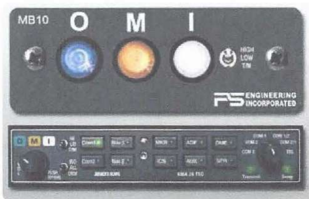
Figure 5-134. Various marker beacon instrument panel display lights.
