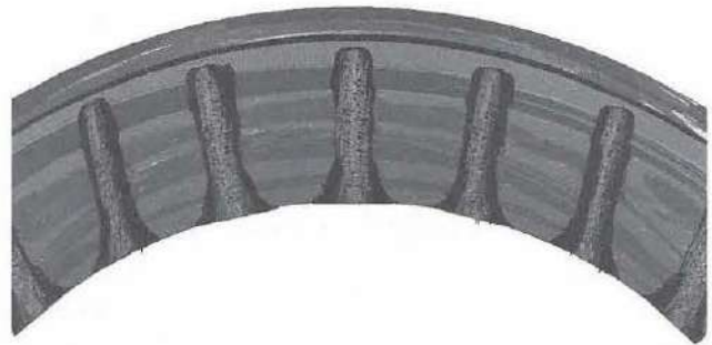
Figure 13-64. Staining and surface marks on the bearing cup that are grayish black streaks with the same spacing as the rollers are caused by water that has gotten into the bearing. It is the first stage of deeper corrosion that will follow.
