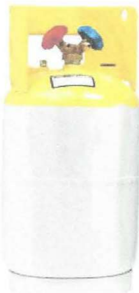
Figure 4-30. A 30 pound R134a refrigerant container with dual fittings. The fitting controlled by the blue valve wheel opens to the vapor space above the liquid refrigerant for connection to the low side of the vaporcycle system. The fitting controlled by the red valve wheel draws liquid refrigerant from the bottom of the cylinder through a stand tube. This fitting is connected to the system high side. On containers without dual fittings, the container must be inverted to deliver liquid refrigerant through a connected hose.
