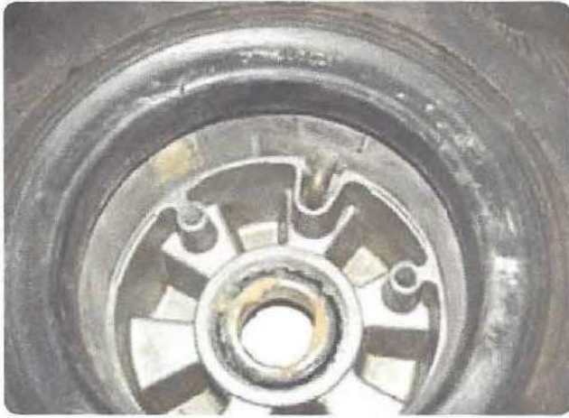
Figure 13-145. Mounting a tube type tire with the tube valve stem positioned to pass through the outboard wheel half.
