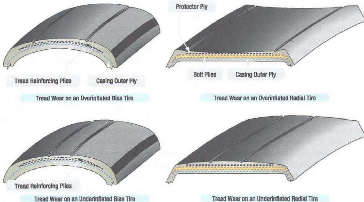
Figure 13-122. Tires that are overinflated lack adherence to the runway and develop excess tread wear in the center of the tread. Tires that are under inflated develop excess tread wear on the tire shoulders. Overheating resulting in internal carcass damage and potential failure are possible from flexing the tire beyond design limits.
