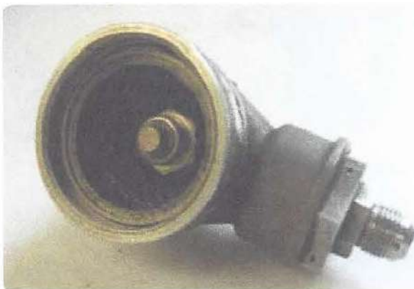
Figure 8-13. Discharge valve (left) and cartridge, or squib (right).
