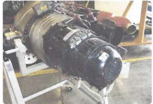
Figure 6-14. Large aircraft AC alternator.
