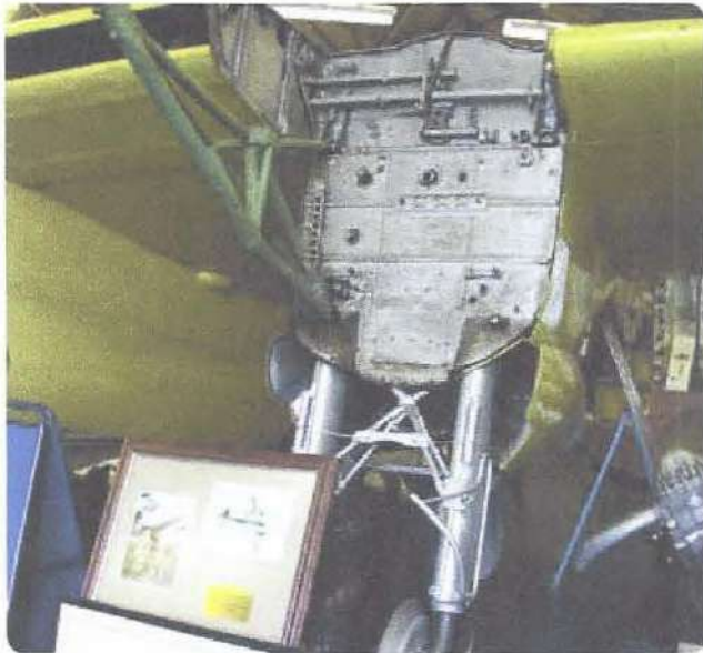
Figure 3-28. An engine nacelle firewall.
