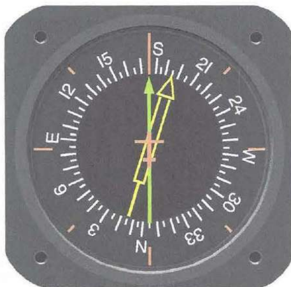
Figure 5-126. A radio magnetic indicator (RMI) combines a magnetic compass, VOR, and ADF indications.
