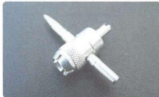
Figure 13-29. This valve tool features internal and external thread chasers, a notched valve core removal/installation tool, and a tapered end for depressing a valve core or clearing debris.
