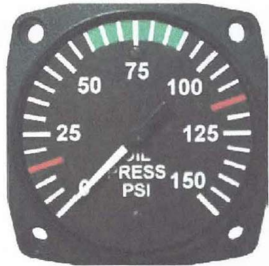
Figure 5-13. An analog oil pressure gauge is driven by a Bourdon tube. Oil pressure is vital to engine health and must be monitored by the pilot.
