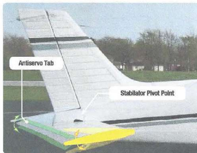
Figure 1-18. An Anti-servo tab moves in the same direction as the control tab. Shown here on a stabilator, it desensitizes the pitch control.
