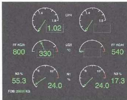
B. A digital EPR indication and other turbine engine parameters on a cockpit digital display screen.
