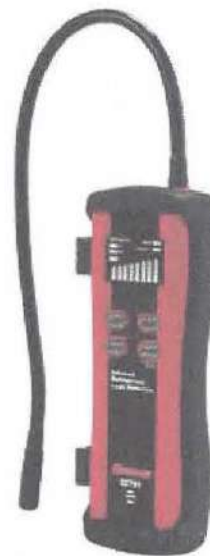
Figure 4-33. This electronic infrared leak detector can detect leaks that would lose less than ¼ ounce of refrigerant per year.
