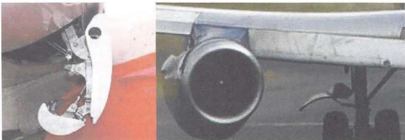
Figure 1-26. Side view (left) and front view (right) of a Krueger flap on a Boeing 737.
