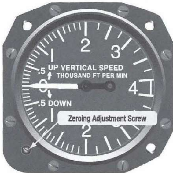
Figure 5-38. A typical vertical speed indicator.
