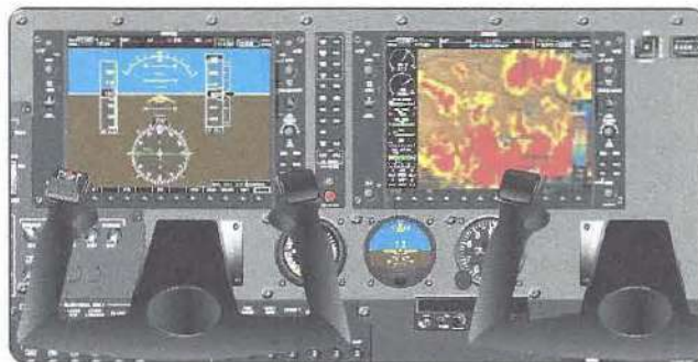
Figure 5-5. This electrically operated flat screen display instrument panel, or glass cockpit, retains an analog airspeed indicator, a gyroscope-driven artificial horizon, and an analog altimeter as a backup should electric power be lost, or a display unit fails.
