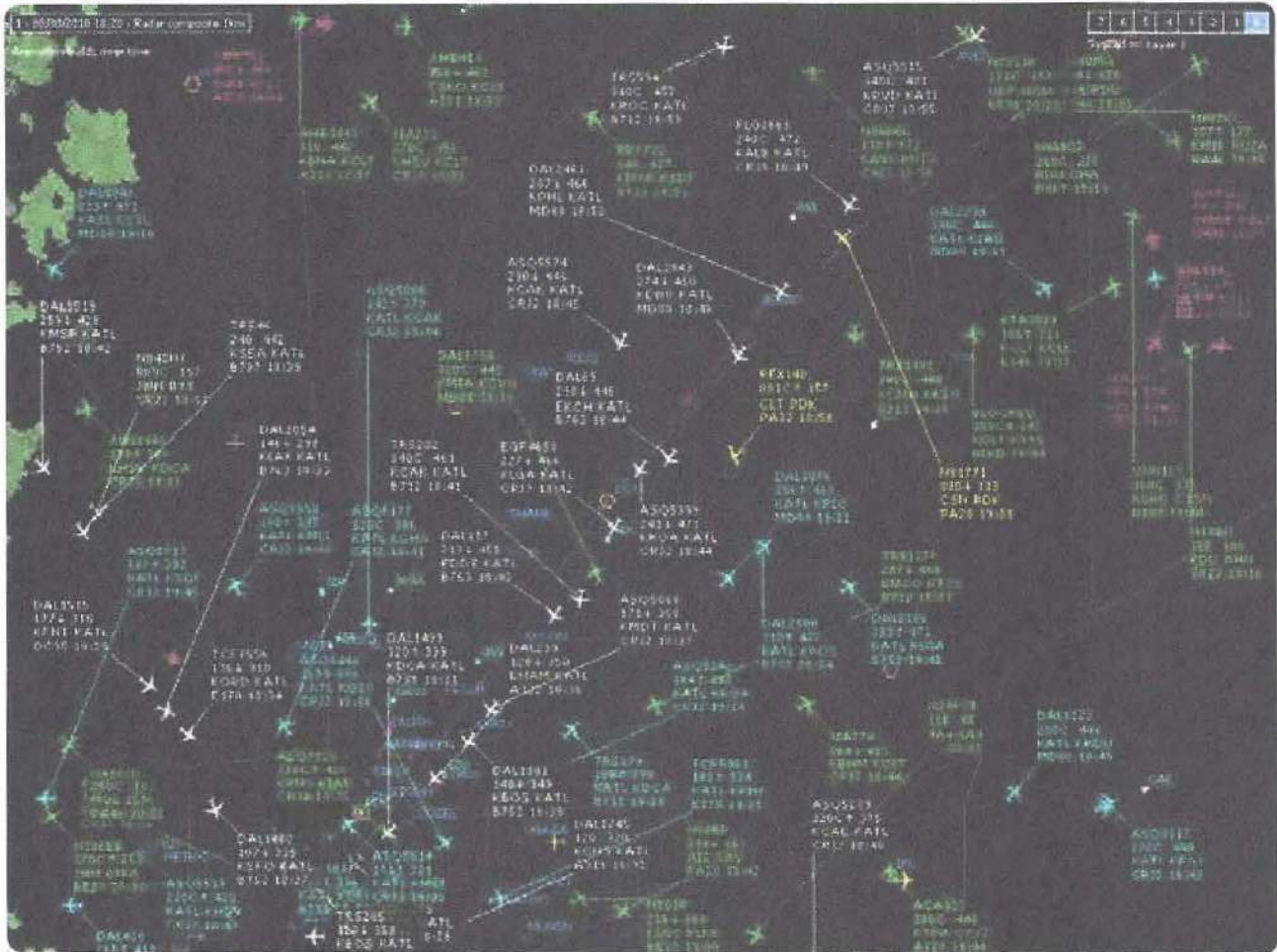
Figure 5-145. Air traffic control radar technology and an onboard radar beacon transponder work together to convey and display air traffic information on a PPI radar screen. A modern approach ATC PPI is shown. Targets representing aircraft are shown as little aircraft on the screen. The nose of the aircraft indicates the direction of travel. Most targets shown above are airliners. The data block for each target includes the following information either transmitted by the transponder or matched and loaded from flight plans by a flight data processor computer: call sign, altitude/speed, origination/destination, and aircraft type/ETA (ZULU time). A "C" after the altitude indicates the information came from a Mode C equipped transponder. The absence of a C indicates Mode S is in use. An arrow up indicates the aircraft is climbing. An arrow down indicates a descent. White targets are arrivals, light blue targets are departures, all other colors are for arrivals and departures to different airports in the area.
