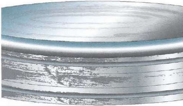
Figure 13-67. Bearing cups should be tight in the wheel boss and should never rotate. The outside of a bearing cup that was spinning while installed in the wheel is shown.
