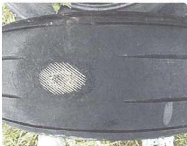
Figure 13-128. Landing with the brake on causes a tire flat spot that exposes the under tread and requires replacement of the tire.
