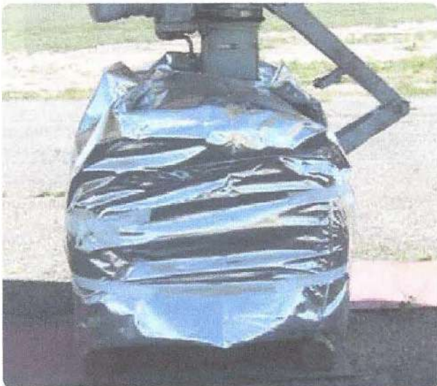
Figure 13-133. Cover tires to protect from harmful chemicals and from the elements when parked outside for long periods of time.
