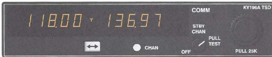
Figure 5-116. A NAV/COM receiver typically found in light aircraft.
