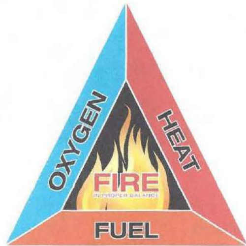
Figure 8-1. The fire triangle; all three elements shown are required for fire to occur.
