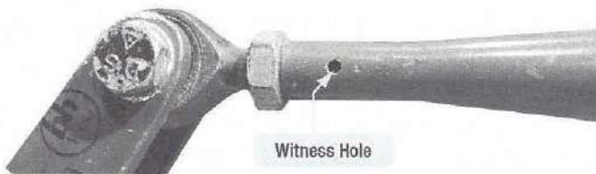
Figure 9-15. Witness hole in push-pull tube. When the terminal end is adequately threaded into the tube, the threads will block the witness hole.
