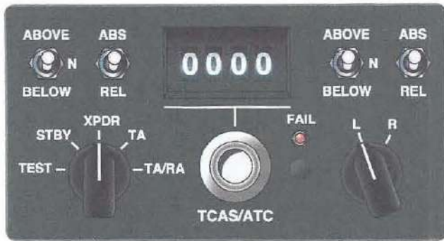
Figure 5-151. This control panel from a Boeing 767 controls the transponder for ATC use and TCAS.
