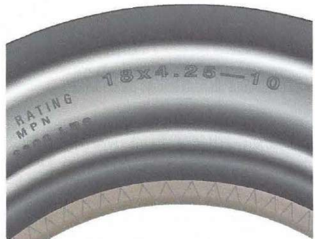
Figure 13-115. A Type VIII or three part nomenclature tire is identified by 3 parameters: overall diameter, section width, and rim diameter.
