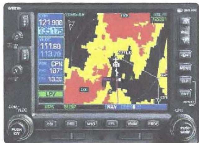
Figure 5-169. A GPS unit integrated with NAV/COM circuitry.
