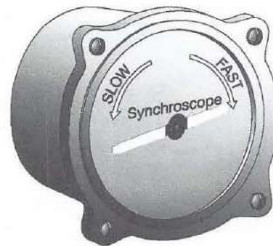
Figure 5-59. This synchroscope indicates the relative speed of the slave engine to the master.
