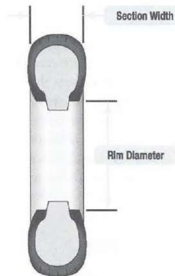
Figure 13-113. Type III aircraft tires are identified via a two number system with a (-) separating the numbers. The first number is the tire section width in inches. The second number is the rim diameter in inches. For example: 6.00 X 6 is a Cessna 172 tire that is 6.00 inches wide and fits on a rim that has a diameter of 6 inches.
