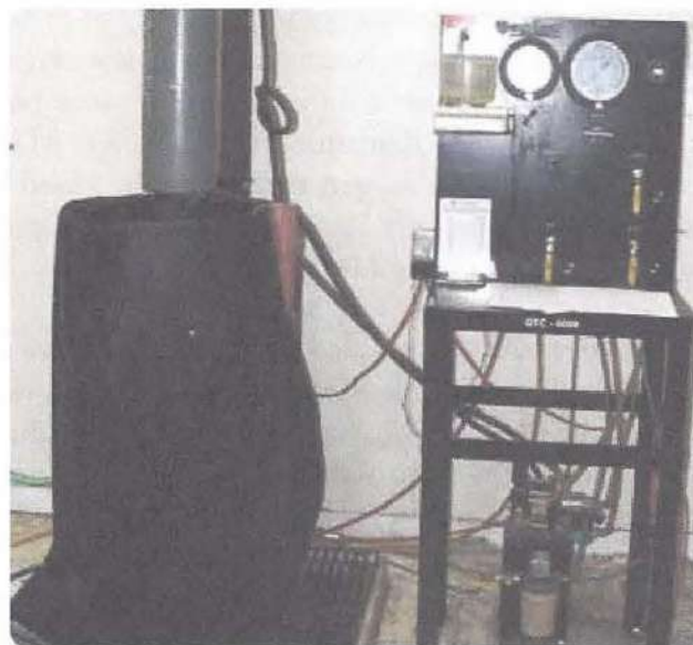
Figure 15-4. This test stand is used for hydrostatic testing of oxygen cylinders. The water-filled cylinder is lowered into the barrel on the left where it is pressurized to the proper level as monitored via gauges mounted on the control panel. A displacement container on the top left of the control board collects water from the barrel to measure the expansion of the cylinder when pressurized to ensure it is within limits.
