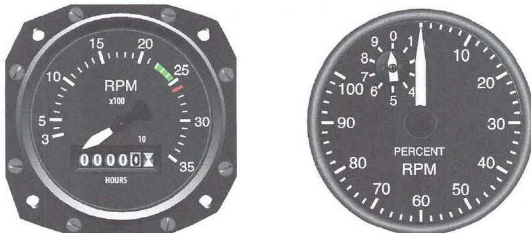
Figure 5-52. A tachometer for a reciprocating engine is calibrated in rpm. A tachometer for a turbine engine is calculated in percent of rpm.
