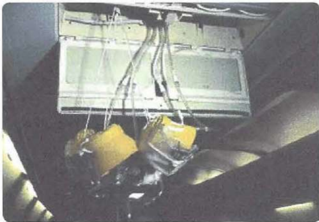
Figure 15-15. A passenger service unit (psu) is hinged over each row of seats in an airliner. Four yellow continuous flow oxygen masks are shown deployed. They are normally stored behind a separate hinged panel that opens to allow the masks to fall from the PSU for use.
