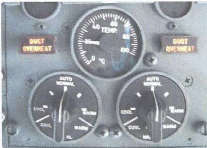
Figure 4-39. Typical temperature selectors on a transport category aircraft temperature control panel in the cockpit (left) and a business jet (right). On large aircraft, temperature selectors may be located on control panels located in a particular cabin air distribution zone.
