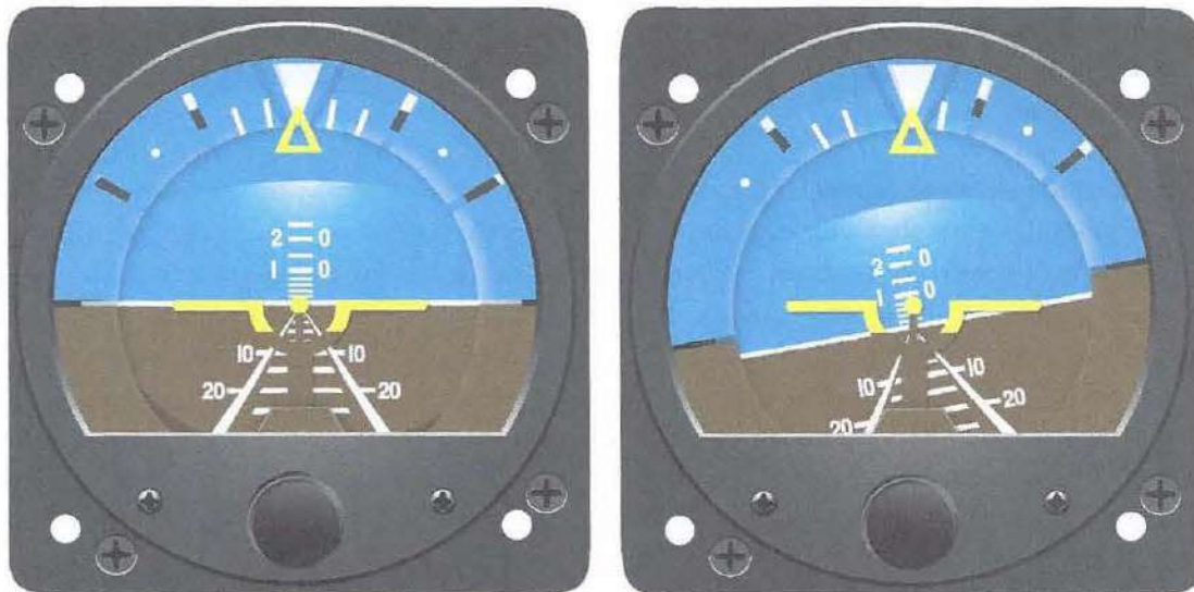
Figure 5-94. A typical vacuum-driven attitude indicator shown with the aircraft in level flight (left) and in a climbing right turn (right).
