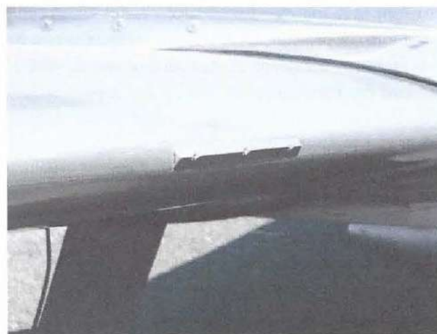
Figure 1-36. A stall wedge causes the wing root to stall before the outboard wing. This preserves airflow over the ailerons for controlled recovery from the stall.
