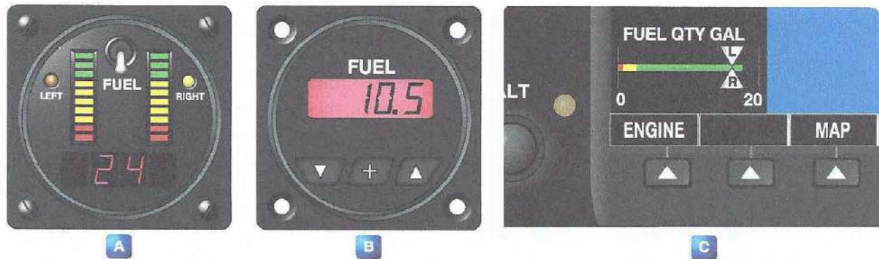
Figure 10-31. Digital fuel quantity gauges that work off of variable resistance from the tank unit are shown in A and B. The fuel quantity indication of a Garmin G-1000 flat screen display is shown in C.
