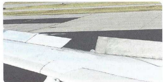
Figure 9-9. Speed Brakes for Aerodynamic Braking. The flight spoilers, shown as the two panels in the center, join the ground spoilers to maximize aerodynamic braking after landing. Note: the aileron near wing tip is not above the wing with flight spoilers acting as speed brakes.
