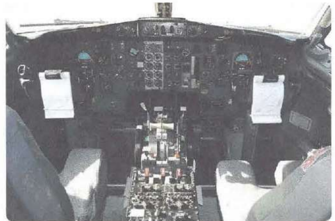
Figure 19-1. An older instrument panel with many discrete indicators.
