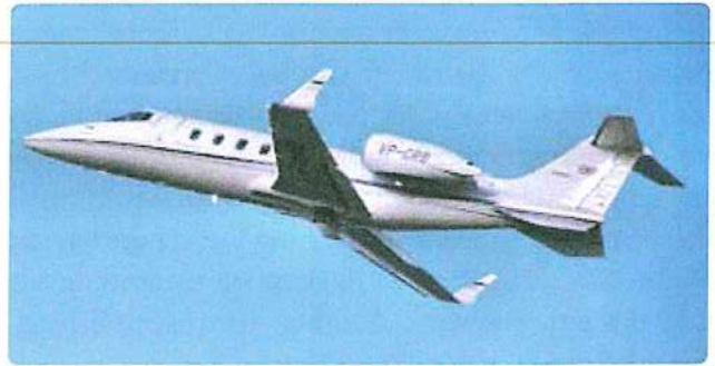
Figure 2-20. Winglets help reduce induced drag.
