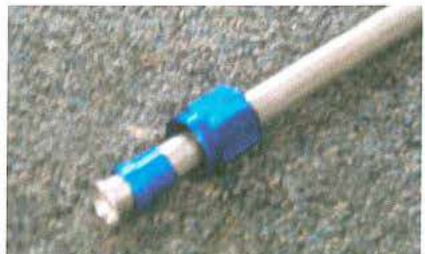
Flared tube assembled with sleeve and nut.
