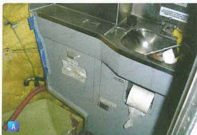
Figure 4-15. (A) Typical lavatory floor damages shown with the toilet is removed. (B) Corrosion caused by water and urine collecting on a lavatory attach bracket.
