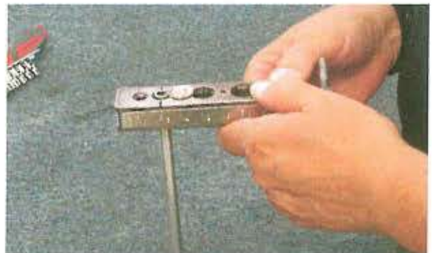
Setting tube in die (dime's thickness over top).
