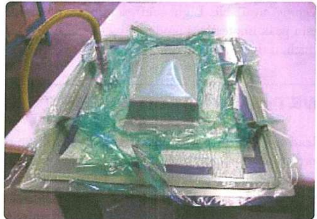
Figure 3-50. Vacuum bagging of contoured part.
