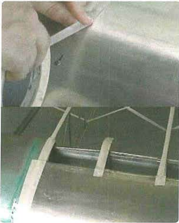
Figure 3-147. Anti-chafe tape is applied to all features that might cut or wear through the fabric.
