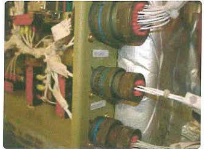
Figure 11-52. Connector arrangement to avoid wrong connection.
