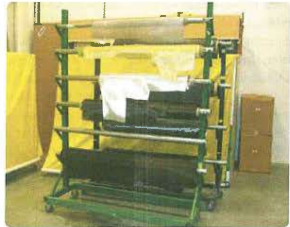
Figure 3-14. Dry fabric materials (top to bottom: aluminum lightning protection mesh, Kevlar®, fiberglass and carbon fiber).
