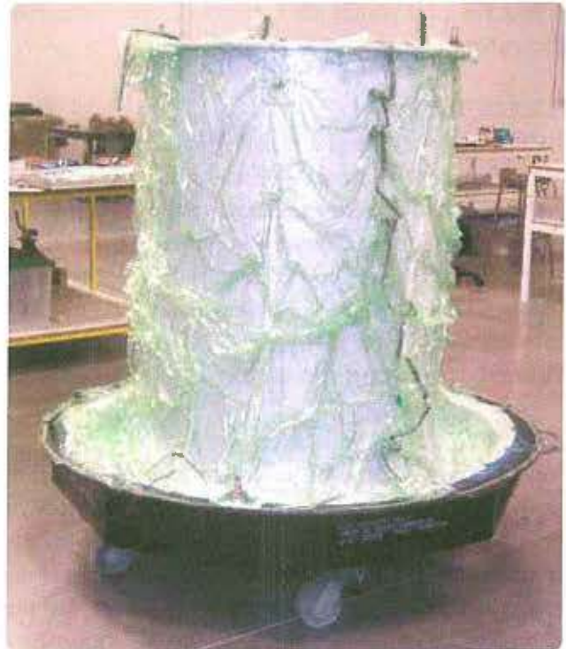
Figure 3-38. Bagging of complex part.
