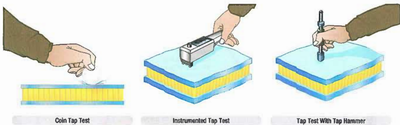
Figure 3-57. Tap testing techniques.
