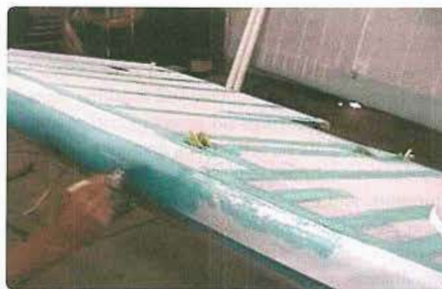
Figure 3-162. Cement is brushed through a four-inch tape during installation over the fabric seam on a wing leading edge. Two-inch tapes cover the wing rib and rib lacing.
