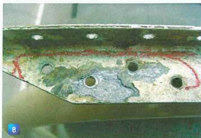
Figure 4-15. (A) Typical lavatory floor damages shown with the toilet is removed. (B) Corrosion caused by water and urine collecting on a lavatory attach bracket.
