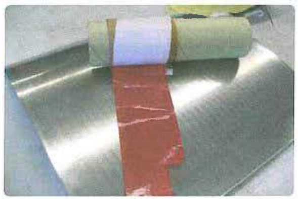
Figure 3-16. A roll of film adhesive.
