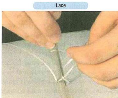
Figure 3-135. Clips, screws, rivets, or lace are used to attach the fabric to wing and empennage ribs.
