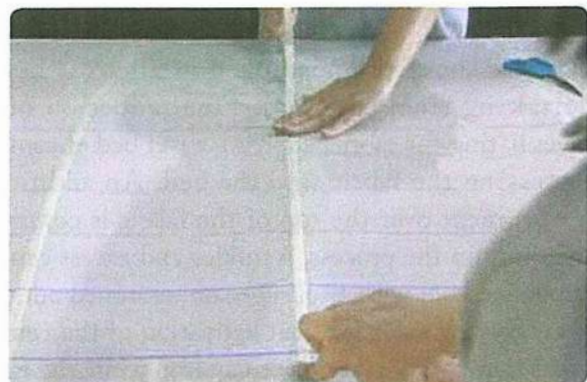
Figure 3-152. Reinforcing tape the same width as the wing ribs is applied over all wing ribs.
