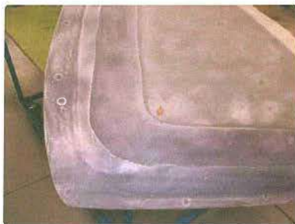
Figure 3-11. Aluminum mesh lightning protection material.
