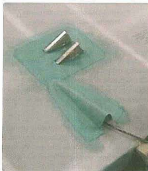
Figure 3-161. A strut fitting and cable guide with reinforcing fabric gussets cemented in place.
