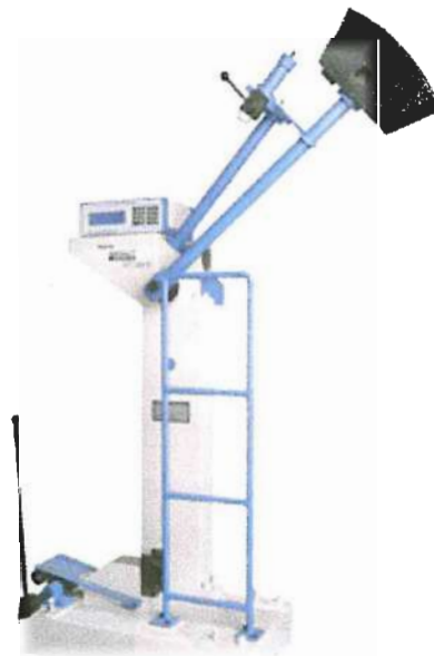
Figure 1-10. An IZOD impact test machine.
