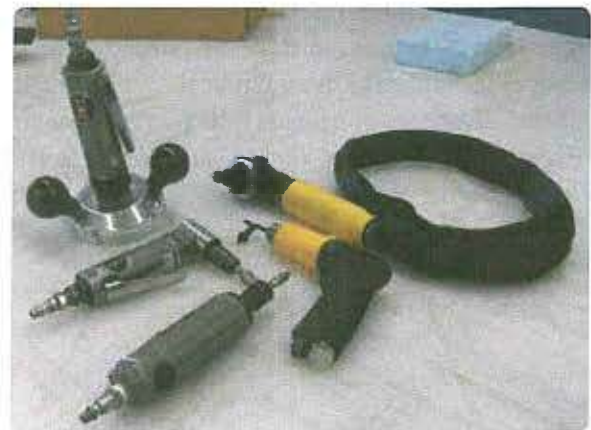
Figure 3-34. Air tools used for composite repair.
