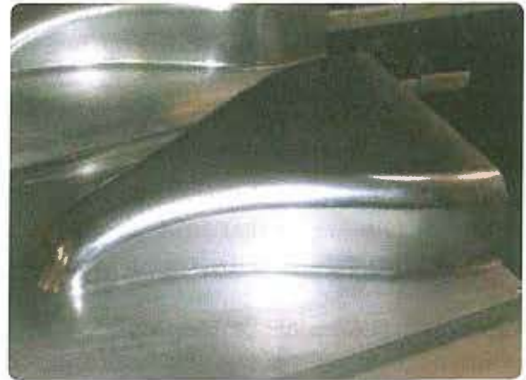
Figure 3-36. A mold of an inlet duct.
