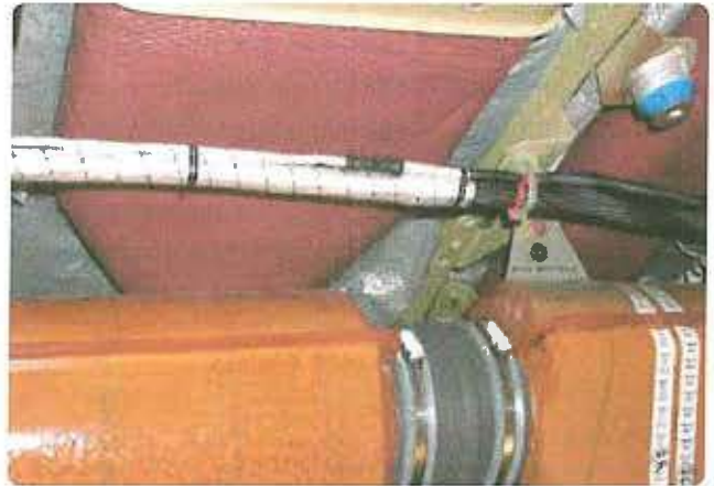
Figure 11-4. Shielded wire harness for flight control.
