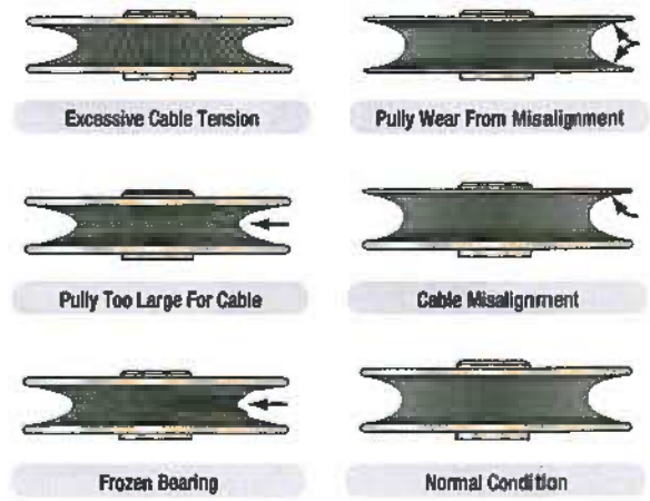
Figure 10-3. Pulley wear patterns.
