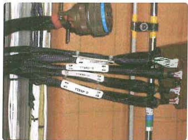
Figure 11-18. Alternate method of identifying wire bundles.
