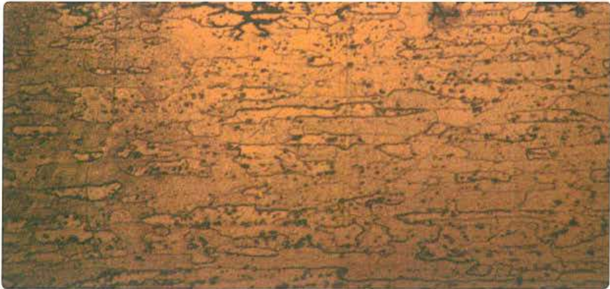
Figure 4-9. Intergranular corrosion present on 6061-T6 aluminum.
