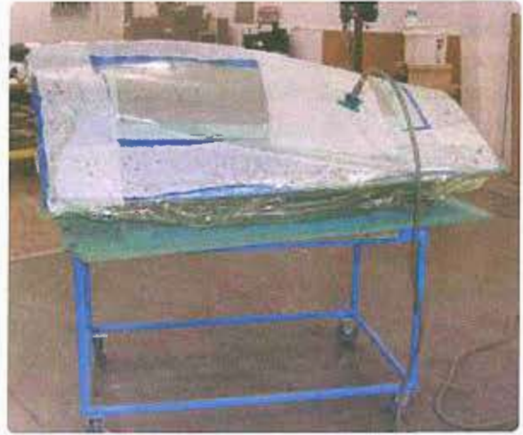
Figure 3-54. Envelope bagging of repair.
