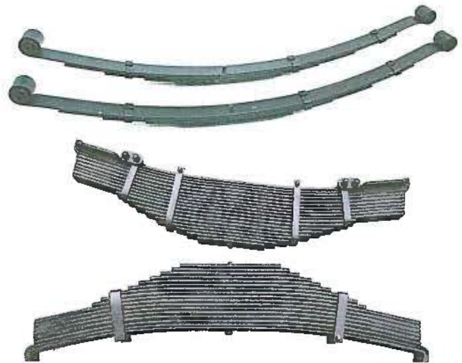
Figure 7-2. Example of leaf springs.
