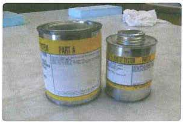
Figure 3-17. Two-part paste adhesive.
