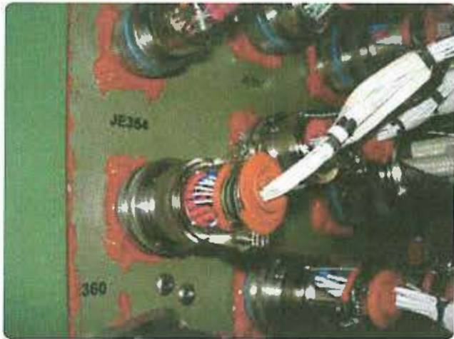
Figure 11-53. Backshells with strain relief.
