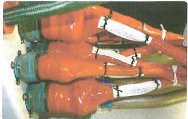
Figure 11-5. Wire harness with protective jacket.
