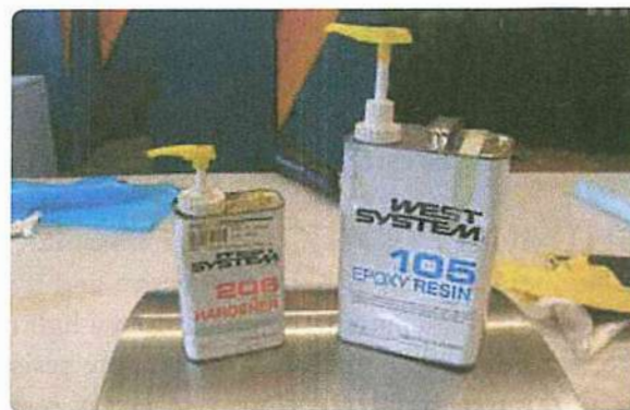
Figure 3-12. Two part wet layup epoxy resin system with pump dispenser.
