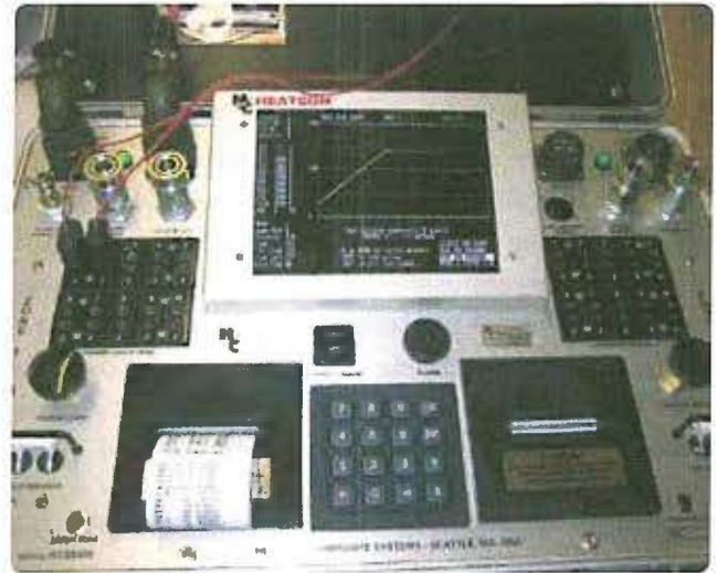
Figure 3-42. Heat bonder equipment.
