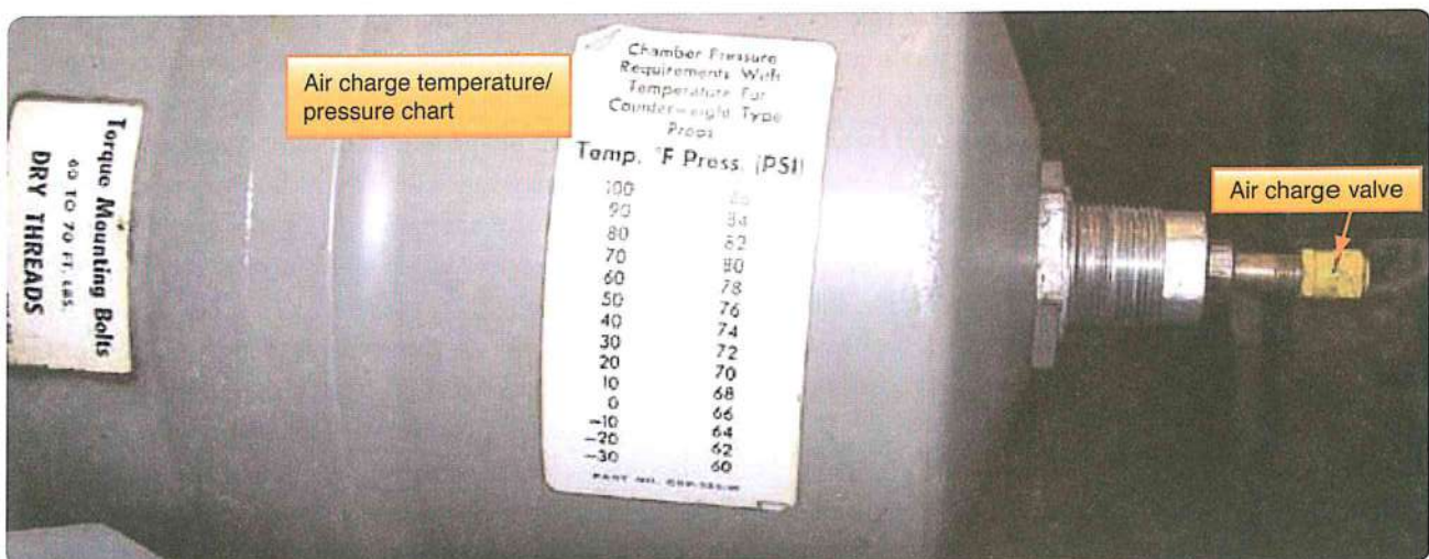
Figure 6-21. Gas charging port on propeller dome.
