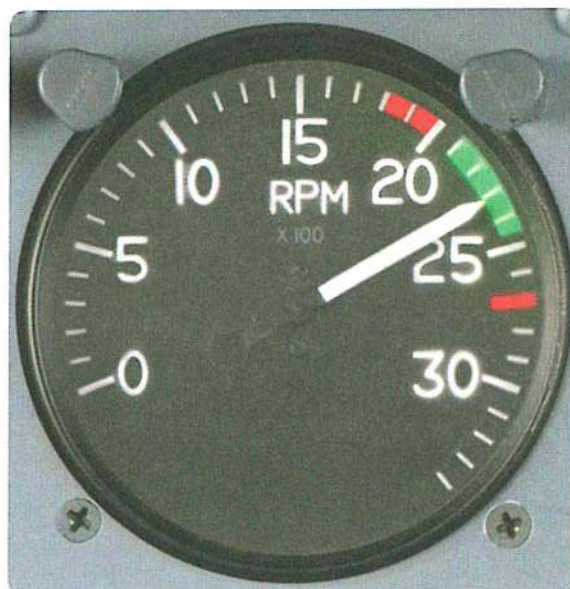
Figure 1-17. Red arc from 1 800 to 2 000 rpm.
