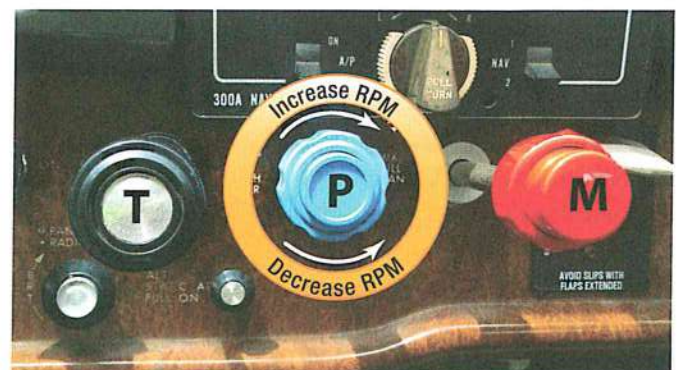
Figure 3-2. Push-pull type controls for throttle (T), propeller (P), and mixture (M). Rotating the propeller vernier control clockwise increases the on speed rpm. Pressing the release button in the center of the knob allows the control to be rapidly moved in a linear fashion. Both the propeller and mixture controls are equipped with the vernier feature in this illustration.
