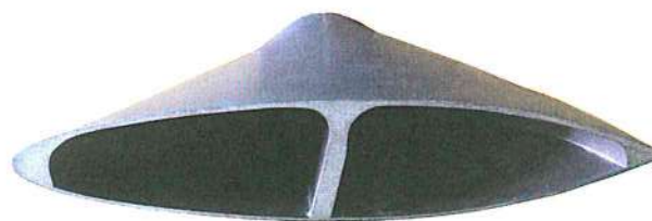
Figure 2-8. Cross section of steel propeller blade.
