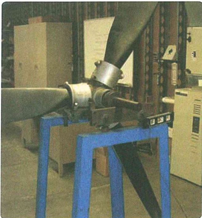
Figure 6-11. Checking three-bladed propeller for static balance with blade in other-than-vertical position using knife-edge stand.
