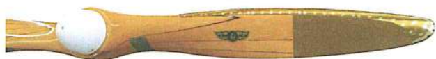
Figure 2-3. Wooden propeller showing spinner, hub, laminates, metal tipping, fabric covering, and drain holes.
