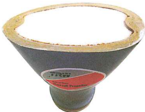
Figure 2-10. Cross section of composite propeller blade.
