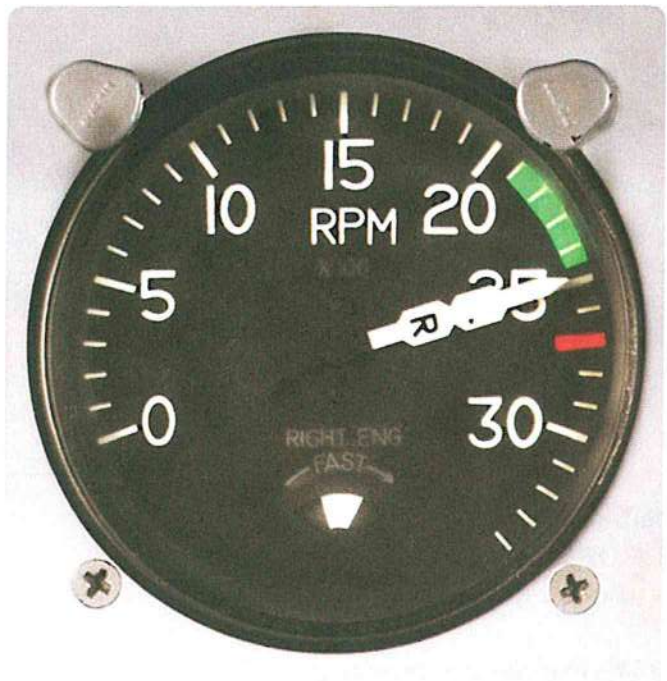
Figure 4-1. Twin engine tachometer with synchronizing disk or synchroscope.
