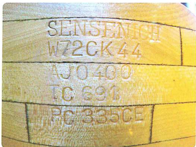
Figure 2-2. Propeller data. This propeller has a 72-inch diameter with a 44-inch pitch. It could serve as a climb propeller on some airplanes and a cruise propeller on others. Note the laminates.
