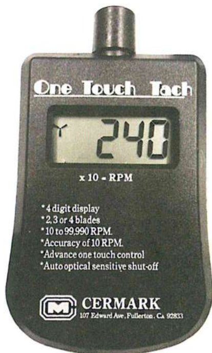
Figure 6-22. Electronic handheld tachometer checker. Note number of propeller blades shown in upper left of display window and rpm X 10 shown in display. In this example, a three bladed propeller was revolving at 2 400 rpm.
