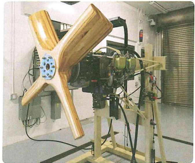
Figure 2-12. Club propeller used in test cell.
