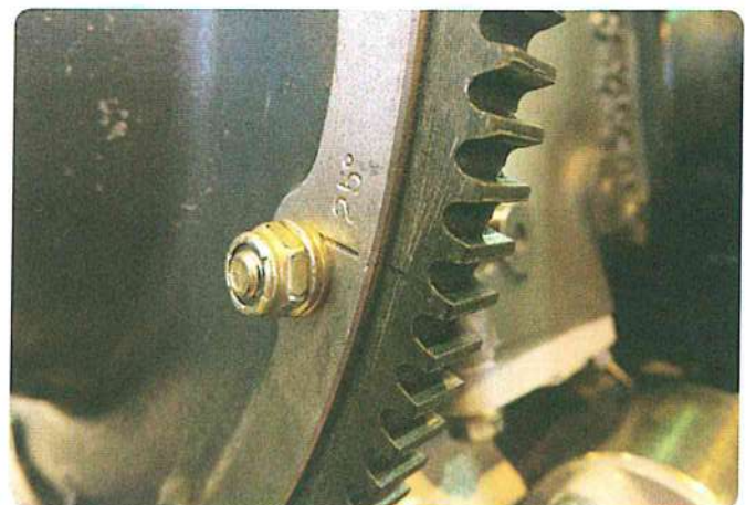
Figure 6-13. Weight added to Lycoming starter ring gear.
