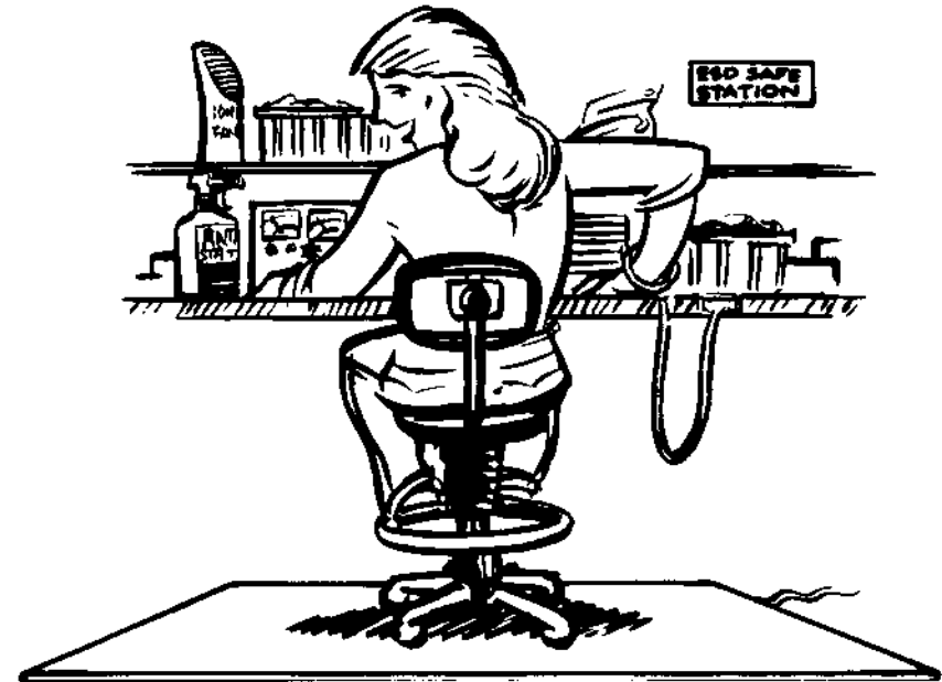
Figure 13: ESD Safe Workstation
