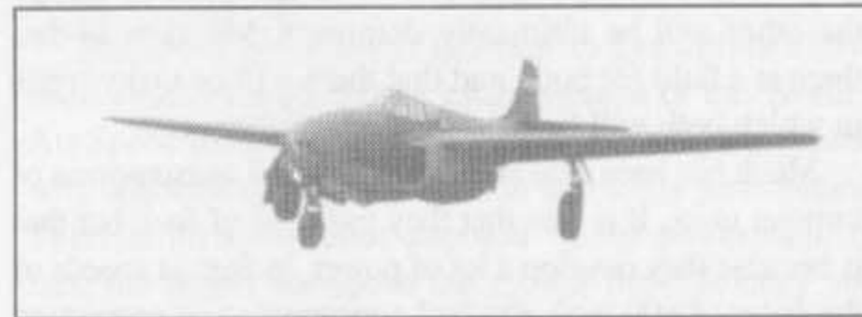
Fig. 1-17 — The Bell "Airacomet" was a twin turbojet fighter, powered by two Whittle-type G.E. gas turbines.
