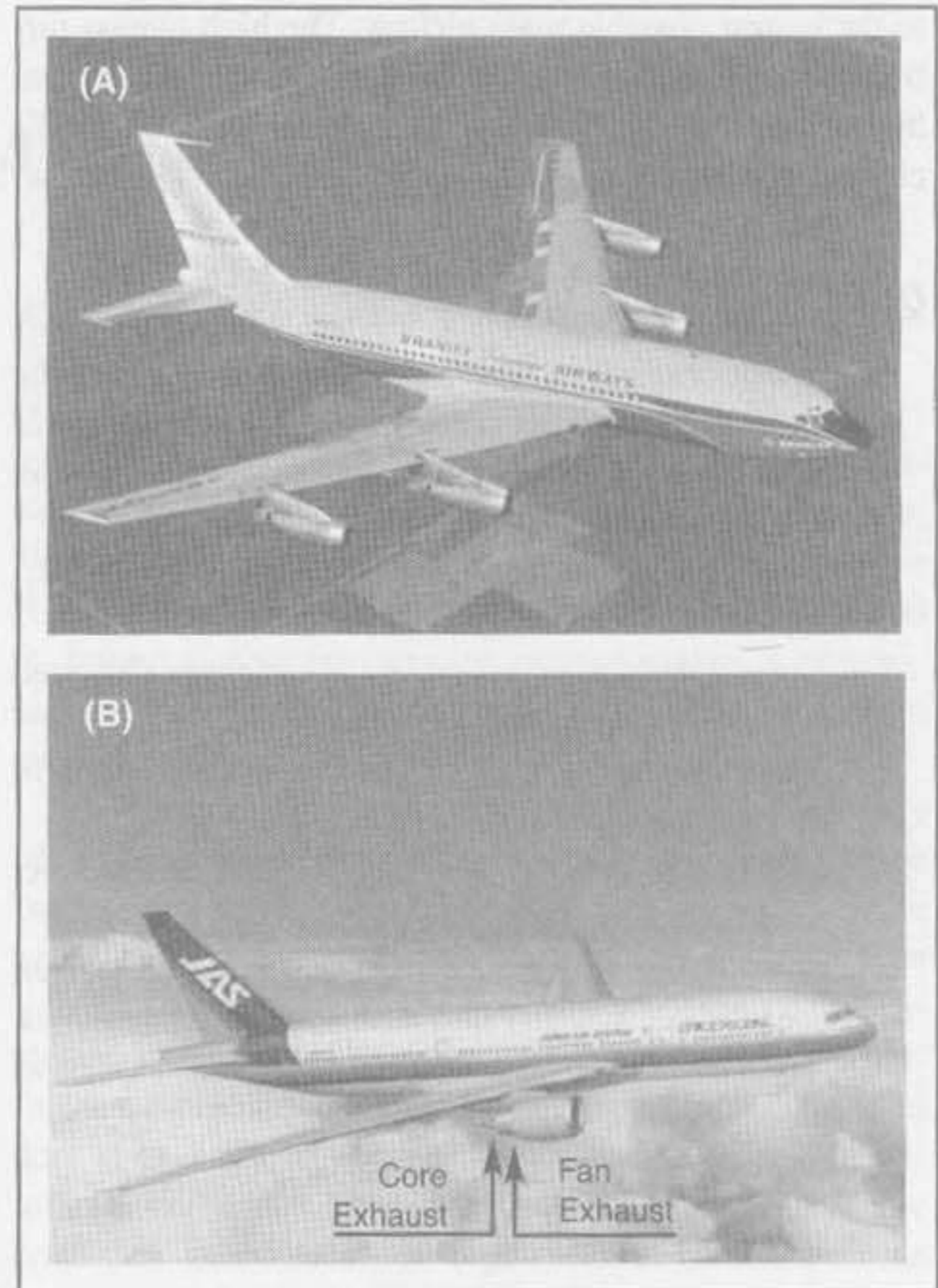
Fig. 2-50A — Early turbojet powered airliner with narrow inlet and single exhaust.
