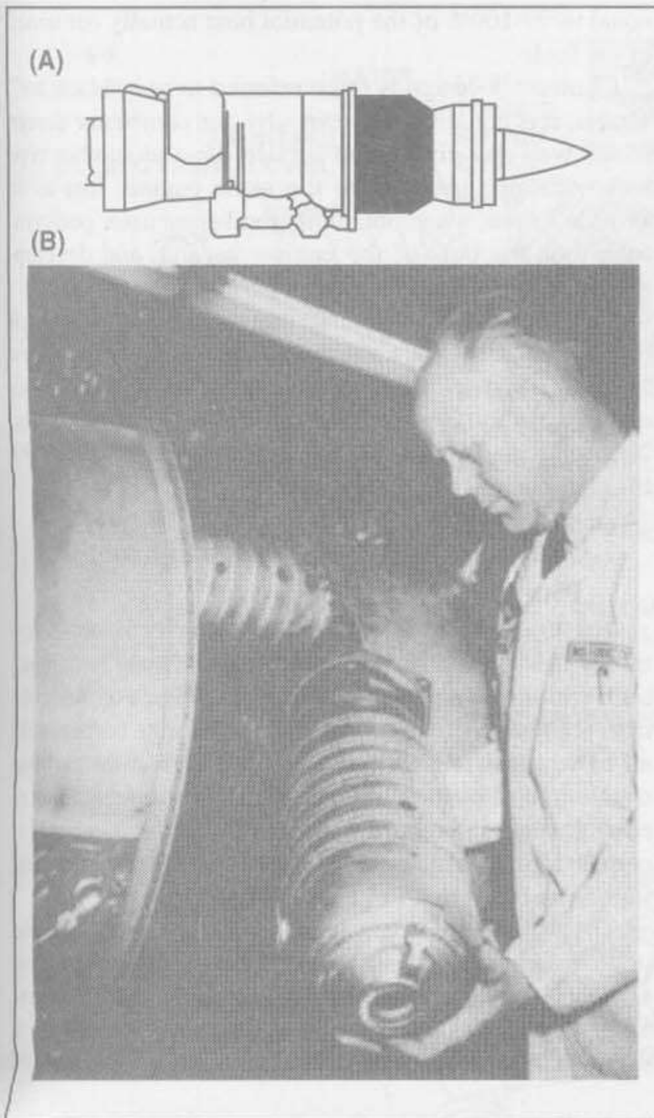
Fig. 3-48A — Location of combustor. Fig. 3-48B — Removal of through-flow, can-annular liner, from Pratt & Whitney JT8D turbofan.
