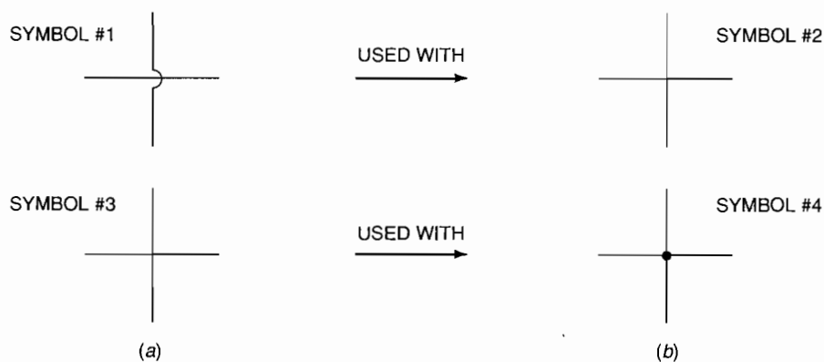
FIGURE 4-42 Wiring diagram symbols for electric wire. (a) Wires without an electrical connection; (b) wires with an electrical connection.
