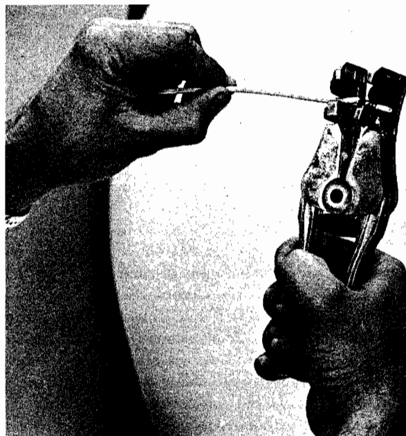
FIGURE 4-16 Use of a wire stripper.
