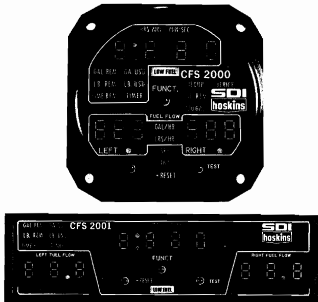
FIGURE 17-19 Indicator panels for a computerized fuel system. (Symbolic Displays, Inc.)
