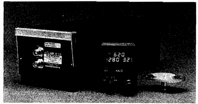
FIGURE 15-30 Microwave landing system equipment; from left to right: the airborne receiver, the digital display-control panel, and the MLS antenna. (Bendix Avionics Division)
