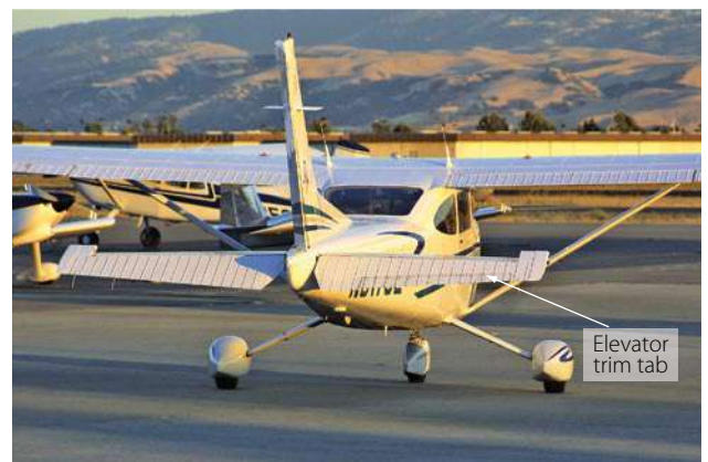
Figure 3-71. Elevator trim tab on a Cessna 182.
