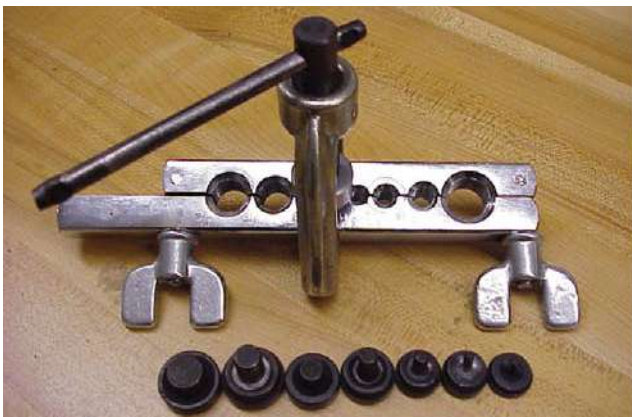
Figure 7-10. Double flare tool.
