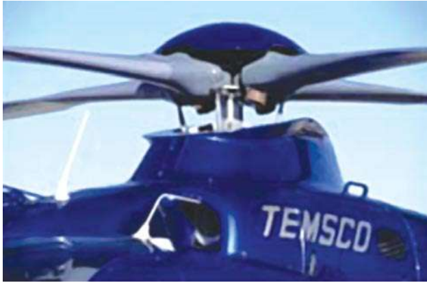
Figure 3-85. Eurocopter Model 135 rigid rotor system.
