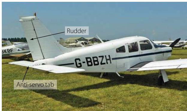
Figure 3-70. Rudder on a Piper Cherokee Arrow.
