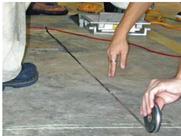
Figure 4-18. Measuring the nosewheel arm on a Cessna 310.
