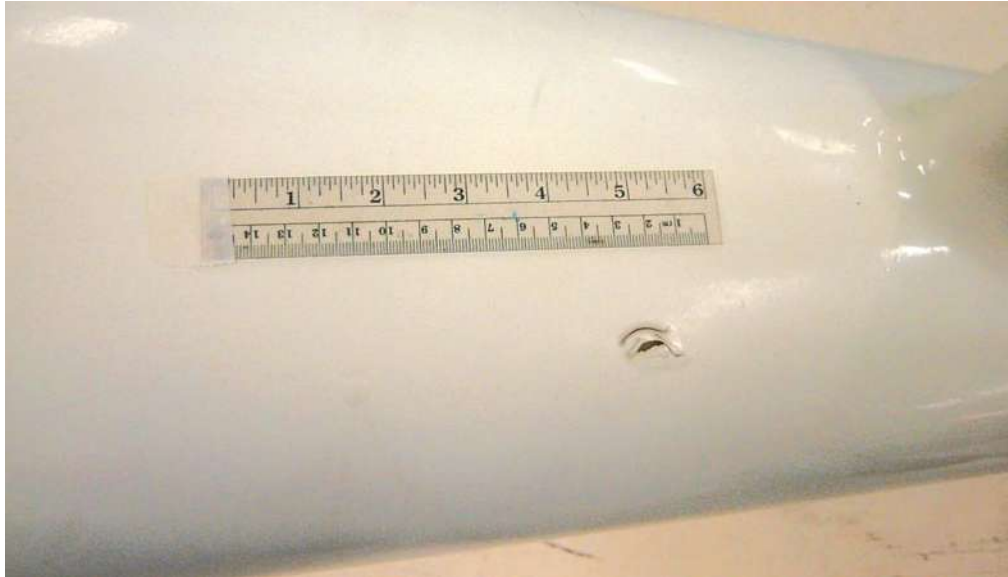
Figure 2-32. Digital image of impact damage.
