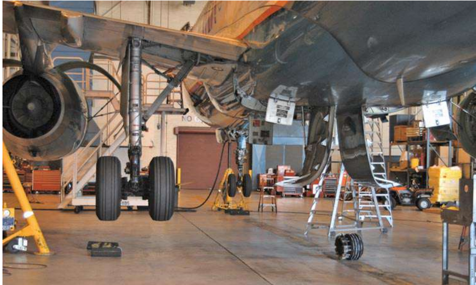
Figure 3-4. Airbus A-320 being jacked.
