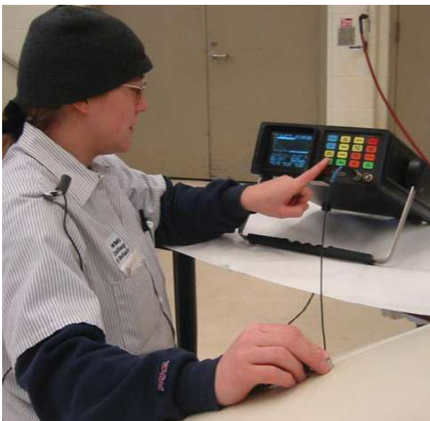
Figure 8-12. Ultrasonic inspection of a composite structure.
