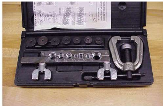
Figure 7-10. Double flare tool.
