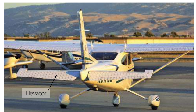
Figure 3-65. Elevator on a Cessna 182 provides pitch control.
