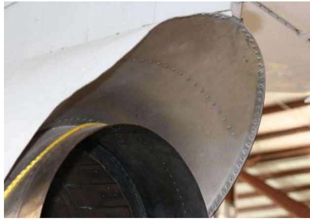
Figure 6-11. Exhaust nozzle area.
