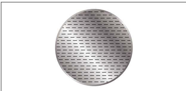
Figure 10-10. Even distribution of charge on metal disk.
