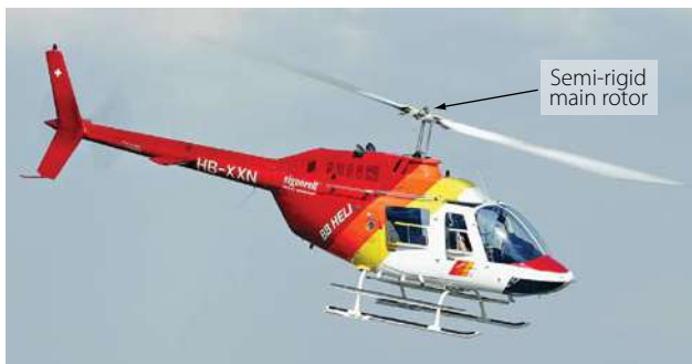
Figure 3-84. Bell Jet Ranger with semi-rigid main rotor.
