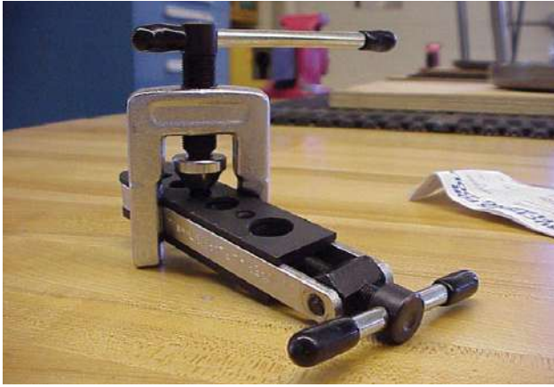
Figure 7-9. Hand flaring tool.
