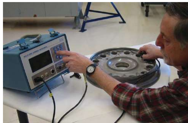
Figure 8-5. Eddy current inspection of wheel half.
