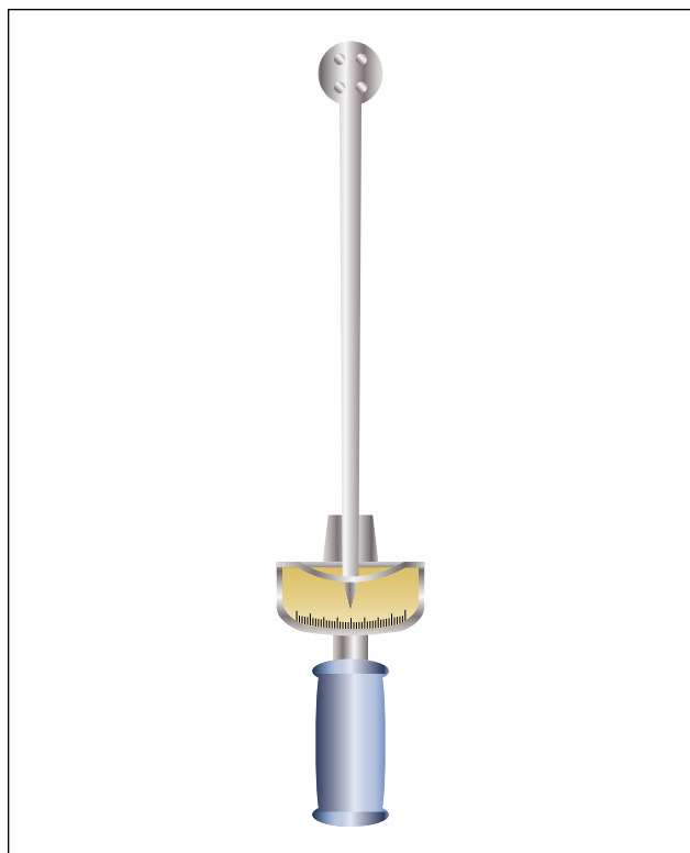
Figure 3-24. Deflecting beam torque wrench, measures strain by distortion.
