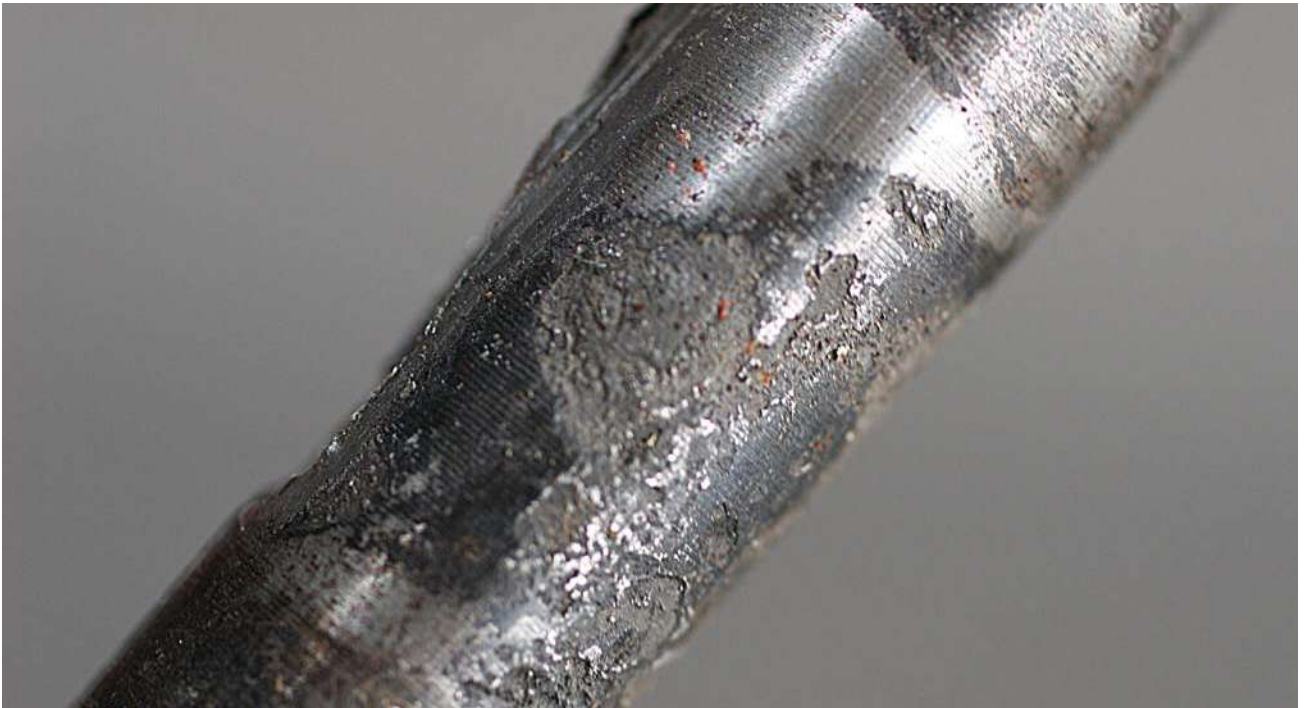
Figure 6-7. Dissimilar metal corrosion.
