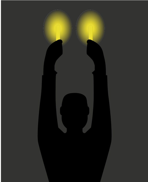
Figure 11-26. Night operations with wands.
