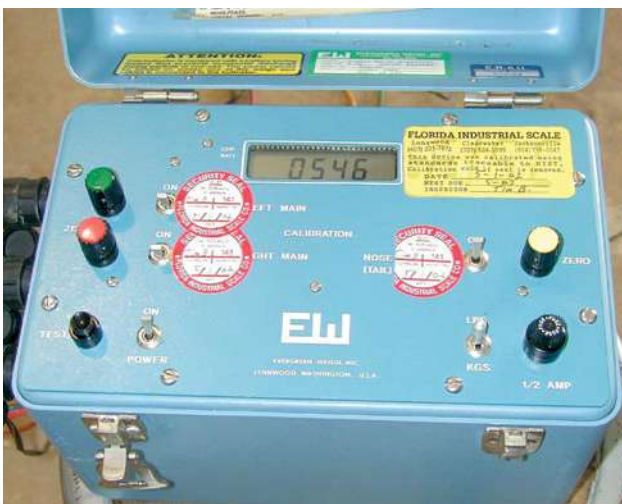
Figure 4-14. Display unit showing nosewheel weight for Mooney M20.
