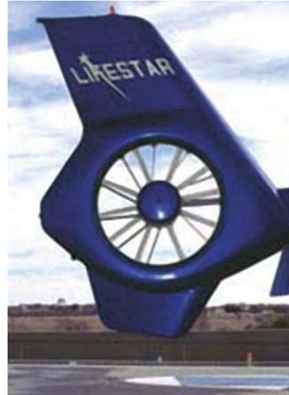
Figure 3-87. Fenestron on a Eurocopter Model 135.
