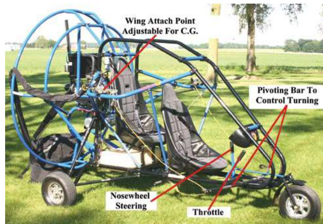
Figure 4-39. Powered parachute structure with wing attach points.
