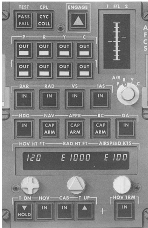
Figure 9.22 EH 101 AFCS pilot's control unit (Courtesy of Smiths Group – now GE Aviation)
