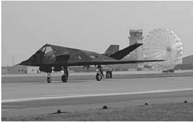
Figure 4.32 F117 deploying brake parachute (Courtesy of US Air Force/ Senior Airman Darnell Cannady)
