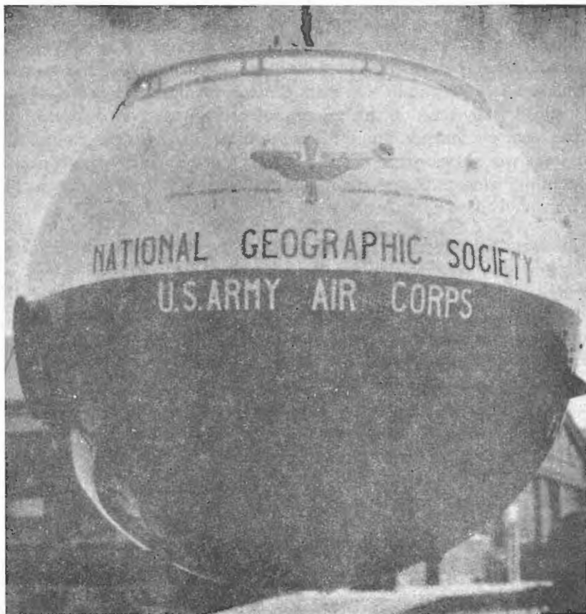
FIGURE 47. Stratosphere Gondola; Magnesium-alloy Sheet
