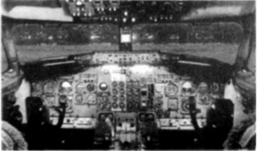
Figure 1.19 Flight instrument grouping. (a) Basic six; (b) basic 'T' (with flight director system indicators).
