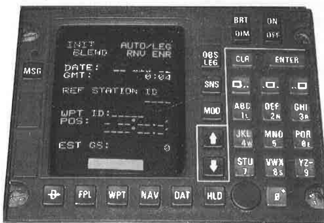
FIGURE 15-34 Push-button control panel for a navigation system.
