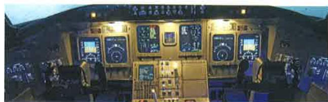
FIGURE 6-85 A modern instrument panel replaces conventional instruments with multiple flat panel displays.
