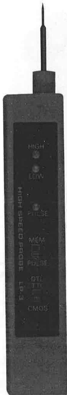
FIGURE 7-80 A logic probe. ( Global Specialties, an Interplex Electronic Company. )
