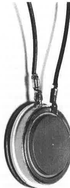
FIGURE 11-36 A 600-A power transistor. (Westinghouse Electric Corporation.)
