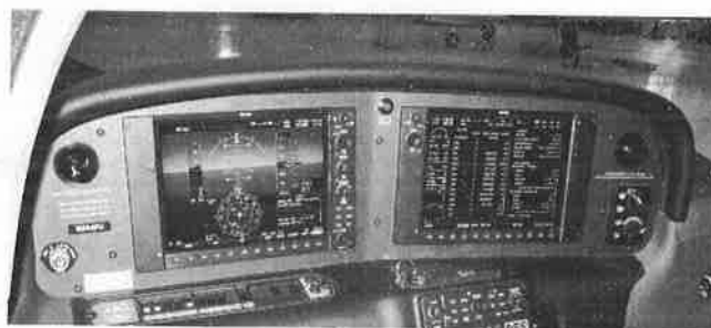
FIGURE 17-25 Light aircraft electronic display systems (the Cirrus SR20).
