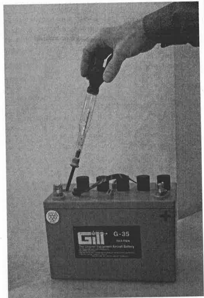
FIGURE 3-20 Performing a specific gravity test using a hydrometer.
