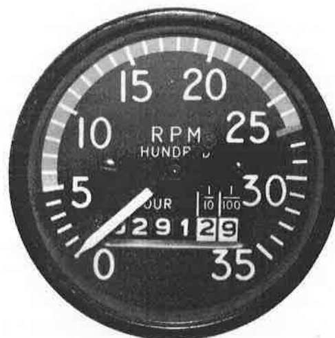
FIGURE 17-1 Tachometer for a reciprocating engine.
