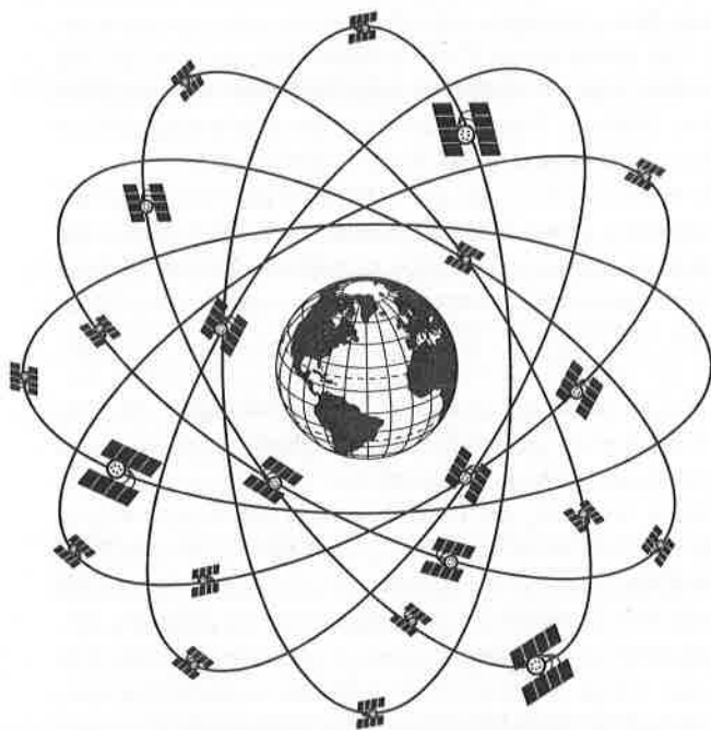
FIGURE 15-38 Orbiting satellites for a GPS.
