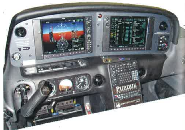
FIGURE 12-7 Cirrus SR20 instrument panel.
