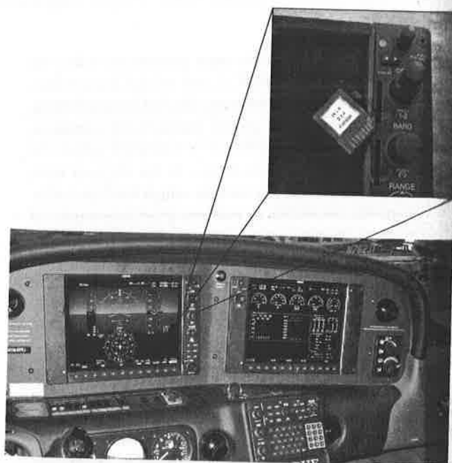
FIGURE 13-53 A secure data (SD) card used for software configuration on the G-1000 system.
