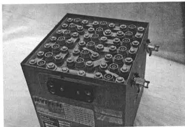
FIGURE 3-27 A 20-cell nickel-cadmium battery, top removed.
