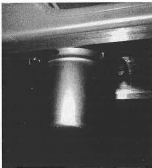
FIGURE 17-40 A typical flux detector for an electronic compass system.
