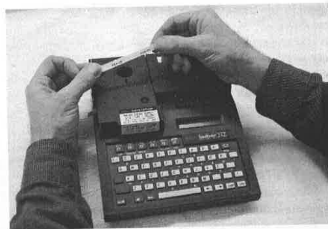
FIGURE 4-47 Wire marking machine for heat shrink tubing.
