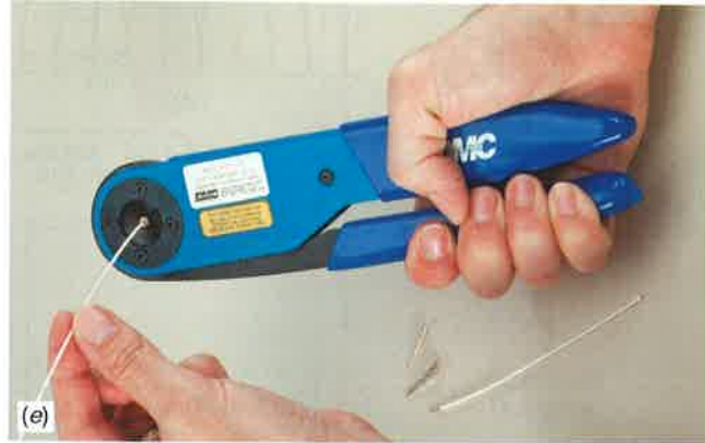
FIGURE 4-34 Common steps used during the crimping process. (a) Select the correct crimping tool and adaptors for the wire and pin being crimped. (e) Completely compress (squeeze) handles until tool automatically releases. (Daniels Manufacturing Corporation.)
