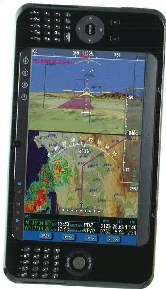
FIGURE 17-28 The AV80R portable multifunction display designed for light aircraft. (Bendix King, by Honeywell.)
