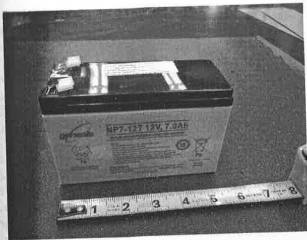
FIGURE 11-20 Battery #3 Cirrus aircraft; one of two batteries connected in a series.
