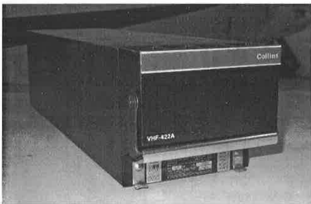
FIGURE 15-4 A VHF communications transmitter/receiver LRU for a typical corporate aircraft.
