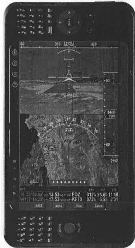
FIGURE 17-28 The AV80R portable multifunction display designed for light aircraft. See also color insert. (Bendix King, by Honeywell.)
