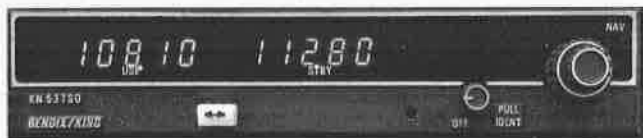
FIGURE 15-24 Panel-mounted VHF navigation receiver.
