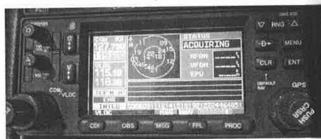
FIGURE 15-39 A typical panel-mounted GPS navigation receiver/processor for light aircraft.
