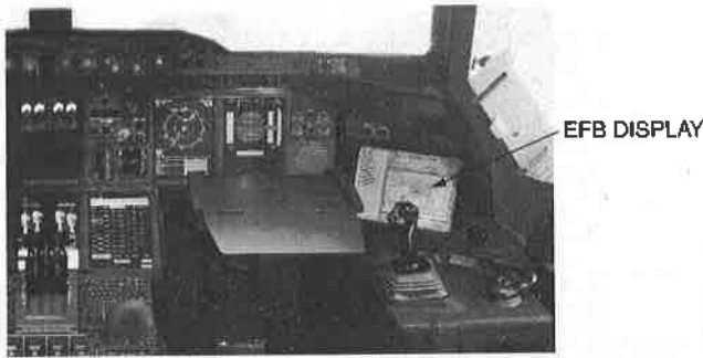
FIGURE 17-29 A-380 Class III electronic flight bag (first officer's station).
