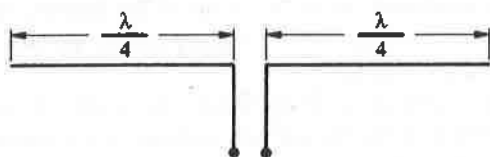
FIGURE 14-10 The Hertz dipole antenna.
