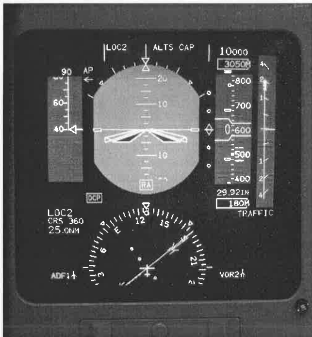
FIGURE 15-23 An electronic primary flight display for a corporate or commuter type aircraft.
