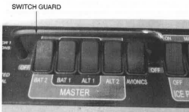
FIGURE 12-3 A master switch control panel for a Cirrus SR22.
