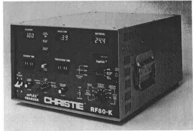
FIGURE 3-34 A typical nickel-cadmium battery charger/analyzer. (The Christie Corporation.)
