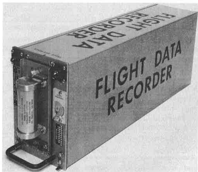
FIGURE 15-48 A flight data recorder. (Sundstrand Corporation.)
