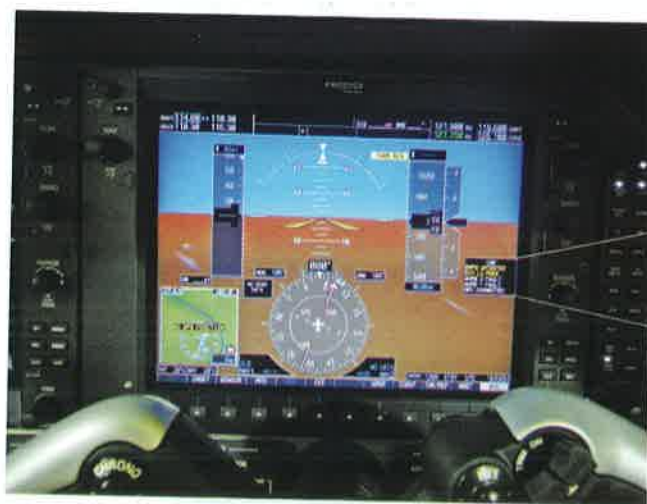
FIGURE 13-10 Caution data shown on a modern flat panel display.
