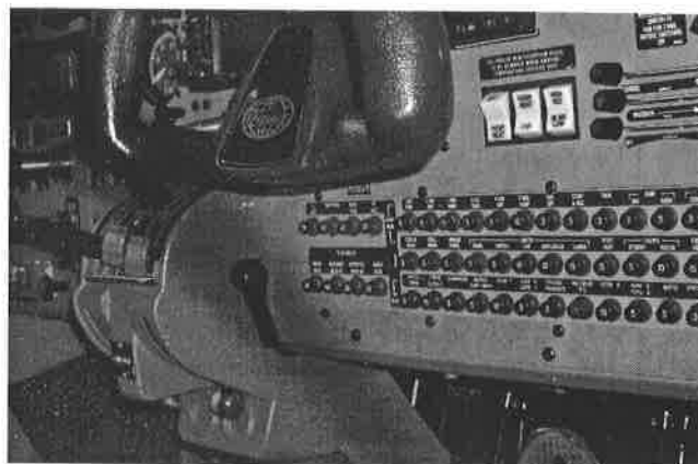
FIGURE 12-2 Circuit breaker panel, twin-engine Piper aircraft.
