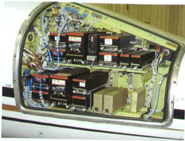
FIGURE 13-1 Forward equipment bay in the nose of a light jet aircraft.
