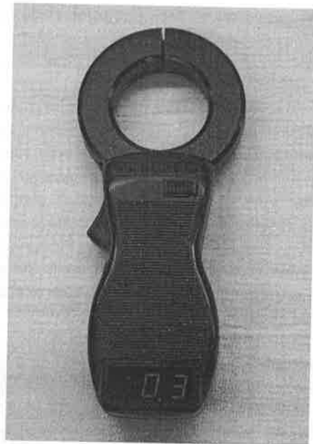
FIGURE 8-21 An inductive pickup meter.
