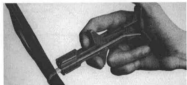
FIGURE 4-12 Typical tie strap installation tool. (Thomas & Betts Corp.)
