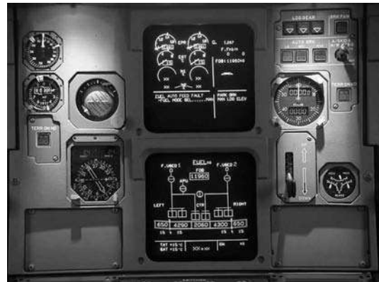
1.18 A320 ECAM displays located above the centre console between the captain and first officer
