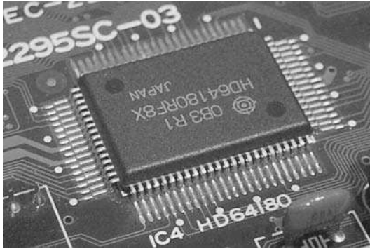
8.3 An 8-bit CMOS microprocessor supplied in an 80-pin plastic quad flat package (PQFP)
