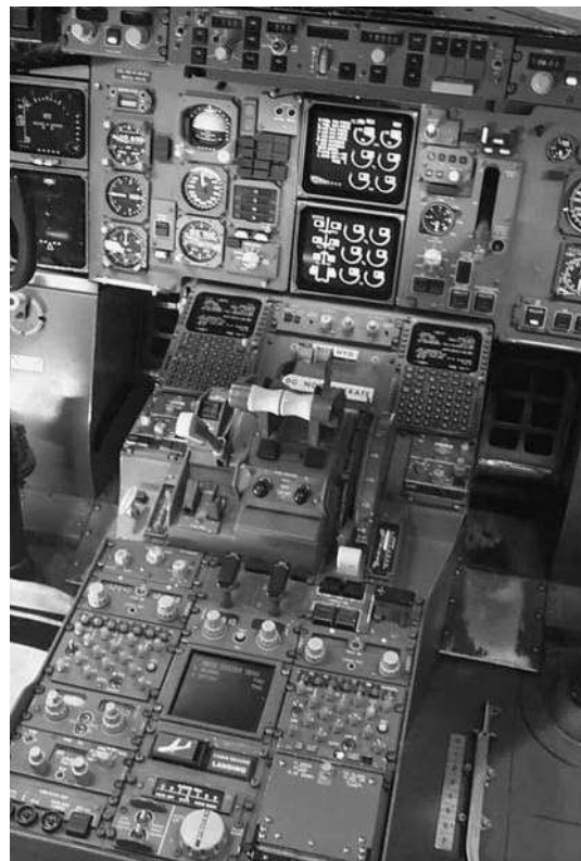
1.1 Boeing 757 flight instruments and displays
