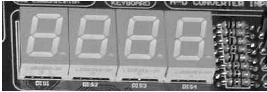
11.13 Typical example of a four-digit seven-segment display
