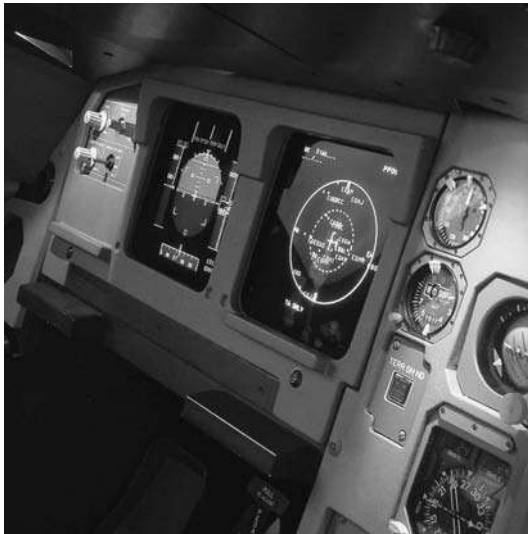
15.3 'Glass cockpit' (EFIS) displays in an A320
