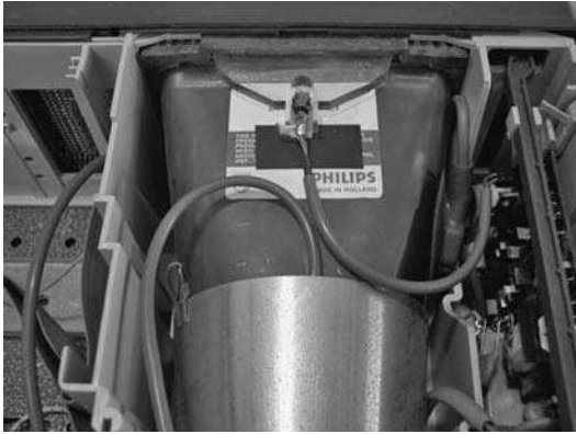
11.2 Rear view of a CRT display showing external graphite coating and mumetal magnetic shielding
