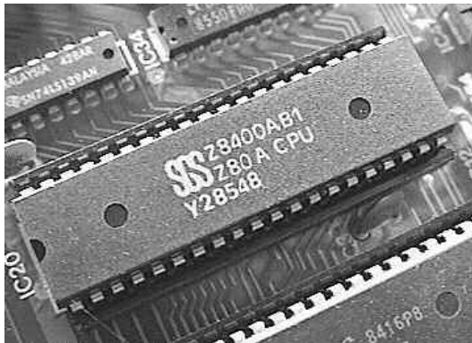
7.5 The Z80 is a basic 8-bit microprocessor supplied in a 40-pin dual-in-line (DIL) package. The chip operates from a single +5 V supply.
