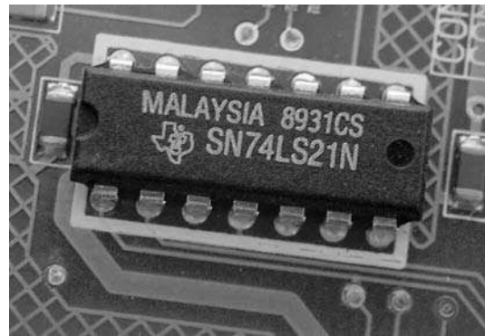
5.28 A low-power Schottky TTL logic circuit supplied in a 14-pin dual-in-line (DIL) package
