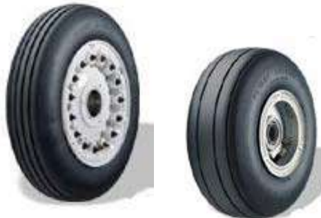
Diagram 8.33 Circumferentially Grooved Tyres
