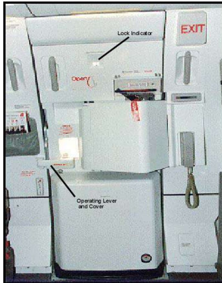
Diagram 15.9 Type I Door Locking Lever and Cover
