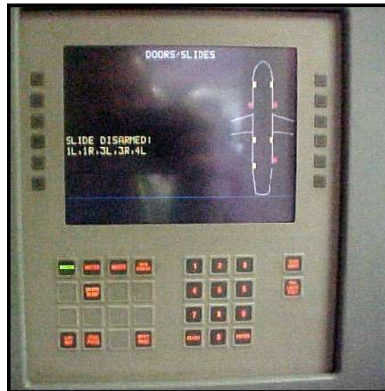
Diagram 15.10 Door Indication on ECAM Lower Screen
