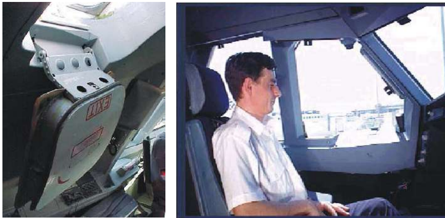
Diagram 15.11 Flight Crew Emergency Exits—Escape Hatch and Removable DV Window
