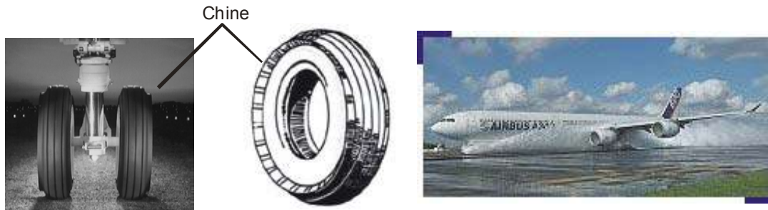
Diagram 8.37 Chined Tyre and Spray from a Nose Wheel
