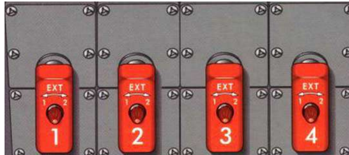
Diagram 14.22 Fire Handles Illuminate to Warn of Engine Fires
