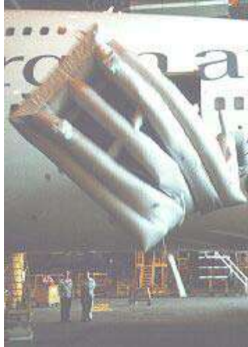
Diagram 15.23 Slide Raft Inflating
