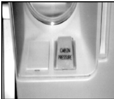
Diagram 13.25 Residual Pressure Indicators
