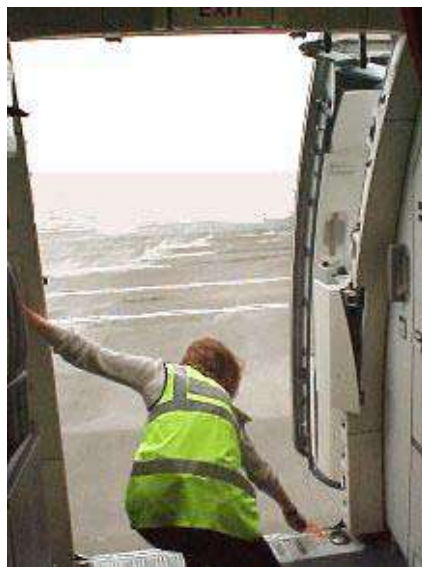
Diagram 15.22 Manual Inflation of Slide Raft after Automatic System Failed
