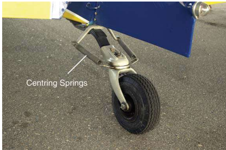
Diagram 7.15 Load-Operated Tail Wheel
