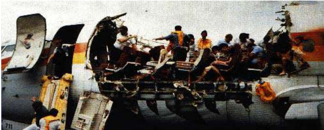
Diagram 1.6 Aloha B737 after a section of the cabin blew out when cracks in the aircraft's skin exceeded the material's CCL.
