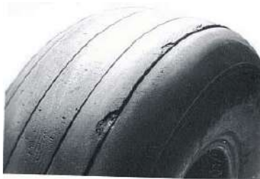
Diagram 8.45 Tread Chunking Cuts
