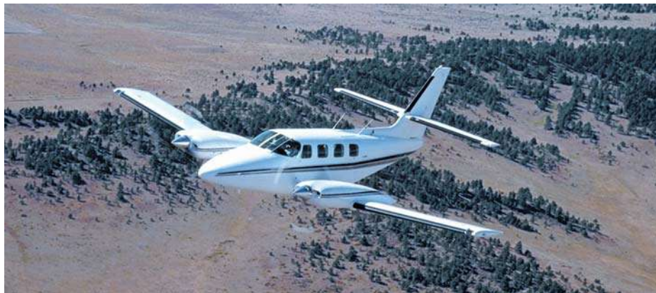
Diagram 4.15a Mid-Fin Mounted Tailplane
