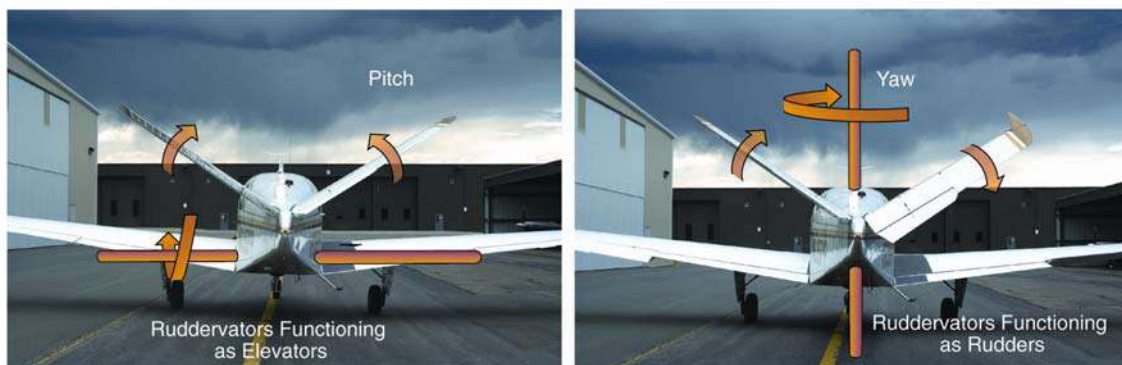
Diagram 5.45 V Tails Function
